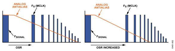
Figure 2. Increasing Oversampling Ratio (OSR) Reduces Noise
