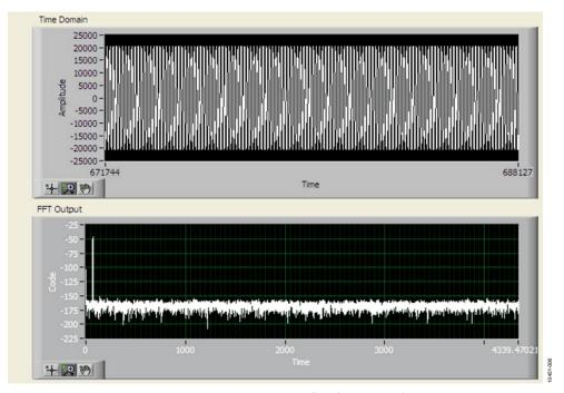
Figure 6. Response to 70 Hz Small-Scale Input Signal
