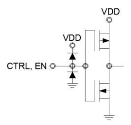
FIGURE 7. CTRL, EN Interface schematic circuits
