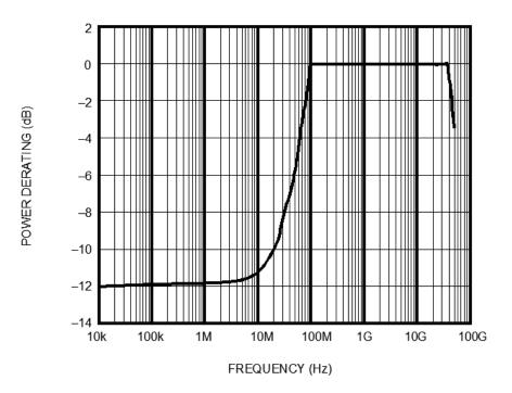
FIGURE 5. Power rating versus high frequency graph.
