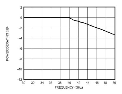
FIGURE 4. Power rating versus low frequency graph.
