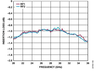
Figure 6. Insertion Loss vs. Frequency
