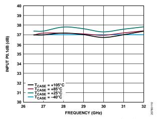
Figure 10. Input P0.1dB vs. Frequency, RF1 Selected
