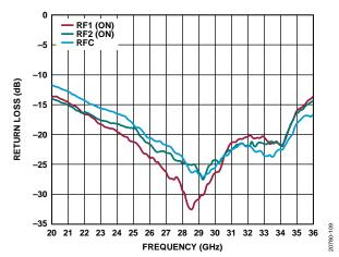
Figure 9. Return Loss vs. Frequency
