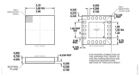
Figure 19. 20-Terminal Land Grid Array [LGA] 3 mm × 3 mm Body and 0.75 mm Package Height (CC-20-9) Dimensions shown in millimeters
