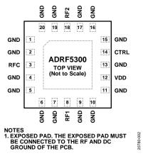
Figure 2. Pin Configuration (Top View)
