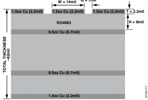
Figure 17. Probe Matrix Board Stack Up
