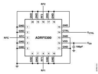
Figure 16. ADRF5300-EVALZ Simplified Application Circuit
