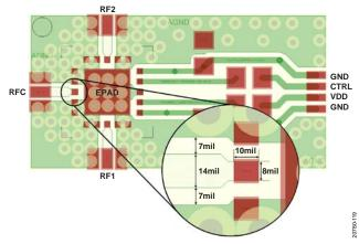
Figure 18. Probe Matrix Board, Top Layer
