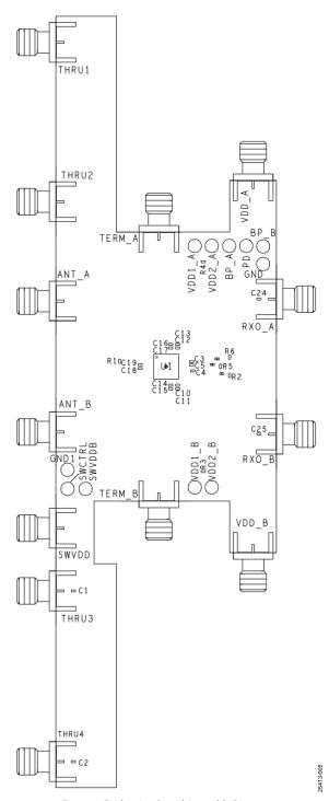
Figure 5. Evaluation Board Assembly Diagram
