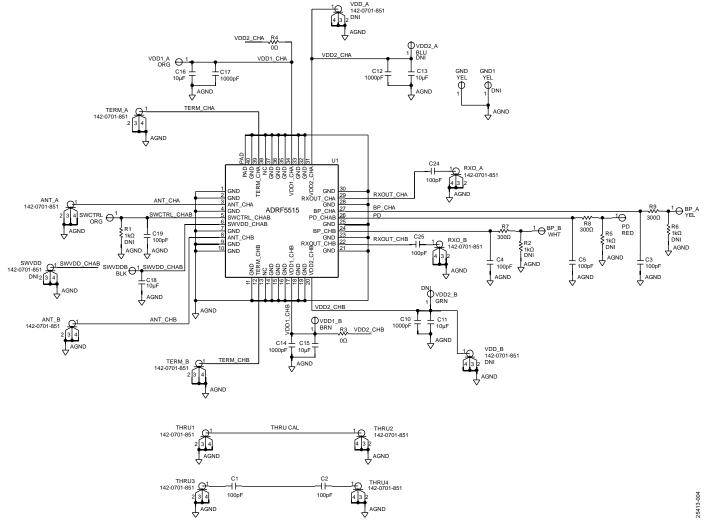
Figure 4. Evaluation Board Schematic
