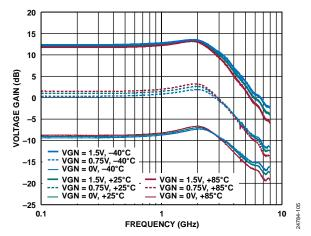
Figure 5. Voltage Gain vs. Frequency over Temperature and VGN, 43  $\Omega$  Back Terminations not De-Embedded
