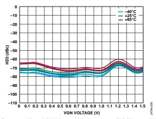
Figure 100. HD3 vs. VGN Voltage over Temperature and VOCM at 500 MHz
