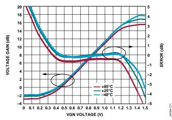
Figure 64. Voltage Gain and Error vs. VGN Voltage over Temperature at 3 GHz
