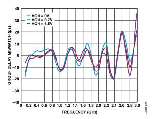
Figure 113. Group Delay Mismatch (Channel to Channel) vs. Frequency over
