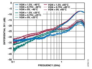
Figure 9. Differential Input Return Loss (S11) vs. Frequency over Temperature and VGN
