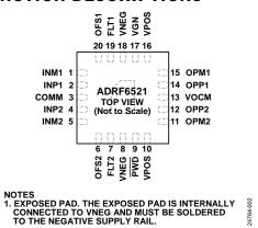
Figure 2. Pin Configuration
