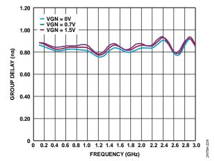
Figure 112. Group Delay vs. Frequency over VGN
