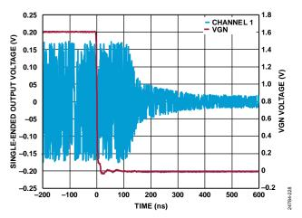
Figure 118. VGA Step Response Time, Maximum to Minimum Gain
