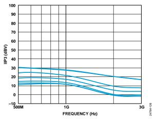
Figure 25. IIP3 vs. Frequency over VGN
