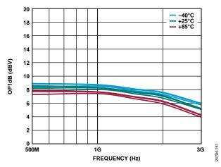
Figure 47. OP1dB vs. Frequency over Temperature and OFSx
