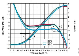
Figure 63. Voltage Gain and Error vs. VGN Voltage over Temperature at 1 GHz
