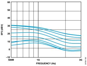
Figure 82. IIP3 vs. Frequency over VGN in 200 mV Steps
