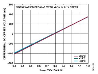
Figure 51. Differential DC Offset Voltage vs. V<sub>OFSx</sub> Voltage over Temperature and VOCM
