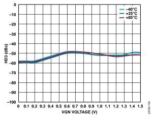
Figure 49. HD3 vs. VGN Voltage over Temperature and VOCM at 3 GHz
