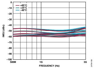
Figure 78. IMD2 vs. Frequency over Temperature and VGN
