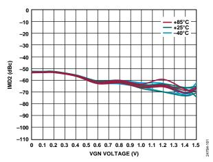
Figure 80. IMD2 vs. VGN Voltage over Temperature and OFSx at 500 MHz
