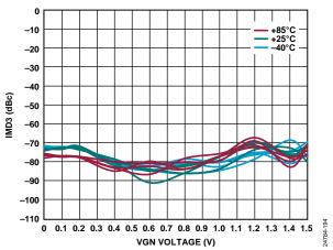
Figure 83. IMD3 vs. VGN Voltage over Temperature and OFSx at 500 MHz
