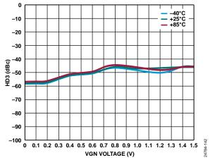
Figure 38. HD3 vs. VGN Voltage over Temperature and OFSx at 2 GHz
