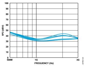
Figure 22. IIP2 vs. Frequency over VGN
