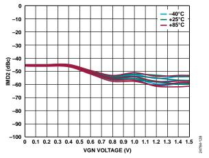
Figure 27. IMD2 vs. VGN Voltage over Temperature and OFSx at 1 GHz
