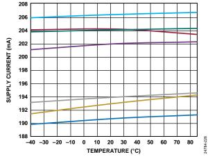
Figure 117. Supply Current vs. Temperature over Multiple Devices
