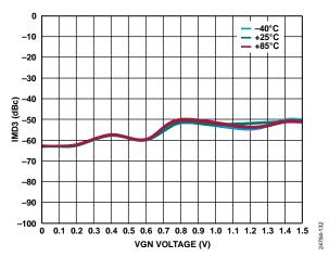
Figure 31. IMD3 vs. VGN Voltage over Temperature and OFSx at 2 GHz
