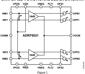
for second and third harmonic distortion (HD2 and HD3) from low frequency to 1 GHz. Variable output dc offset control is accomplished with the OFS1 and OFS2 pins, and the output common-mode can be controlled with the VOCM pin.
