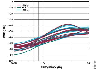
Figure 81. IMD3 vs. Frequency over Temperature and VGN
