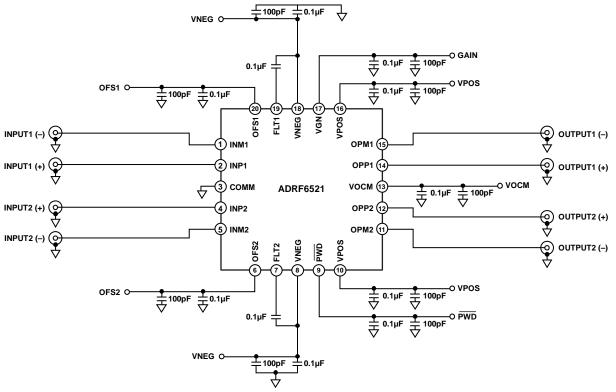
Figure 125. Basic Connections
