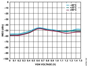
Figure 32. IMD3 vs. VGN Voltage over Temperature and OFSx at 3 GHz
