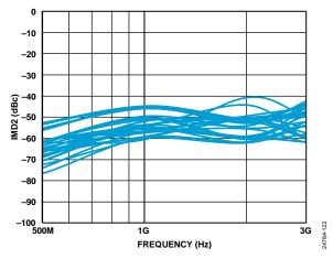
Figure 21. IMD2 vs. Frequency over VGN and OFSx
