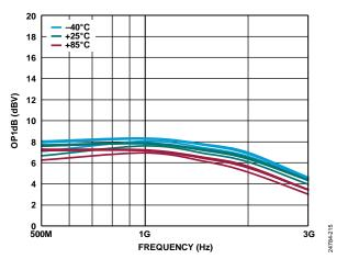
Figure 104. OP1dB vs. Frequency over Temperature and OFSx at Maximum
