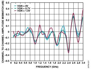
Figure 109. Channel to Channel Amplitude Mismatch vs. Frequency over VGN
