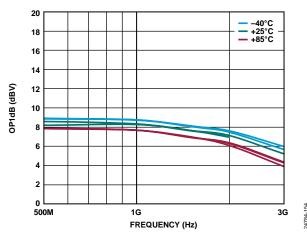
Figure 50. OP1dB vs. Frequency over Temperature and VOCM
