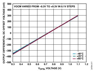
Figure 108. Output Differential DC Offset Voltage vs. V<sub>OFSx</sub> Voltage over Temperature and VOCM
