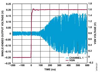
Figure 115. VGA Step Response Time, Minimum to Maximum Gain
