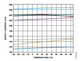
Figure 53. Supply Current vs. Temperature for Multiple Devices
