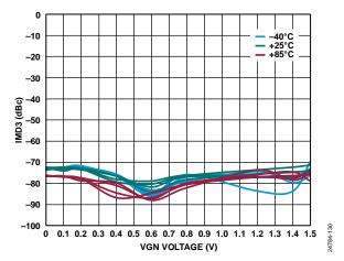
Figure 26. IMD3 vs. VGN Voltage over Temperature and OFSx at 500 MHz
