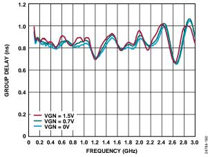
Figure 55. Group Delay vs. Frequency over VGN
