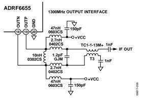
Figure 56. 1300 MHz Output Matching Network (Output return loss measured to be better than 12 dB from 1075 MHz to 1525 MHz.)
