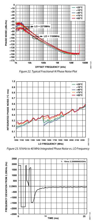
Figure 24. Lock Time for 10 MHz Step with 1.5 kHz Loop Filter
