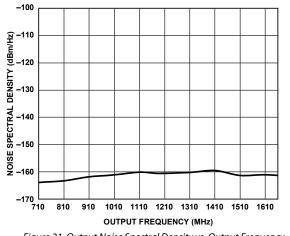
Figure 21. Output Noise Spectral Density vs. Output Frequency
