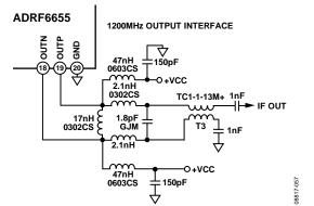
Figure 55. 1200 MHz Output Matching Network (Output return loss measured to be better than 12 dB from 950 MHz to 1500 MHz.)
