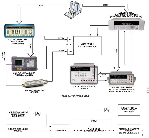
Figure 81. Noise Figure with Presence of Blocker Signal
