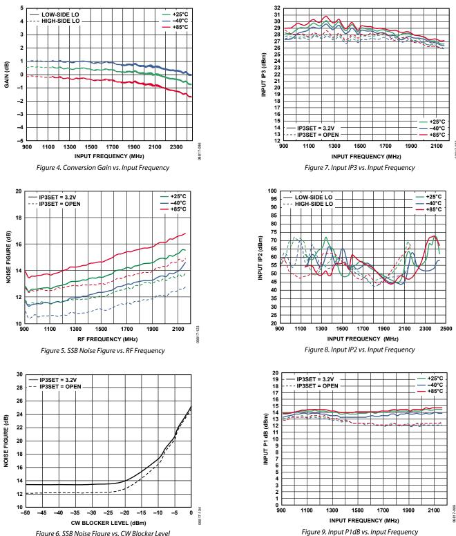
Figure 6. SSB Noise Figure vs. CW Blocker Level
