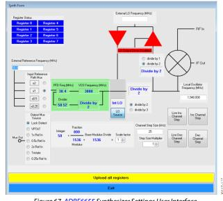
Figure 67. ADRF6655 Synthesizer Settings User Interface
