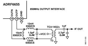
Figure 53. 850 MHz Output Matching Network Using the Center-Tap of the TC4-14T+ Transformer for Biasing the Open Collector Outputs (Output return loss measured to be better than 12 dB from 800 MHz to 925 MHz.)
