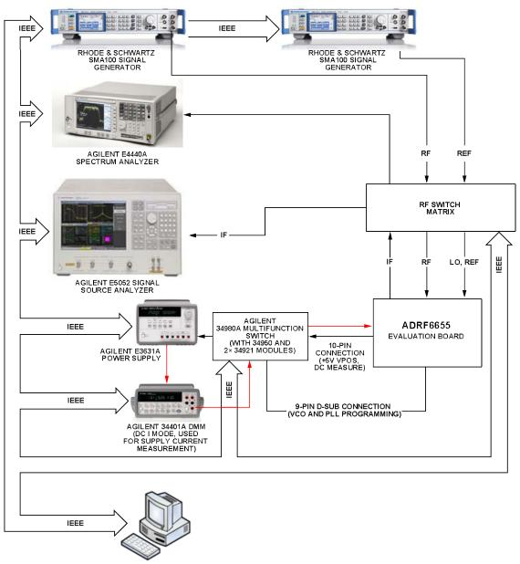
Figure 79. Phase Noise Setup
