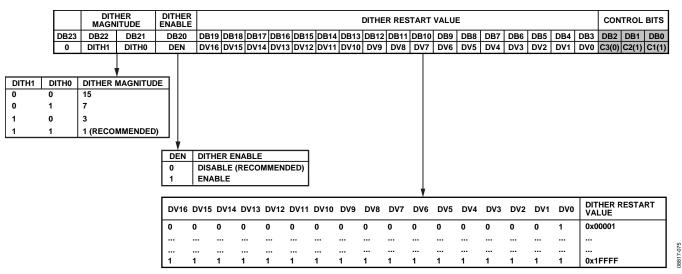
Figure 73.  $\Sigma$ - $\Delta$  Modulator Dither Control Register (R3)
