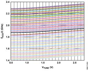
Figure 50. fvco/2 vs. Tuning Voltage for All 64 Bands
