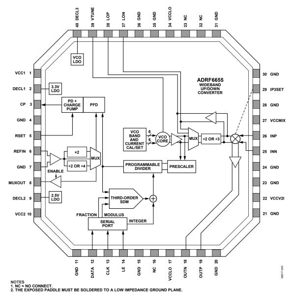
Figure 3. Pin Configuration
