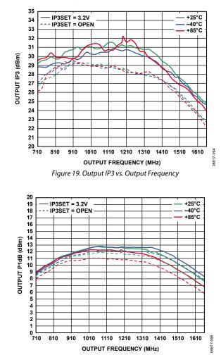
Figure 20. Output P1dB vs. Output Frequency
