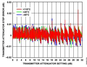
Figure 36. Transmitter Attenuator Step Error vs. Transmitter Attenuator Setting, LO = 525 MHz, Baseband Frequency = 10 MHz, Backoff = 15 dBFS
