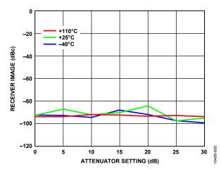
Figure 102. Receiver Image vs. Attenuator Setting, RF Bandwidth = 25 MHz, Tracking Calibration Active, Sample Rate = 61.44 MSPS, LO = 75 MHz, Baseband Frequency = 25 MHz
