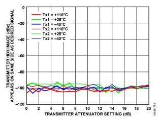
Figure 258. Transmitter HD3 Image Appears on Same Side as Desired Signal vs. Transmitter Attenuator Setting, LO = 3600 MHz, CW = -15 dBFS
