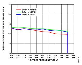
Figure 57. Observation Receiver IIP3, 2f1 – f2 vs. f1 Offset Frequency, LO = 300 MHz, Attenuation = 0 dB, Tones Separated by 1 MHz Swept Across Pass Band at –25 dBm Each
