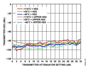
Figure 254. Transmitter HD2 vs. Transmitter Attenuator Setting, Baseband Frequency = 10 MHz, LO = 3600 MHz, CW = -15 dBFS
