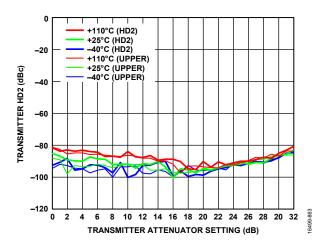
Figure 361. Transmitter HD2 vs. Transmitter Attenuator Setting, Baseband Frequency = 10 MHz, LO = 5900 MHz, CW = -15 dBFS
