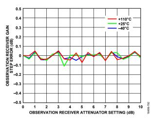
Figure 289. Observation Receiver Gain Step Error vs. Observation Receiver Attenuator Setting, LO = 3600 MHz
