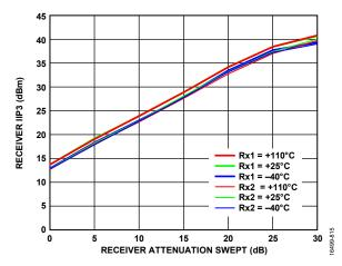
Figure 313. Receiver IIP3 vs. Receiver Attenuation Swept, LO = 4600 MHz, Tone 1 = 4695 MHz, Tone 2 = 4696 MHz, -21 dBm Plus Attenuation
