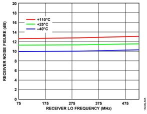
Figure 85. Receiver Noise Figure vs. Receiver LO Frequency, Receiver Attenuation = 0 dB, RF Bandwidth = 50 MHz, Sample Rate = 61.44 MSPS, Integration Bandwidth =  $\pm 25$  MHz
