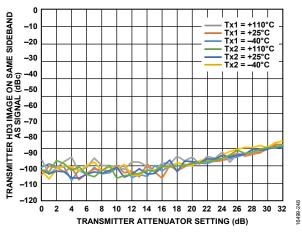
Figure 366. Transmitter HD3 Image on Same Sideband as Signal vs. Transmitter Attenuator Setting, LO = 5500 MHz, CW = -15 dBFS
