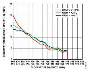
Figure 168. Observation Receiver IIP3, 2f1 – f2 vs. f1 Offset Frequency, LO = 650 MHz, Attenuation = 0 dB, Tones Separated by 1 MHz Swept Across Pass Band at –19 dBm Each
