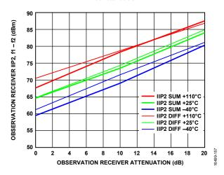
Figure 54. Observation Receiver IIP2, f1 - f2 vs. Observation Receiver Attenuation, LO = 300 MHz, Tone 1 = 302 MHz, Tone 2 = 322 MHz at -25 dBm Plus Attenuation
