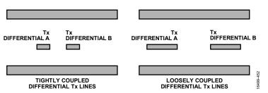
Figure 444. Routing JESD204B, Differential A and Differential B Correspond to Differential Positive Signals or Negative Signals (One Differential Pair)
