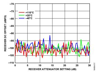
Figure 114. Receiver DC Offset vs. Receiver Attenuator Setting, LO = 525 MHz
