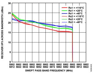
Figure 409. Receiver IIP3 Across Bandwidth vs. Swept Pass Band Frequency, Receiver Attenuation = 0 dB, LO = 5800 MHz, Tone 1 = 5802 MHz, Tone 2 Swept Across Pass Band, -21 dBm Each
