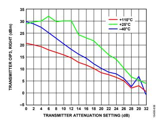
Figure 354. Transmitter OIP3, Right vs. Transmitter Attenuator Setting, LO = 5500 MHz, Total RMS Power = -12 dBFS
