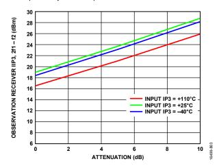
Figure 384. Observation Receiver IIP3, 2f1 – f2 vs. Attenuation, LO = 5700 MHz, Tone 1 = 5745 MHz, Tone 2 = 5746 MHz at –19 dBm Plus Attenuation
