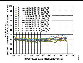
Figure 209. Receiver IIP2 Sum and Difference Across Bandwidth vs. Swept Pass Band Frequency, Receiver Attenuation = 0 dB, LO = 1800 MHz, Tone 1 = 1802 MHz, Tone 2 = Swept, -21 dBm Each
