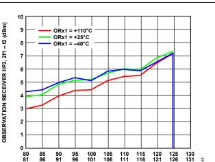
Figure 56. Observation Receiver IIP3, 2f1 (Where 2f1 is 2 × f1) – f2 vs. Intermodulation Frequency, LO = 75 MHz, Attenuation = 0 dB, Tones Separated by 1 MHz Swept Across Pass Band at –25 dBm Each
