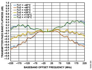
Figure 244. Transmitter Pass Band Flatness vs. Baseband Offset Frequency, Off Chip Match Response De-Embedded, LO = 3600 MHz
