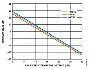
Figure 105. Receiver Gain vs. Receiver Attenuator Setting, RF Bandwidth = 50 MHz, Sample Rate = 61.44 MSPS, LO = 325 MHz
