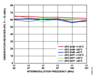
Figure 50. Observation Receiver IIP2, f1 – f2 (Where f2 is Frequency 2) vs. Intermodulation Frequency, LO = 75 MHz, Tone 1 = 77 MHz, Tone 2 = Swept, –25 dBm Each, Attenuation = 0 dB
