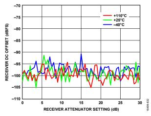
Figure 330. Receiver DC Offset vs. Receiver Attenuator Setting, LO = 3600 MHz
