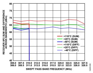
Figure 92. Receiver IIP2 Sum and Difference Across Bandwidth vs. Swept Pass Band Frequency, Receiver Attenuation = 0 dB, LO = 300 MHz, 10 Tone Pairs, -23.5 dBm Each
