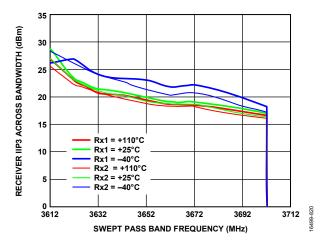
Figure 318. Receiver IIP3 Across Bandwidth vs. Swept Pass Band Frequency, Receiver Attenuation = 0 dB, LO = 3600 MHz, Tone 1 = 3602 MHz, Tone 2 = Swept Across Pass Band, -21 dBm Each
