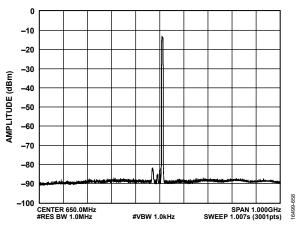
Figure 155. Amplitude vs. Frequency, Transmitter Output Spurious, Transmitter 1 = 2850 MHz, LTE = 5 MHz, Offset = 10 MHz, RMS = -12 dBFS, Temperature =  $25^{\circ}$ C
