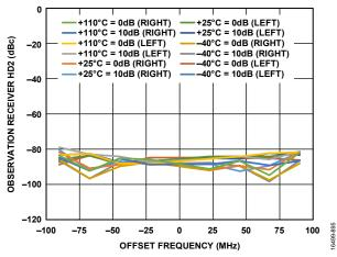
Figure 396. Observation Receiver HD2 vs. Offset Frequency, LO = 5700 MHz, Tone Level = -20 dBm Plus Attenuation
