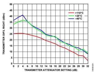
Figure 21. Transmitter OIP3 Right vs. Transmitter Attenuator Setting, LO = 525 MHz, Total RMS Power = -12 dBFS, 20 MHz/25 MHz Tones
