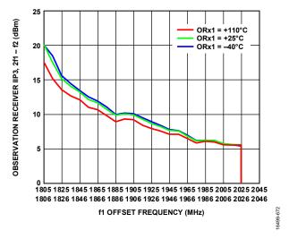
Figure 169. Observation Receiver IIP3, 2f1 – f2 vs. f1 Offset Frequency, LO = 1800 MHz, Attenuation = 0 dB, Tones Separated by 1 MHz Swept Across Pass Band at –19 dBm Each
