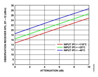
Figure 386. Observation Receiver IIP3, 2f1 - f2 vs. Attenuation, LO = 5700 MHz, Tone 1 = 5702 MHz, Tone 2 = 5822 MHz at -19 dBm Plus Attenuation
