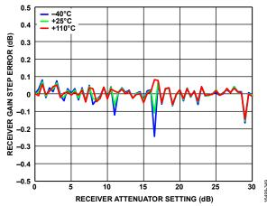
Figure 225. Receiver Gain Step Error vs. Receiver Attenuator Setting over Temperature
