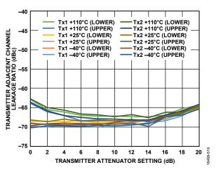
Figure 16. Transmitter Adjacent Channel Leakage Ratio vs. Transmitter Attenuator Setting, Signal Offset = 0 MHz, LO = 75 MHz, LTE = 20 MHz, Peak to Average Ratio (PAR) = 12 dB, DAC Boost Normal, Upper Side and Lower Side, Performance Limited by Spectrum Analyzer at Higher Attenuation Settings
