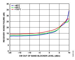
Figure 202. Receiver Noise Figure vs. CW Out of Band Blocker Level, Receiver LO = 1685 MHz, Blocker = 2085 MHz
