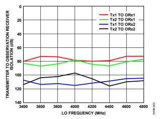
Figure 299. Transmitter to Observation Receiver Isolation vs. LO Frequency, Temperature =  $25^{\circ}$ C
