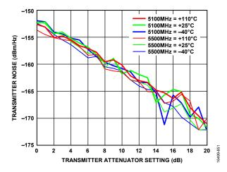
Figure 349. Transmitter Noise vs. Transmitter Attenuator Setting
