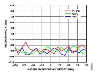
Figure 410. Receiver Image vs. Baseband Frequency Offset, Attenuation = 0 dB, RF Bandwidth = 200 MHz, Tracking Calibration Active, Sample Rate = 245.76 MSPS, LO = 5200 MHz
