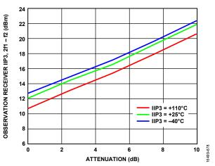
Figure 175. Observation Receiver IIP3, 2f1 – f2 vs. Attenuation, LO = 1800 MHz, Tone 1 = 1802 MHz, Tone 2 = 1922 MHz at –19 dBm Plus Attenuation
