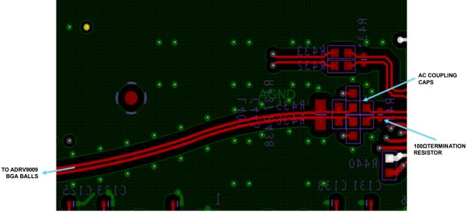
Figure 435. REF\_CLK\_IN± Routing Recommendation
