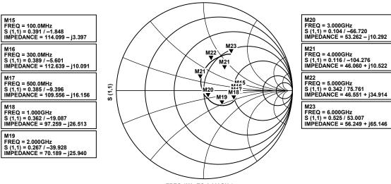
**FREQ (0Hz TO 6.000GHz)** Figure 428. Observation Receiver Input Impedance SEDZ
