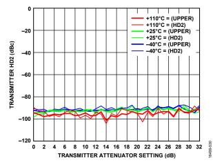
Figure 27. Transmitter HD2 vs. Transmitter Attenuator Setting, Baseband Frequency = 10 MHz, LO = 525 MHz, CW = -15 dBFS
