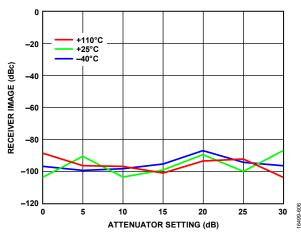
Figure 103. Receiver Image vs. Attenuator Setting, RF Bandwidth = 25 MHz, Tracking Calibration Active, Sample Rate = 61.44 MSPS, LO = 325 MHz, Baseband Frequency = 25 MHz
