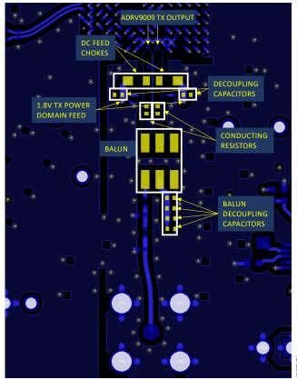
Figure 443. Transmitter DC Chokes and Balun Feed Supply
