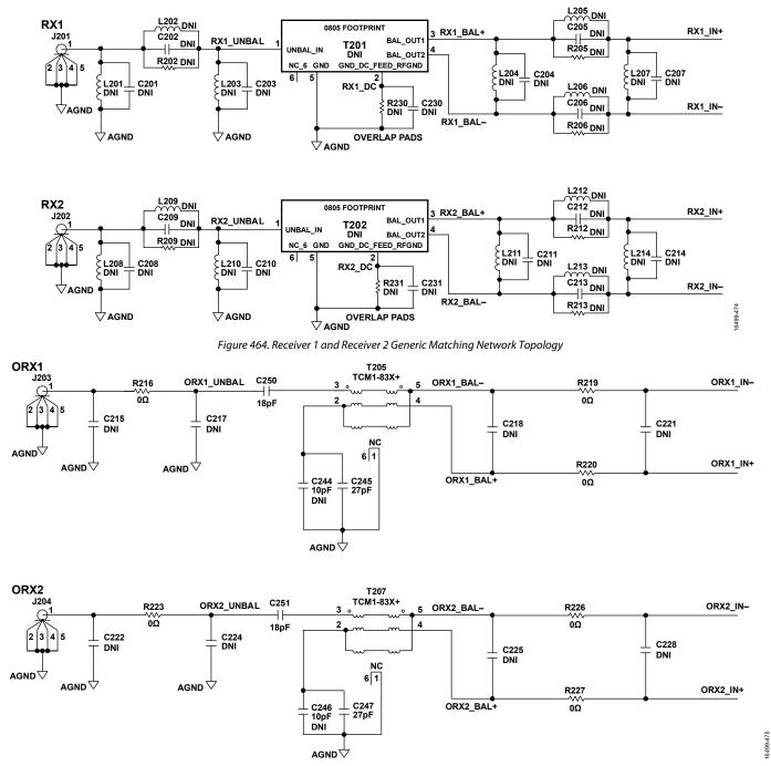
Figure 465. Observation Receiver 1 and Observation Receiver 2 Generic Matching Network Topology
