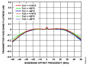
Figure 11. Transmitter Pass Band Flatness vs. Baseband Offset Frequency, Off Chip Match Response De-Embedded, LO = 300 MHz, Calibrated at  $25^{\circ}$ C
