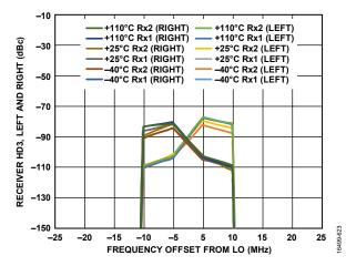
Figure 120. Receiver HD3, Left and Right vs. Frequency Offset from LO, Tone Level = -17 dBm at Attenuation = 0 dB, LO = 525 MHz
