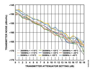
Figure 135. Transmitter Noise vs. Transmitter Attenuator Setting,
