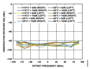
Figure 395. Observation Receiver HD2 vs. Offset Frequency, LO = 5200 MHz, Tone Level = -20 dBm Plus Attenuation
