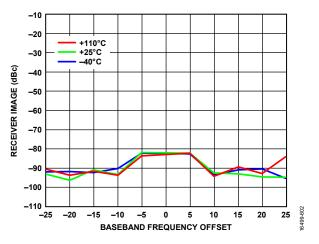
Figure 99. Receiver Image vs. Baseband Frequency Offset, Attenuation = 0 dB, RF Bandwidth = 50 MHz, Tracking Calibration Active, Sample Rate = 61.44 MSPS, LO = 75 MHz
