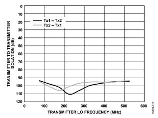
Figure 14. Transmitter to Transmitter Isolation vs. Transmitter LO Frequency, Temperature =  $25^{\circ}$ C
