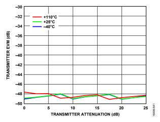
Figure 38. Transmitter EVM vs. Transmitter Attenuation, LTE = 20 MHz, Signal Centered on DC, LO = 300 MHz
