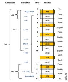
Figure 432. ADRV9009-W/PCBZ Trace Impedance and Stackup
