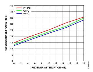
Figure 197. Receiver Noise Figure vs. Receiver Attenuation, LO = 2850 MHz, Receiver Bandwidth = 200 MHz Bandwidth, Sample Rate = 245.76 MSPS, Integration Bandwidth = 500 kHz to 100 MHz
