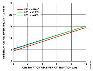
Figure 58. Observation Receiver IIP3, 2f1 - f2 vs. Observation Receiver Attenuation, LO = 75 MHz, Tone 1 = 100 MHz, Tone 2 = 101 MHz at -24 dBm Plus Attenuation
