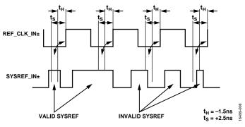
Figure 3. SYSREF\_IN± Setup and Hold Timing Examples, Relative to Device Clock
