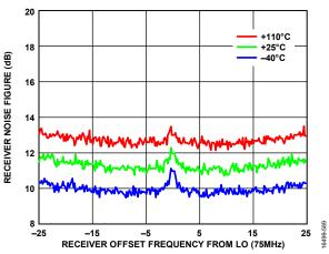
Figure 86. Receiver Noise Figure vs. Receiver Offset Frequency from LO, Integration Bandwidth = 200 kHz, LO = 75 MHz
