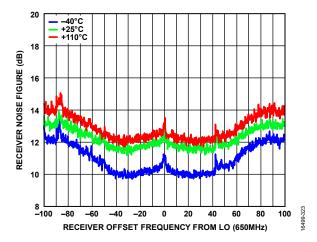
Figure 199. Receiver Noise Figure vs. Receiver Offset Frequency from LO, LO = 650 MHz
