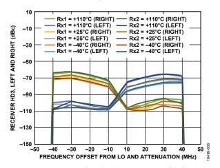
Figure 334. Receiver HD3, Left and Right vs. Frequency Offset from LO and Attenuation, Tone Level = -15 dBm at Attenuation = 0 dB, LO = 3600 MHz
