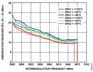
Figure 174. Observation Receiver IIP3, 2f1 - f2 vs. Intermodulation Frequency, LO = 2850 MHz, Tone 1 = 2852 MHz, Tone 2 = Swept at -19 dBm Each
