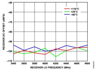
Figure 329. Receiver DC Offset vs. Receiver LO Frequency
