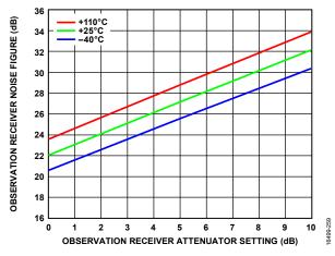
Figure 377. Observation Receiver Noise Figure vs. Observation Receiver Attenuator Setting, LO = 5500 MHz, Total Nyquist Integration Bandwidth
