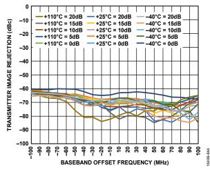
Figure 342. Transmitter Image Rejection vs. Baseband Offset Frequency, QEC Trained with Three Tones Placed at 10 MHz, 50 MHz, and 100 MHz (Tracking On), Total Combined Power = –6 dBFS, Correction then Frozen (Tracking Turned Off), CW Tone Swept Across Large Signal Bandwidth, LO = 5100 MHz
