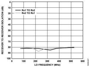
Figure 124. Receiver to Receiver Isolation vs. LO Frequency, Baseband Frequency = 10 MHz
