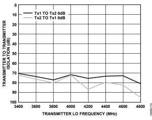
Figure 248. Transmitter to Transmitter Isolation vs. Transmitter LO Frequency, Temperature = 25℃
