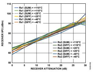
Figure 93. Receiver IIP2 vs. Receiver Attenuation, LO = 75 MHz, Tones Placed at 77 MHz and 97 MHz, -23.5 dBm Plus Attenuation
