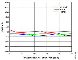
Figure 262. EVM vs. Transmitter Attenuation, LTE = 20 MHz Signal Centered on DC, LO = 3600 MHz
