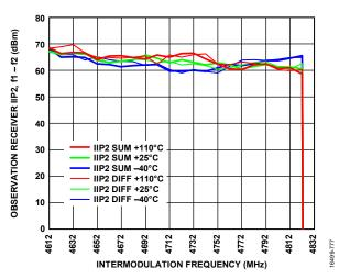
Figure 274. Observation Receiver IIP2, f1 – f2 vs. Intermodulation Frequency, LO = 4600 MHz, Tone 1 = 4602 MHz, Tone 2 Swept, –22 dBm Each, Attenuation = 0 dB
