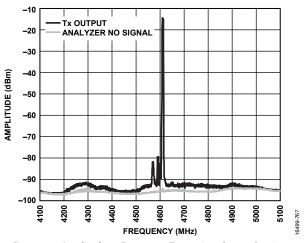
Figure 264. Amplitude vs. Frequency, Transmitter Output Spurious, Transmitter 1 = 4600 MHz, LTE = 5 MHz, Offset = 10 MHz, RMS Ripple in Noise Floor Due to Spectrum Analyzer = -12 dBFS, Temperature =  $25^{\circ}$ C
