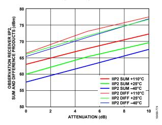
Figure 271. Observation Receiver IIP2, Sum and Difference Products vs. Attenuation, LO = 3600 MHz, Tone 1 = 3645 MHz, Tone 2 = 3646 MHz at -22 dBm Plus Attenuation
