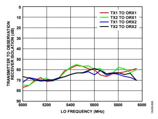
Figure 399. Transmitter to Observation Receiver Isolation vs. LO Frequency, Temperature =  $25^{\circ}$ C
