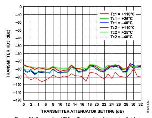
Figure 30. Transmitter HD3 vs. Transmitter Attenuator Setting, LO = 525 MHz, CW = -15 dBFS, Baseband Frequency = 10 MHz
