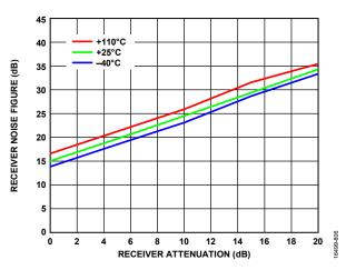
Figure 303. Receiver Noise Figure vs. Receiver Attenuation, LO = 4600 MHz, Bandwidth = 200 MHz, Sample Rate = 245.76 MSPS, Integration Bandwidth = 500 kHz to 100 MHz
