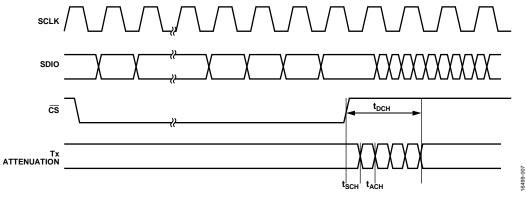
Figure 4. Transmitter Attenuation Update via SPI 2 Port
