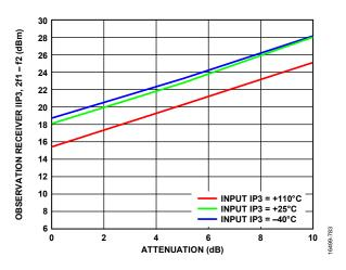
Figure 280. Observation Receiver IIP3, 2f1 – f2 vs. Attenuation, LO = 4600 MHz, Tone 1 = 4695 MHz, Tone 2 = 4696 MHz at –22 dBm Plus Attenuation
