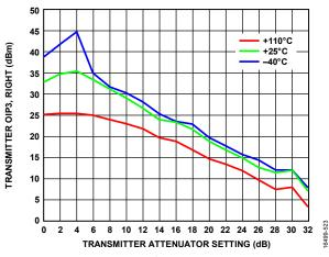
Figure 20. Transmitter OIP3 Right vs. Transmitter Attenuator Setting, LO = 300 MHz, Total RMS Power = -12 dBFS, 20 MHz/25 MHz Tones
