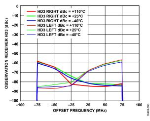
Figure 188. Observation Receiver HD3 vs. Offset Frequency, LO = 650 MHz, Tone Level = -20 dBm at 0 dB Attenuation
