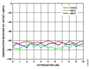
Figure 184. Observation Receiver DC Offset vs. Attenuation, LO = 1850 MHz
