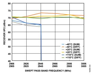
Figure 206. Receiver IIP2 Sum and Difference Across Bandwidth vs Swept Pass Band Frequency, LO = 2900 MHz
