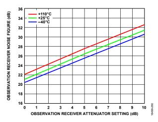
Figure 378. Observation Receiver Noise Figure vs. Observation Receiver Attenuator Setting, LO = 5800 MHz, Total Nyquist Integration Bandwidth
