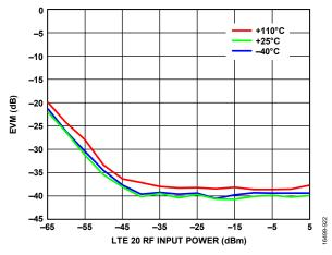
Figure 424. EVM vs. LTE20 RF Input Power, LO = 5800 MHz, Default AGC Settings
