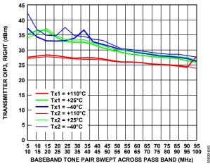
Figure 142. Transmitter OIP3, Right vs. Baseband Tone Pair Swept Across Pass Band, LO = 850 MHz, 15 dB Digital Backoff per Tone
