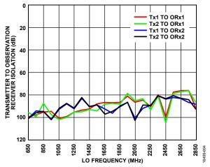
Figure 192. Transmitter to Observation Receiver Isolation vs. LO Frequency, Temperature =  $25^{\circ}$ C
