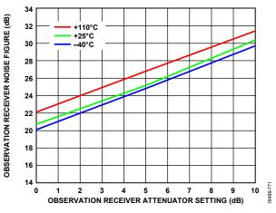
Figure 268. Observation Receiver Noise Figure vs. Observation Receiver Attenuator Setting, LO = 4600 MHz, Total Nyquist Integration Bandwidth
