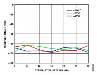
Figure 323. Receiver Image vs. Attenuator Setting, RF Bandwidth = 200 MHz, Tracking Calibration Active, Sample Rate = 245.76 MSPS, LO = 4600 MHz, Baseband Frequency = 10 MHz
