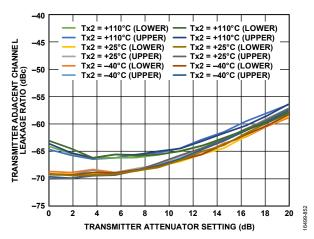
Figure 350. Transmitter Adjacent Channel Leakage Ratio vs. Transmitter Attenuator Setting, LO = 5100 MHz, LTE = 20 MHz, PAR = 12 dB, DAC Boost Normal, Upper Side and Lower Side, Decreasing ACLR at Higher Attenuation Due to Spectrum Analyzer Noise Floor
