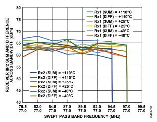
Figure 94. Receiver IIP2 Sum and Difference Across Bandwidth vs. Swept Pass Band Frequency, Receiver Attenuation = 0 dB, LO = 75 MHz, Tone 1 = 77 MHz, Tone 2 Swept, -23.5 dBm Each
