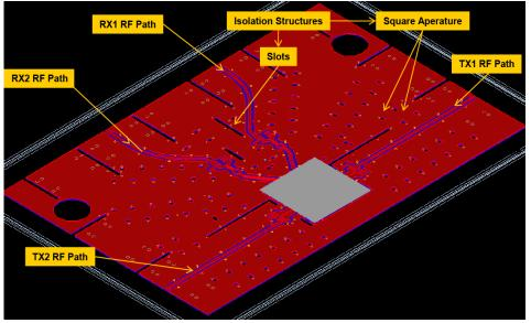
Figure 445. Isolation Structures on the ADRV9009-W/PCBZ
