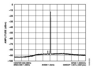
Figure 151. Amplitude vs. Frequency, Transmitter Output Spurious, Transmitter 1 = 650 MHz, LTE = 5 MHz, Offset = 10 MHz, RMS = -12 dBFS, Temperature =  $25^{\circ}C$
