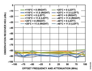
Figure 185. Observation Receiver HD2 vs. Offset Frequency and Attenuation, LO = 650 MHz, Tone Level = -20 dBm at 0 dB Attenuation
