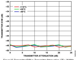
Figure 37. Transmitter EVM vs. Transmitter Attenuation, LTE = 20 MHz, Signal Centered on DC, LO = 75 MHz
