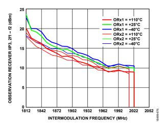
Figure 173. Observation Receiver IIP3, 2f1 - f2 vs. Intermodulation Frequency, LO = 1800 MHz, Tone 1 = 1802 MHz, Tone 2 = Swept at -19 dBm Each
