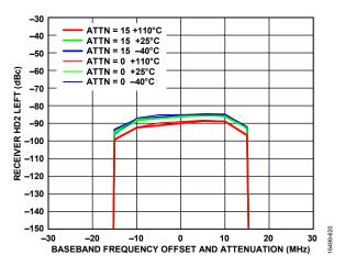
Figure 117. Receiver HD2 Left vs. Baseband Frequency Offset and Attenuation, Tone Level = -21 dBm at Attenuation = 0 dB, X-Axis is Baseband Frequency Offset of Fundamental Tone, Not Frequency of HD2 Product (HD2 Product Is 2 × Baseband Frequency), HD2 Canceller Disabled, LO = 525 MHz
