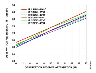
Figure 53. Observation Receiver IIP2, f1 - f2 vs. Observation Receiver Attenuation, LO = 75 MHz, Tone 1 = 77 MHz, Tone 2 = 97 MHz at -25 dBm Plus Attenuation
