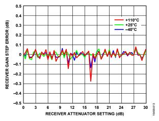
Figure 110. Receiver Gain Step Error vs. Receiver Attenuator Setting, LO = 525 MHz
