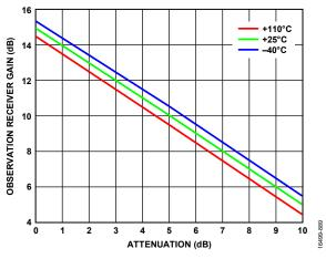
Figure 390. Observation Receiver Gain vs. Attenuation, LO = 5700 MHz
