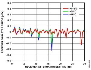
Figure 416. Receiver Gain Step Error vs. Receiver Attenuator Setting, LO = 6000 MHz
