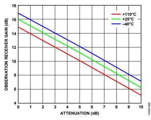
Figure 389. Observation Receiver Gain vs. Attenuation, LO = 5200 MHz
