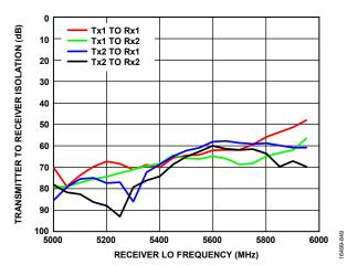
Figure 347. Transmitter to Receiver Isolation vs. Receiver LO Frequency, Temperature =  $25^{\circ}$ C
