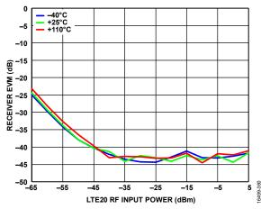
Figure 235. Receiver EVM vs. LTE20 RF Input Power, LTE = 20 MHz RF Signal, LO = 600 MHz
