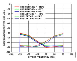
Figure 189. Observation Receiver HD3 vs. Offset Frequency, LO = 1850 MHz, Tone Level = -20 dBm at 0 dB Attenuation
