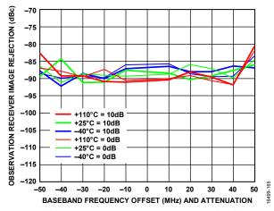
Figure 62. Observation Receiver Image Rejection vs. Baseband Frequency Offset and Attenuation, CW Signal Swept Across the Pass Band, LO = 75 MHz
