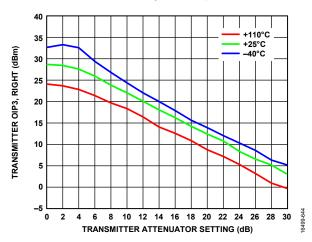
Figure 141. Transmitter OIP3, Right vs. Transmitter Attenuator Setting, LO = 2650 MHz, 15 dB Digital Backoff per Tone
