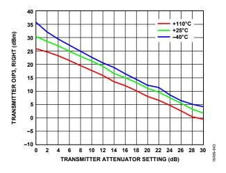
Figure 140. Transmitter OIP3, Right vs. Transmitter Attenuator Setting, LO = 1850 MHz, 15 dB Digital Backoff per Tone
