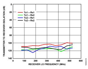
Figure 13. Transmitter to Receiver Isolation vs. Receiver LO Frequency, Temperature =  $25^{\circ}$ C
