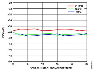
Figure 371. EVM vs. Transmitter Attenuation, LTE Signal = 20 MHz Centered on DC, LO = 5100 MHz
