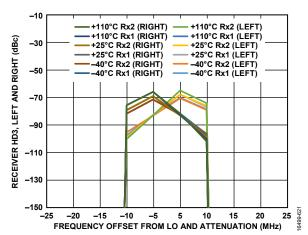
Figure 118. Receiver HD3, Left and Right vs. Frequency Offset from LO and Attenuation, Tone Level = -16 dBm at Attenuation = 0 dB, LO = 75 MHz
