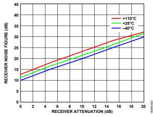
Figure 83. Receiver Noise Figure vs. Receiver Attenuation, LO = 300 MHz, RF Bandwidth = 50 MHz, Sample Rate = 61.44 MSPS, Integration Bandwidth = 1 MHz to 25 MHz
