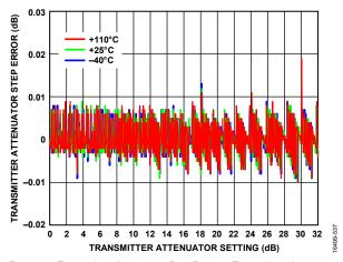
Figure 34. Transmitter Attenuator Step Error vs. Transmitter Attenuator Setting, LO = 75 MHz, Baseband Frequency = 10 MHz, Backoff = 15 dBFS
