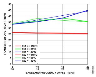
Figure 23. Transmitter OIP3 Right vs. Baseband Frequency Offset, LO = 300 MHz, Total RMS Power = -12 dBFS, Transmitter Attenuation = 4 dB
