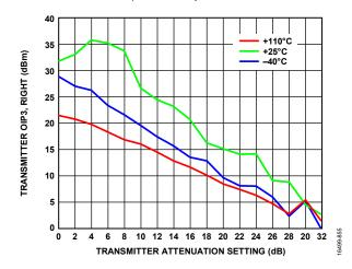
Figure 353. Transmitter OIP3, Right vs. Transmitter Attenuator Setting, LO = 5100 MHz, Total RMS Power = -12 dBFS
