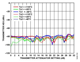
Figure 257. Transmitter HD3 vs. Transmitter Attenuator Setting, LO = 4600 MHz, CW = -15 dBFS, Baseband Frequency = 10 MHz
