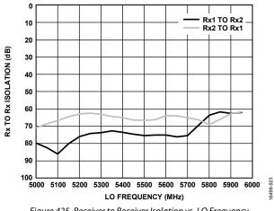
Figure 425. Receiver to Receiver Isolation vs. LO Frequency
