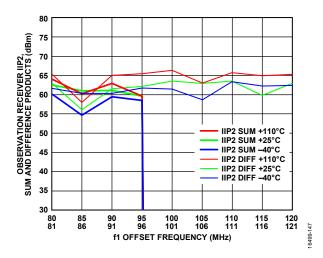
Figure 44. Observation Receiver IIP2, Sum and Difference Products vs. f1 (Where f1 is Frequency 1) Offset Frequency, Tones Separated by 1 MHz Swept Across Pass Band at –25 dBm Each, LO = 75 MHz, Attenuation = 0 dB
