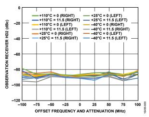
Figure 186. Observation Receiver HD2 vs. Offset Frequency and Attenuation, LO = 1850 MHz, Tone Level = -20 dBm at 0 dB Attenuation
