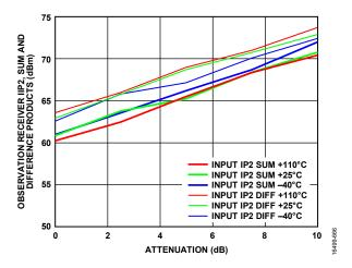
Figure 163. Observation Receiver IIP2, Sum and Difference Products vs. Attenuation, Tone 1 = 1845 MHz, Tone 2 = 1846 MHz at –19 dBm Plus Attenuation, LO = 1800 MHz
