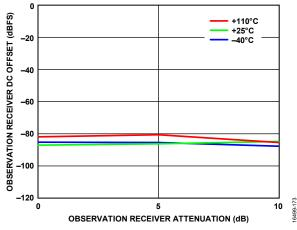
Figure 70. Observation Receiver DC Offset vs. Observation Receiver Attenuation, LO = 75 MHz, Baseband Frequency = 50 MHz
