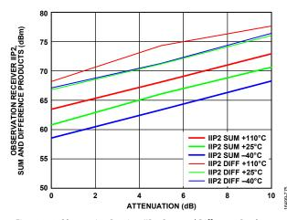
Figure 272. Observation Receiver IIP2, Sum and Difference Products vs. Attenuation, LO = 4600 MHz, Tone 1 = 4645 MHz, Tone 2 = 4646 MHz at -22 dBm Plus Attenuation
