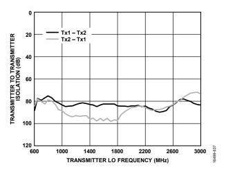
Figure 134. Transmitter to Transmitter Isolation vs. Transmitter LO Frequency, Temperature = 25℃
