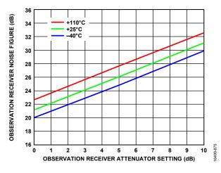
Figure 376. Observation Receiver Noise Figure vs. Observation Receiver Attenuator Setting, 5200 MHz, Total Nyquist Integration Bandwidth
