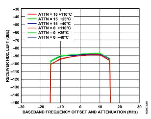
Figure 116. Receiver HD2 Left vs. Baseband Frequency Offset and Attenuation, Tone Level = -21 dBm at Attenuation = 0 dB, X-Axis is Baseband Frequency Offset of Fundamental Tone, Not Frequency of HD2 Product (HD2 Product Is 2 × Baseband Frequency), HD2 Canceller Disabled, LO = 300 MHz
