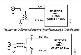
Figure 461. Differential Receiver Interface Using a Transmission Line Balun
