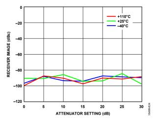
Figure 322. Receiver Image vs. Attenuator Setting, RF Bandwidth = 200 MHz, Tracking Calibration Active, Sample Rate = 245.76 MSPS, LO = 3600 MHz, Baseband Frequency = 10 MHz
