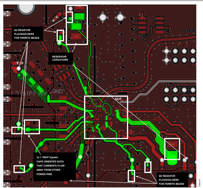
Figure 438. Placement Example of 0 Ω Resistor Placeholders for FBs, Reservoir Capacitors, and Bypass Capacitors on the ADRV9009-W/PCBZ (Layer 12 to Power Layer and Bottom Layer)
