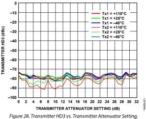
Figure 28. Transmitter HD3 vs. Transmitter Attenuator Setting, LO = 75 MHz, CW = -15 dBFS, Baseband Frequency = 10 MHz
