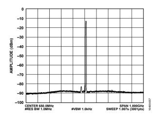
Figure 154. Amplitude vs. Frequency, Transmitter Output Spurious, Transmitter 2 = 1850 MHz, LTE = 5 MHz, Offset = 10 MHz, RMS = -12 dBFS, Temperature =  $25^{\circ}$ C
