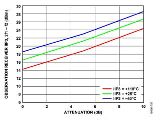
Figure 284. Observation Receiver IIP3, 2f1 - f2 vs. Attenuation, LO = 4600 MHz, Tone 1 = 4602 MHz, Tone 2 = 4722 MHz at -22 dBm Plus Attenuation Each
