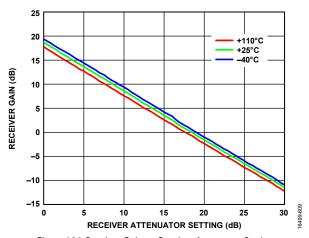
Figure 106. Receiver Gain vs. Receiver Attenuator Setting, RF Bandwidth = 50 MHz, Sample Rate = 61.44 MSPS, LO = 525 MHz
