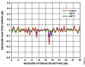
Figure 109. Receiver Gain Step Error vs. Receiver Attenuator Setting, LO = 325 MHz
