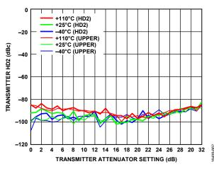
Figure 360. Transmitter HD2 vs. Transmitter Attenuator Setting, Baseband Frequency = 10 MHz, LO = 5500 MHz, CW = -15 dBFS
