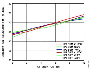
Figure 167. Observation Receiver IIP2, f1 – f2 vs. Attenuation, LO = 1800 MHz, Tone 1 = 1802 MHz, Tone 2 = 1902 MHz at –19 dBm Plus Attenuation
