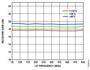
Figure 107. Receiver Gain vs. LO Frequency, RF Bandwidth = 50 MHz, Sample Rate = 61.44 MSPS
