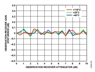
Figure 66. Observation Receiver Gain Step Error vs. Observation Receiver Attenuator, LO = 75 MHz
