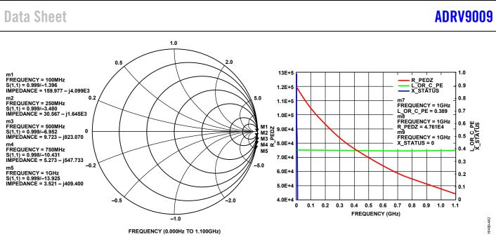
Figure 452. REF\_CLK\_IN± SEDZ and PEDZ Data, On Average, the Real Part of the Parallel Equivalent Differential Impedance ( $R_P$ ) = Approximately 70 k $\Omega$
