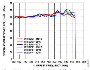
Figure 164. Observation Receiver IIP2, f1 - f2 vs. f1 Offset Frequency, LO = 650 MHz, Tone 1 = 652 MHz, Tone 2 = Swept at -19 dBm Each, Attenuation = 0 dB
