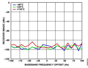
Figure 220. Receiver Image vs. Baseband Frequency Offset, Attenuation = 0 dB, RF Bandwidth = 200 MHz, Tracking Calibration Active, Sample Rate = 245.76 MSPS, LO = 1850 MHz
