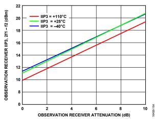
Figure 61. Observation Receiver IIP3, 2f1 - f2 vs. Observation Receiver Attenuation, LO = 300 MHz, Tone 1 = 302 MHz, Tone 2 = 352 MHz at -19 dBm Plus Attenuation
