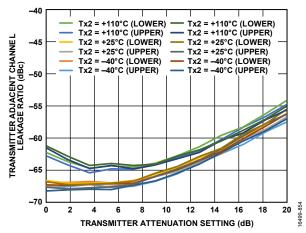
Figure 352. Transmitter Adjacent Channel Leakage Ratio vs. Transmitter Attenuator Setting, LO = 5900 MHz, LTE = 20 MHz, PAR = 12 dB, DAC Boost Normal, Upper Side and Lower Side, Decreasing ACLR at Higher Attenuation Due to Spectrum Analyzer Noise Floor
