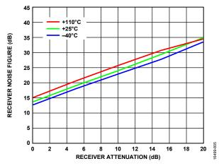
Figure 302. Receiver Noise Figure vs. Receiver Attenuation, LO = 3600 MHz, Receiver Bandwidth = 200 MHz, Sample Rate = 245.76 MSPS, Integration Bandwidth = 500 kHz to 100 MHz
