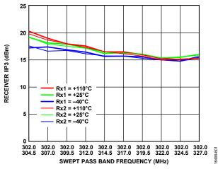
Figure 98. Receiver IIP3 vs. Swept Pass Band Frequency, Receiver Attenuation = 0 dB, LO = 300 MHz, Tone 1 = 302 MHz, Tone 2 = Swept Across Pass Band, -19 dBm Each
