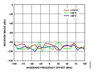
Figure 321. Receiver Image vs. Baseband Frequency Offset, Attenuation = 0 dB, RF Bandwidth = 200 MHz, Tracking Calibration Active, Sample Rate = 245.76 MSPS, LO = 4600 MHz
