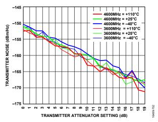
Figure 249. Transmitter Noise vs. Transmitter Attenuator Setting
