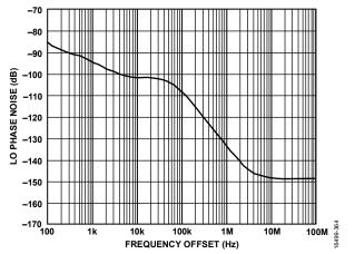
Figure 239. LO Phase Noise vs. Frequency Offset, LO = 1900 MHz, RMS Phase Error Integrated from 2 kHz to 18 MHz, Spectrum Analyzer Limits Far Out Noise
