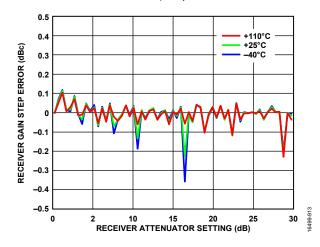
Figure 414. Receiver Gain Step Error vs. Receiver Attenuator Setting, LO = 5200 MHz
