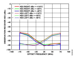
Figure 190. Observation Receiver HD3 vs. Offset Frequency, LO = 2850 MHz, Tone Level = -20 dBm at 0 dB Attenuation
