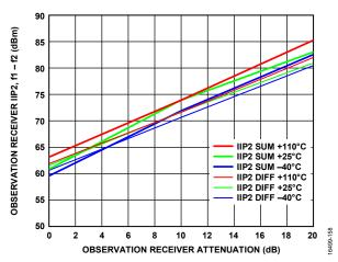
Figure 55. Observation Receiver IIP2, f1 – f2 vs. Observation Receiver Attenuation, LO = 525 MHz, Tone 1 = 527 MHz, Tone 2 = 547 MHz at –25 dBm Plus Attenuation
