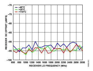
Figure 227. Receiver DC Offset vs. Receiver LO Frequency
