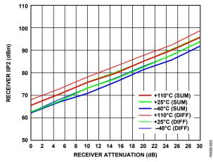
Figure 90. Receiver IIP2 vs. Receiver Attenuation, LO = 300 MHz, Tones Placed at 310 MHz and 311 MHz, -23.5 dBm Plus Attenuation
