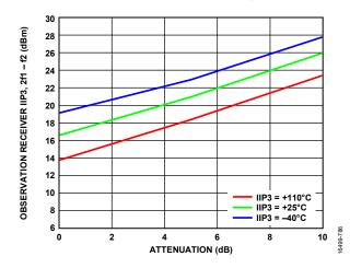
Figure 283. Observation Receiver IIP3, 2f1 – f2 vs. Attenuation, LO = 3600 MHz, Tone 1 = 3602 MHz, Tone 2 = 3722 MHz, -22 dBm Each Plus Attenuation
