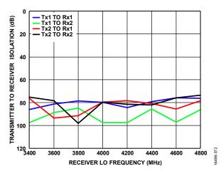
Figure 247. Transmitter to Receiver Isolation vs. Receiver LO Frequency, Temperature =  $-40^{\circ}$ C,  $+25^{\circ}$ C, and  $+110^{\circ}$ C
