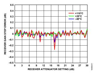
Figure 108. Receiver Gain Step Error vs. Receiver Attenuator Setting, LO = 75 MHz
