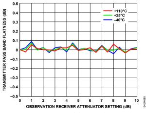
Figure 182. Transmitter Pass Band Flatness vs. Observation Receiver Attenuator Setting, LO = 2600 MHz
