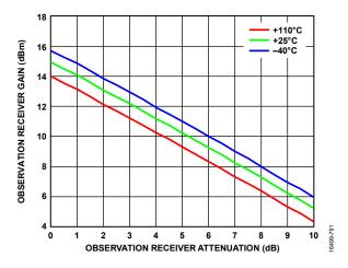
Figure 288. Observation Receiver Gain vs. Observation Receiver Attenuation, LO = 4600 MHz
