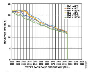
Figure 214. Receiver IIP3 vs. Swept Pass Band Frequency, Receiver Attenuation = 0 dB, LO = 2900 MHz, Tone 2 = Tone 1 + 1 MHz, -21 dBm Each, Swept Across Pass Band
