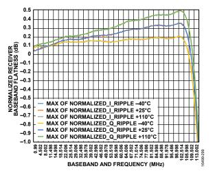
Figure 417. Normalized Receiver Baseband Flatness vs. Baseband and Frequency (Receiver Flatness)
