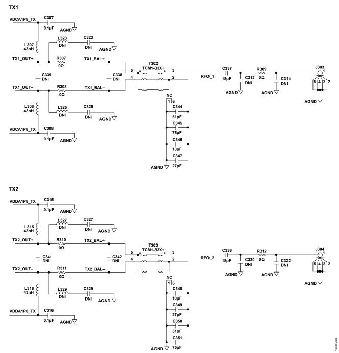
Figure 463. Transmitter 1 and Transmitter 2 Generic Matching Network Topology
