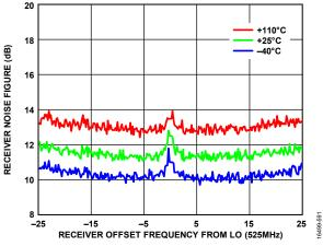
Figure 88. Receiver Noise Figure vs. Receiver Offset Frequency from LO, Integration Bandwidth = 200 kHz, LO = 525 MHz
