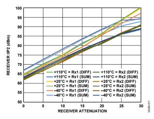
Figure 308. Receiver IIP2 vs. Receiver Attenuation, LO = 3600 MHz, Tones Placed at 3602 MHz and 3692 MHz, -21 dBm Plus Attenuation
