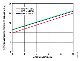
Figure 59. Observation Receiver IIP3, 2f1 – f2 vs. Attenuation, LO = 300 MHz, Tone 1 = 345 MHz, Tone 2 = 346 MHz at -24 dBm Plus Attenuation
