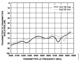
Figure 348. Transmitter to Transmitter Isolation vs. Transmitter LO Frequency, Temperature =  $25^{\circ}$ C
