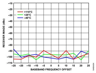
Figure 101. Receiver Image vs. Baseband Frequency Offset, Attenuation = 0 dB, RF Bandwidth = 50 MHz, Tracking Calibration Active, Sample Rate = 61.44 MSPS, LO = 525 MHz
