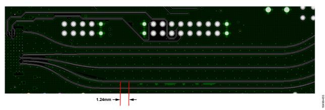
Figure 447. Via Fencing Around JESD204B Lines, PCB Layer 10
