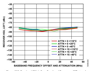
Figure 333. Receiver HD2, Left vs. Baseband Frequency Offset and Attenuation, Tone Level = -15 dBm at Attenuation = 0, X-Axis = Baseband Frequency Offset of the Fundamental Tone, Not the Frequency of the HD2 Product (HD2 Product =  $2 \times$  the Baseband Frequency), HD2 Canceller Disabled, LO = 4600 MHz
