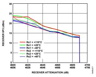
Figure 315. Receiver IIP3 vs. Receiver Attenuation, Receiver Attenuation =  $0 \, dB$ ,  $LO = 4600 \, MHz$ , Tone  $2 = Tone 1 + 1 \, MHz$ ,  $-21 \, dBm Each$ , Swept Across Pass Band
