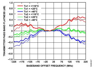
Figure 345. Transmitter Pass Band Flatness vs. Baseband Offset Frequency, Off Chip Match Response De-Embedded, LO = 5700 MHz, Measurements Performed with Device Calibrated at  $25^{\circ}$ C
