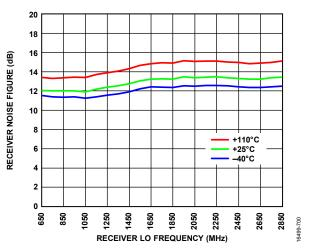
Figure 198. Receiver Noise Figure vs. Receiver LO Frequency, Receiver Attenuation = 0 dB, RF Bandwidth = 200 MHz, Sample Rate = 245.76 MSPS, Integration Bandwidth =  $\pm 100$  MHz
