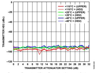
Figure 25. Transmitter HD2 vs. Transmitter Attenuator Setting, Baseband Frequency = 10 MHz, LO = 75 MHz, CW = -15 dBFS
