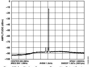
Figure 152. Amplitude vs. Frequency, Transmitter Output Spurious, Transmitter 2 = 650 MHz, LTE = 5 MHz, Offset = 10 MHz, RMS = -12 dBFS, Temperature =  $25^{\circ}$ C
