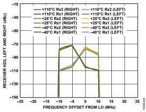
Figure 119. Receiver HD3, Left and Right vs. Frequency Offset from LO, Tone Level = -17 dBm at Attenuation = 0 dB, LO = 300 MHz
