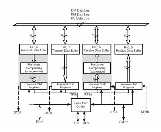
Figure 1. Serial Port Block Diagram
