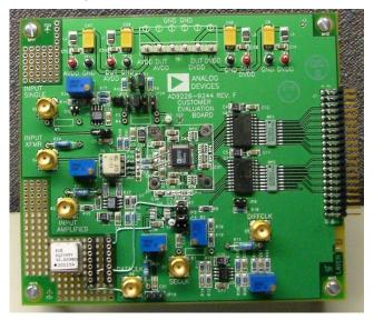
Figure 2. AD9244 ADC Evaluation Board
