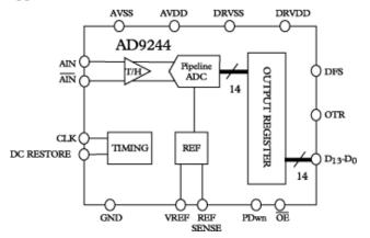
Figure 1. AD9244 Block Diagram
