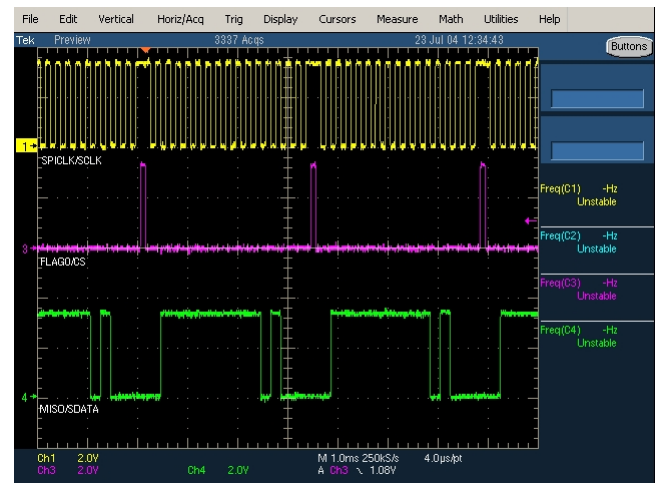
Figure 3. CPHASE=0, CLKPL=1 in Core Mode
