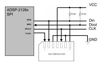
Figure 2. MultiMediaCard Interface with SPI Port
