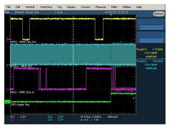
Figure 8. CMD1 Command and R1 Response - 0x00
