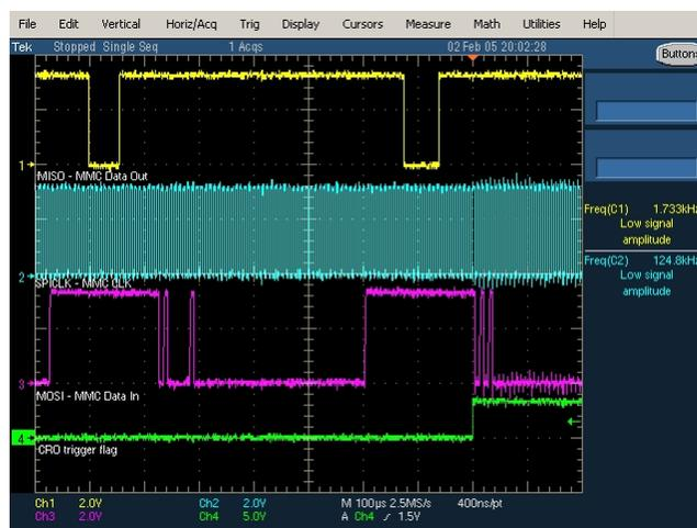
Figure 8. CMD1 Command and R1 Response - 0x00
