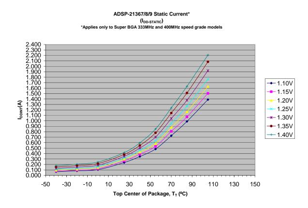
Figure 6 I<sub>DD-STATIC</sub> graph
