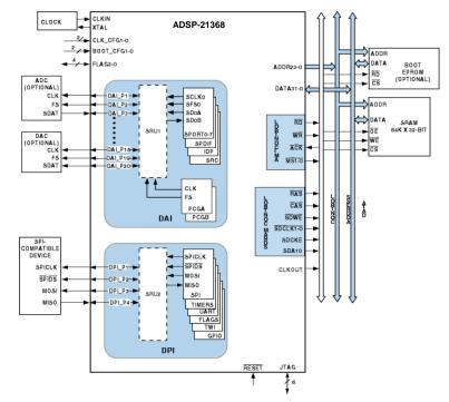
Figure 3. ADSP-21368 system sample configuration
