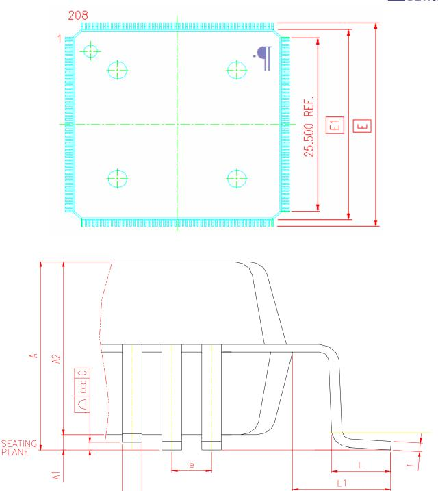
Figure 1. Dimensions of MQFP and LQFP\_EP packages
