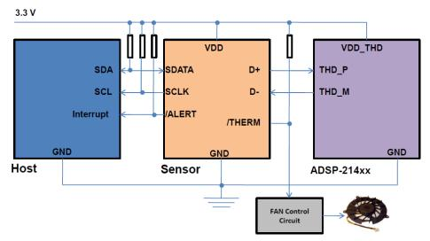
Figure 1. Digital temperature sensor interfaced with an ADSP-214xx processor and a host controller
