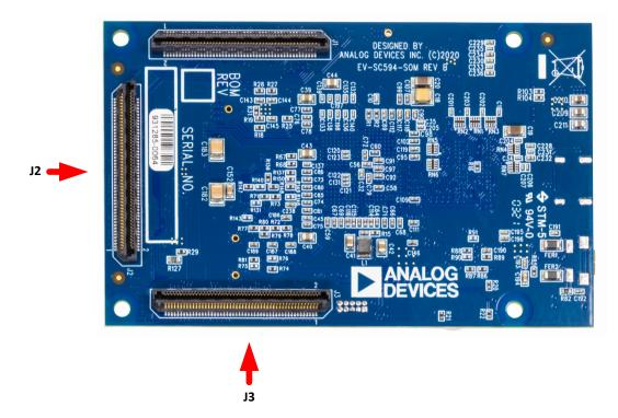
Figure 3-9: Connector Locations Bottom View
