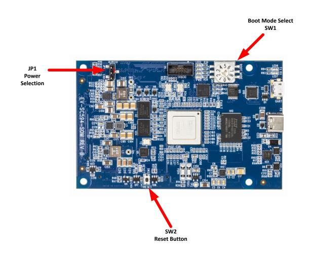
Figure 2-2: Default Hardware Setup
