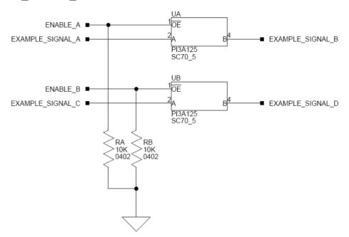
Figure 3-2: Example of Individual FET Switches
