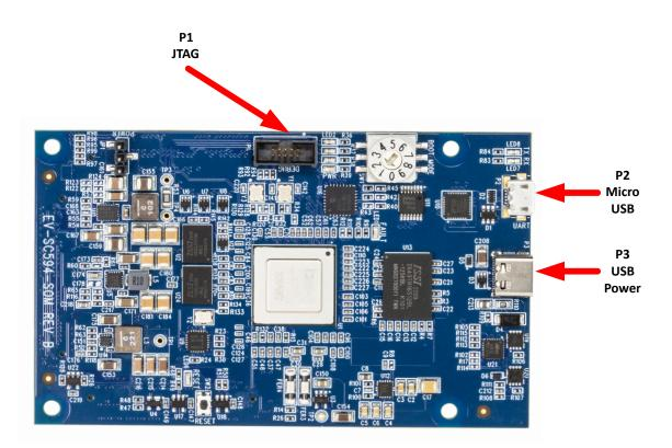
Figure 3-8: Connector Locations Top View
