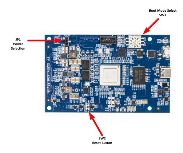
Figure 3-6: Switch/Jumper Locations
