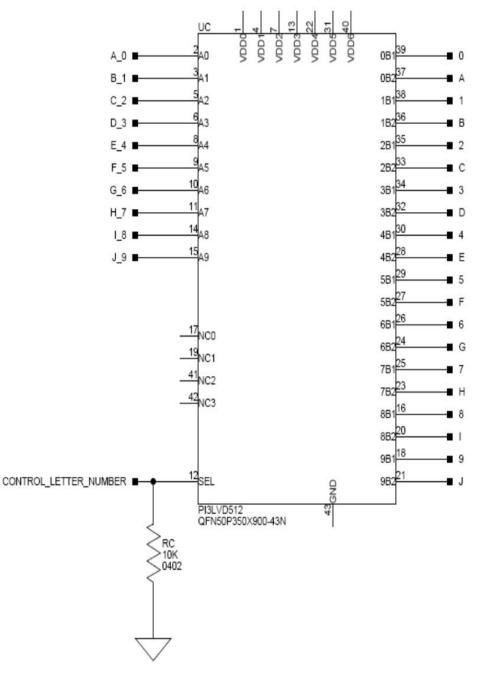
Figure 3-4: Example of a Bus Switch
