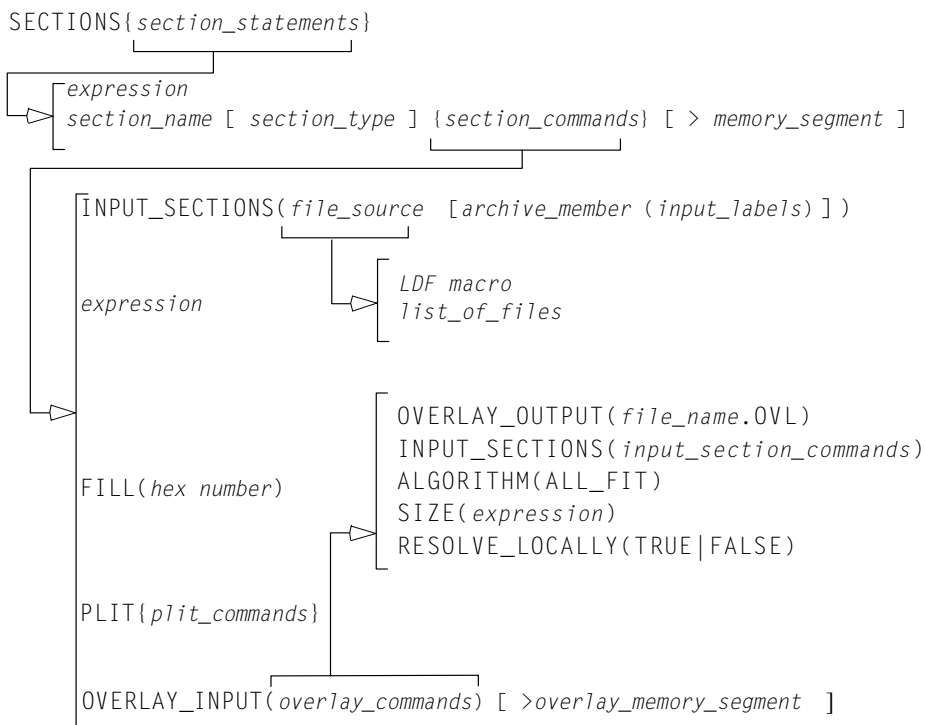
Figure 3-4. Syntax Tree of the SECTIONS{} Command
