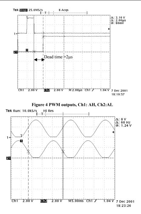
Figure 5 Filtered PWM outputs (over modulation) Ch1: AH, Ch2: AL
