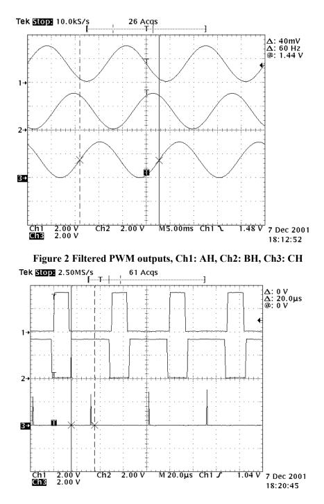
Figure 3 PWM outputs, Ch1: AH, Ch2: AL, Ch3: PWMSYNC
