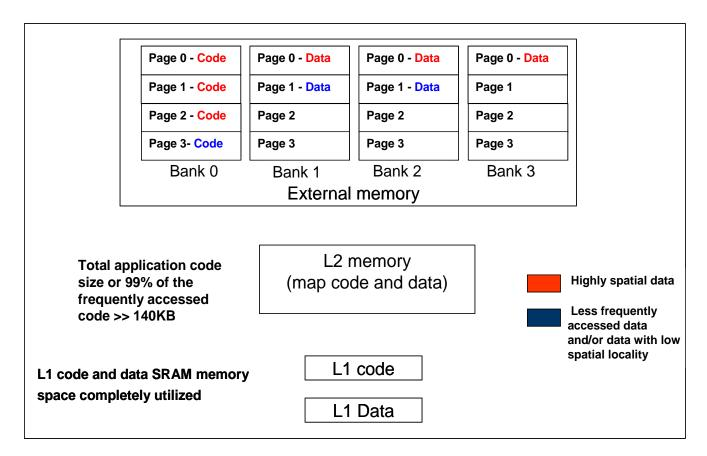
Figure 4. Placing code in only one SDRAM internal memory bank page
