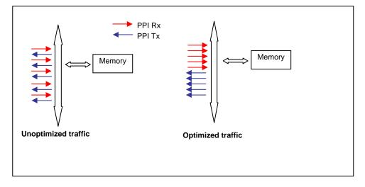
Figure 7. Optimizing DMA traffic over the system buses
