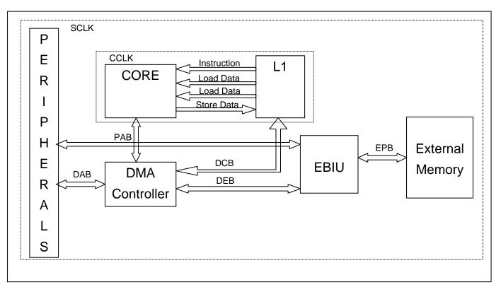
Figure 6. Internal bus structure for ADSP-BF53x/ADSP-BF52x Blackfin processors. For the ADSP-BF561 processor, there are two cores, two DMA controllers, and a block of L2 memory.
