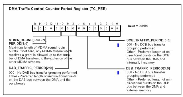
Figure 8. DMA traffic control register
