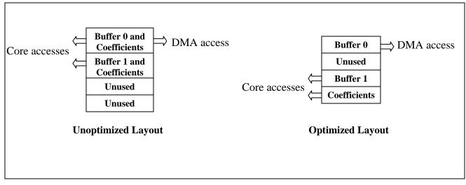
Figure 2. Efficient use of multi-ported sub-bank internal memory architecture
