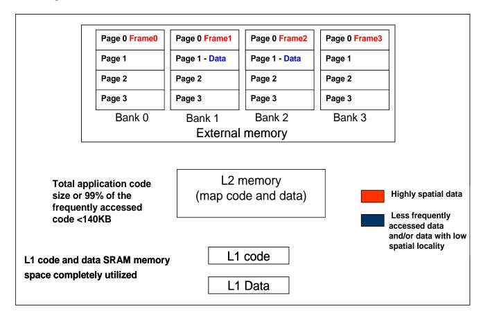
Figure 5. Placing frame buffers in four different SDRAM internal banks
