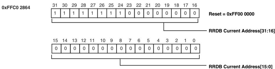
Figure 21-37. MXVR Remote Read Buffer Current Address Register (MXVR\_RRDB\_CURR\_ADDR)
