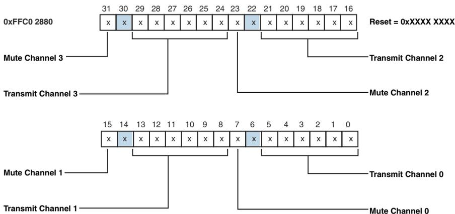
Figure 21-41. MXVR Routing Register 0 (MXVR\_ROUTING\_0)
