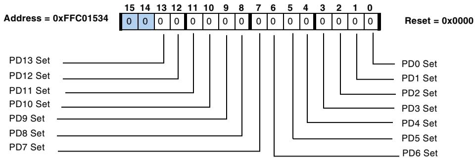
Figure 15-17. GPIO Port D Set Register
