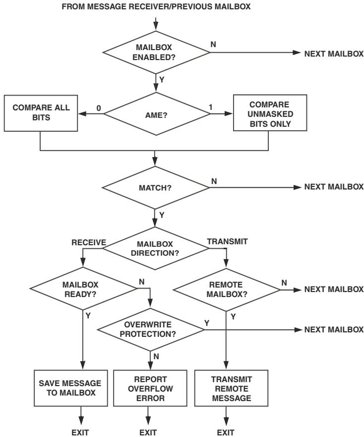
Figure 19-10. CAN Receive Operation Flow Chart
