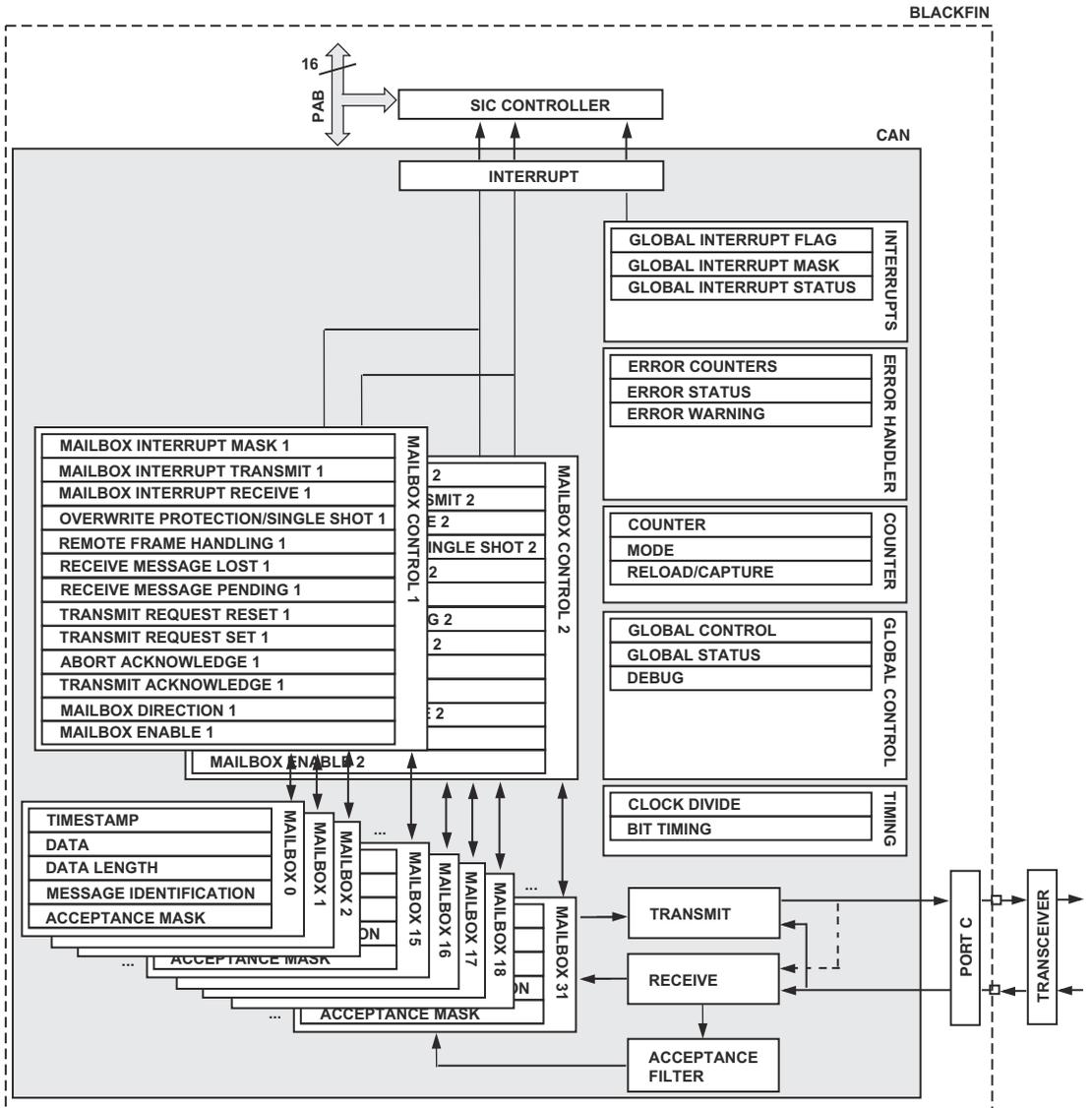
Figure 19-2. CAN Block Diagram
