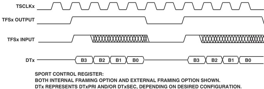
Figure 12-38. SPORT Transmit, Alternate Framing
