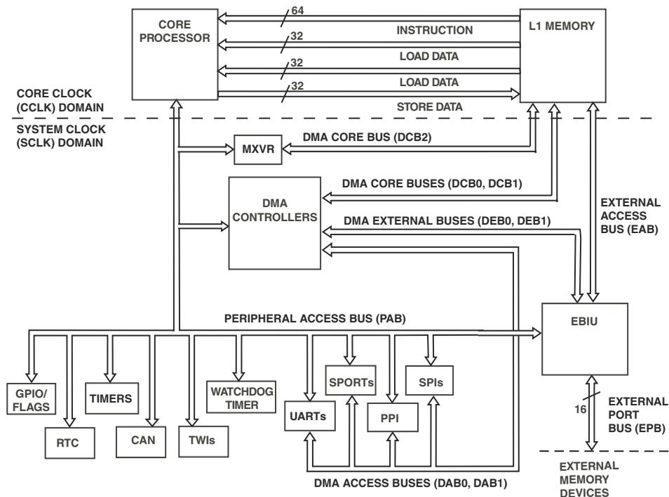
Figure 6-2. Processor Memory Architecture
