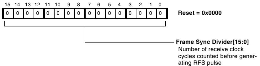
Figure 12-15. SPORTx Receive Frame Sync Divider Register
