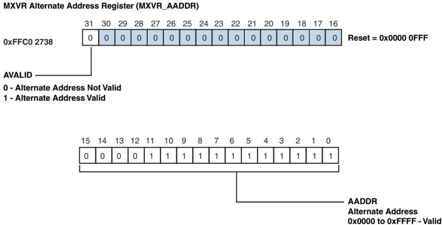
Figure 21-18. MXVR Alternate Address Register (MXVR\_AADDR)
