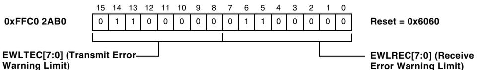
Figure 19-63. Error Counter Warning Level Register
