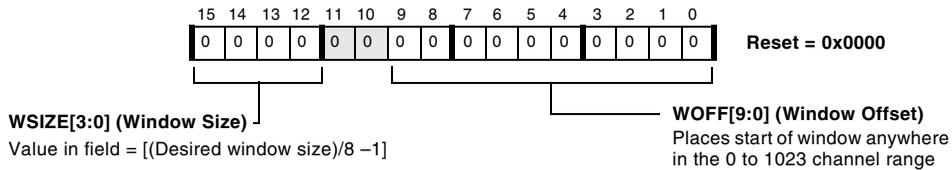
Figure 12-23. SPORTx Multichannel Configuration Register 1
