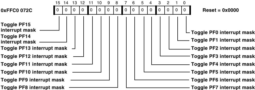
Figure 14-14. Flag Mask Interrupt B Toggle Register
