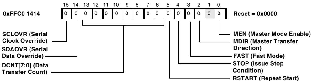
Figure 20-7. TWI Master Mode Control Registers
