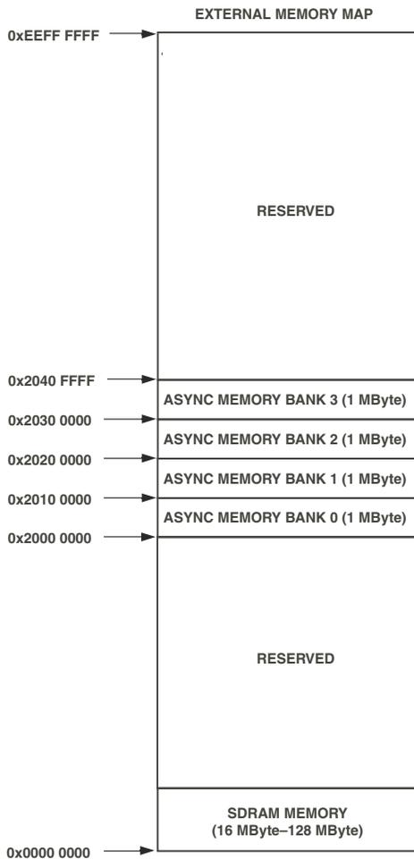
**NOTE: RESERVED OFF-CHIP MEMORY AREAS ARE LABELED IN THE DIAGRAM ABOVE. ALL OTHER OFF-CHIP SYSTEM RESOURCES ARE ADDRESSABLE BY BOTH THE CORE AND THE SYSTEM.**
