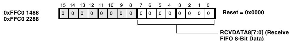
Figure 20-17. TWI FIFO Receive Data Single Byte Registers
