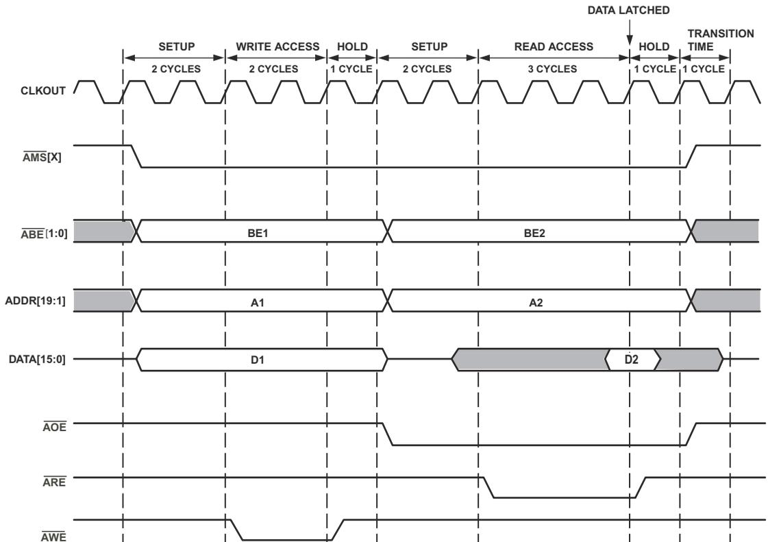
Figure 18-9. Asynchronous Write and Read Bus Cycles
