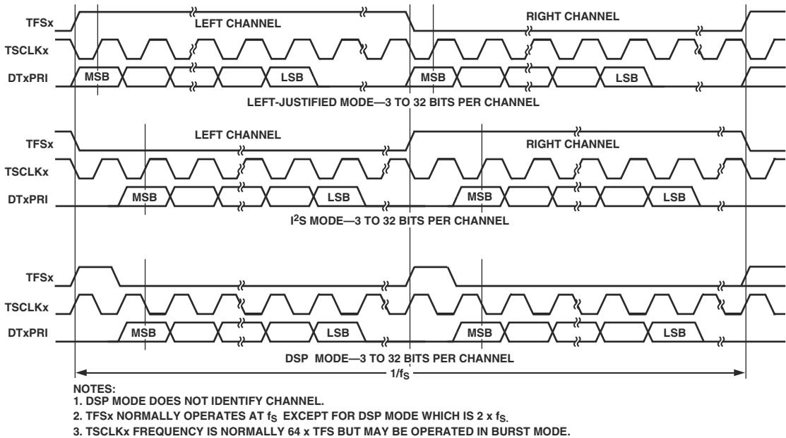
Figure 12-20. SPORT Stereo Serial Modes, Transmit
