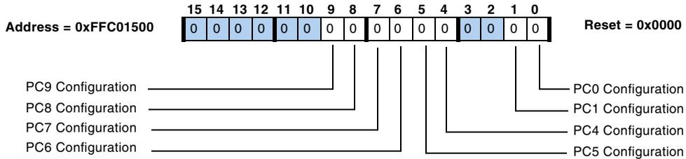
PC1 and PC4 are 5V-tolerant. When configured as outputs, they behave as open-drains.
