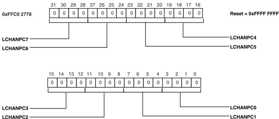
Figure 21-20. MXVR Synchronous Logical Channel Assignment Register (MXVR\_SYNC\_LCHAN\_0)
