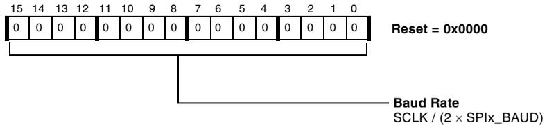
Figure 10-3. SPI Baud Rate Registers
