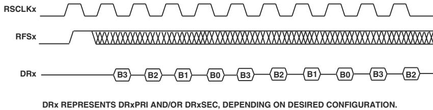
Figure 12-34. SPORT Receive, Unframed Mode, Normal Framing
