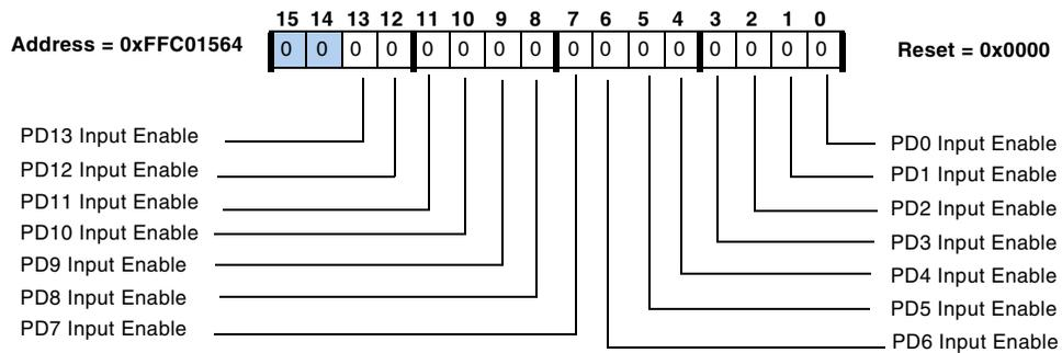
Figure 15-8. GPIO Port D Input Enable Register
