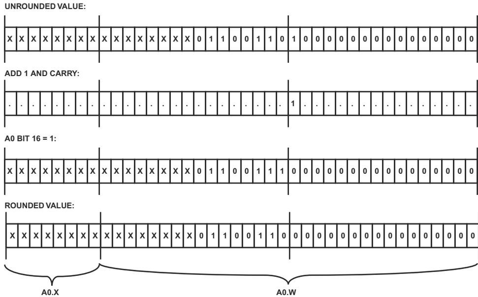
Figure 2-7. Avoiding Net Bias in Unbiased Multiplier Rounding
