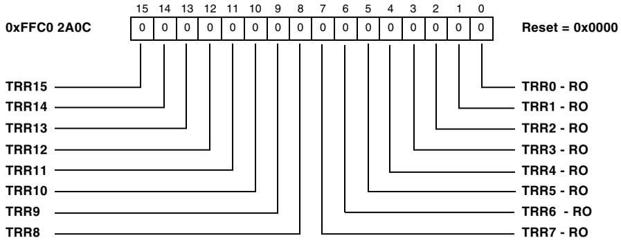
Figure 19-43. Transmission Request Reset Register 1
