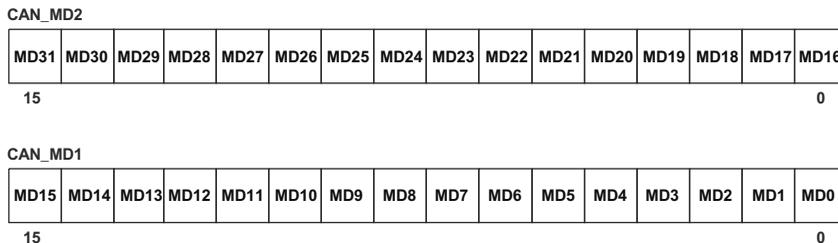
Figure 19-4. CAN Register Pairs
