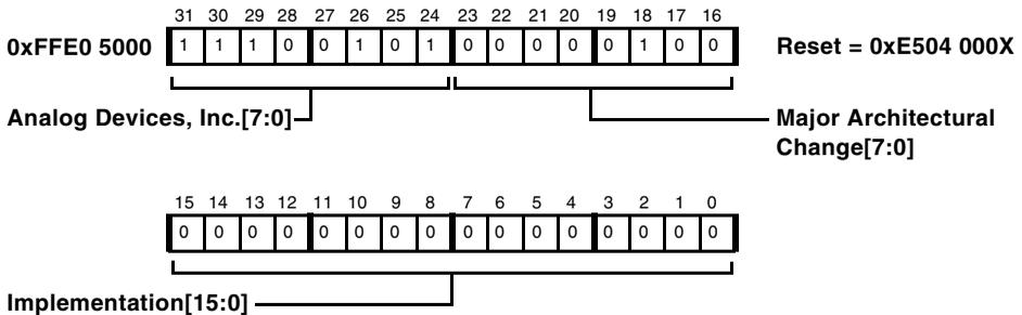
Figure 23-15. DSP Device ID Register
