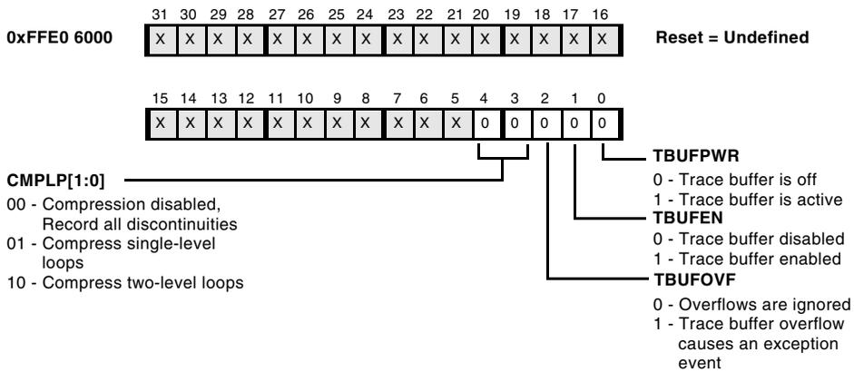
Figure 23-9. Trace Buffer Control Register
