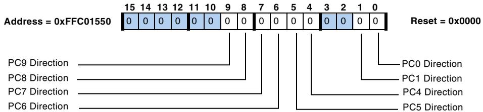
PC1 and PC4 can be used as GPIO. However, they differ from the rest of the PCx pins because they are 5V-tolerant input/open-drain output. When configured as outputs, they are open-drain outputs only.
