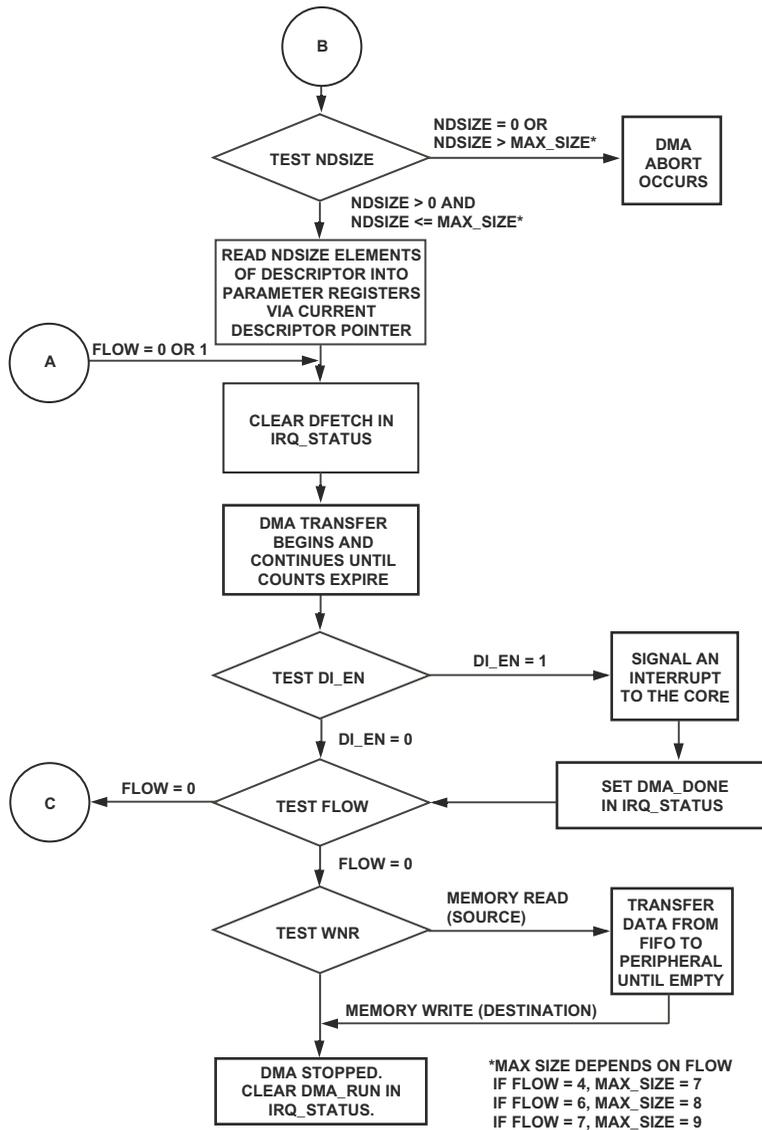
Figure 9-17. DMA Flow, from DMA Controller point of view (2 of 2)
