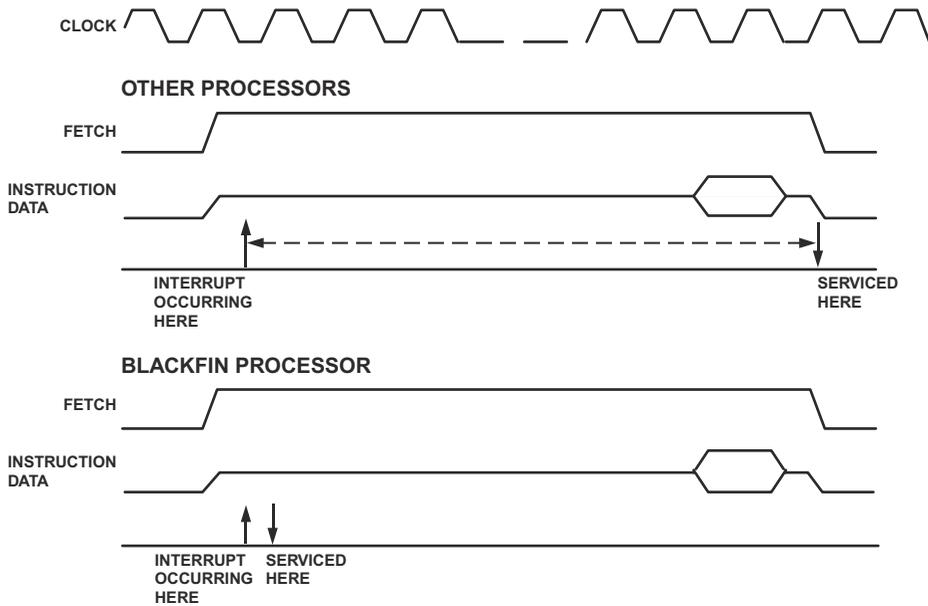
Figure 4-24. Minimizing Latency in Servicing an ISR
