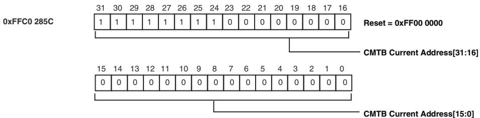
Figure 21-35. MXVR Control Message Transmit Buffer Current Address Register (MXVR\_CMTB\_CURR\_ADDR)
