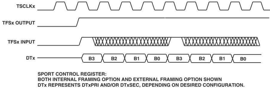
Figure 12-39. SPORT Continuous Transmit, Alternate Framing
