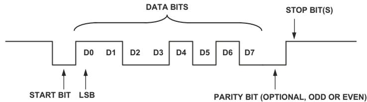
Figure 13-1. Bitstream on the TXx Pin
