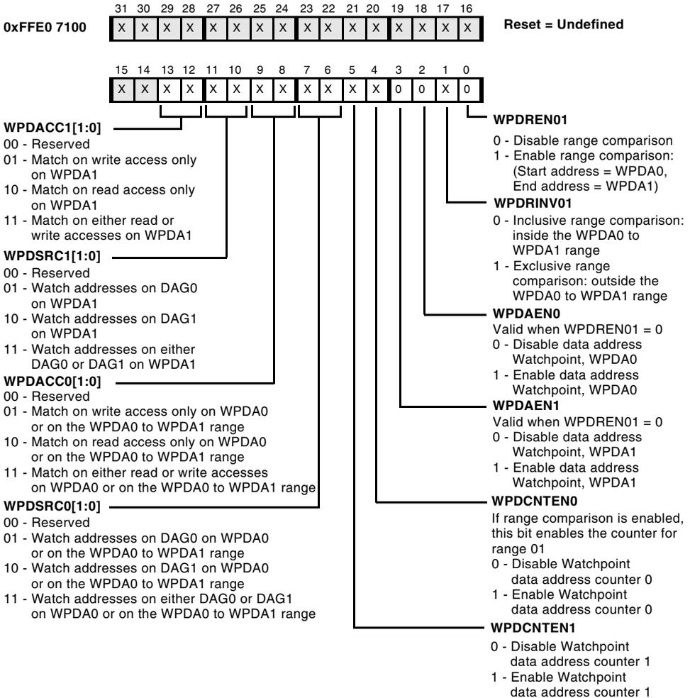
Figure 23-7. Data Watchpoint Address Control Register
