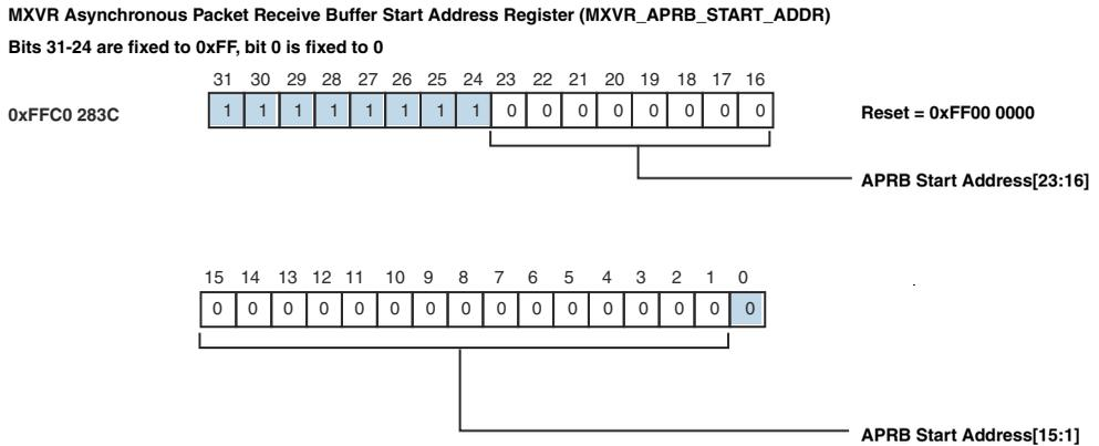
Figure 21-27. MXVR APRB Start Address Register (MXVR\_APRB\_START\_ADDR)
