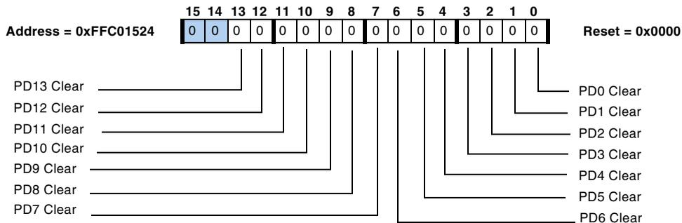
Figure 15-14. GPIO Port D Clear Register
