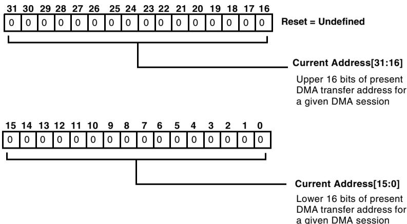
Figure 9-9. Current Address Register
