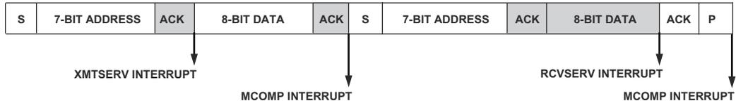
Figure 20-25. Transmit/Receive Data Repeated Start
