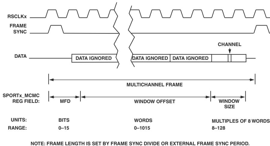
Figure 12-25. Relationships for Multichannel Parameters
