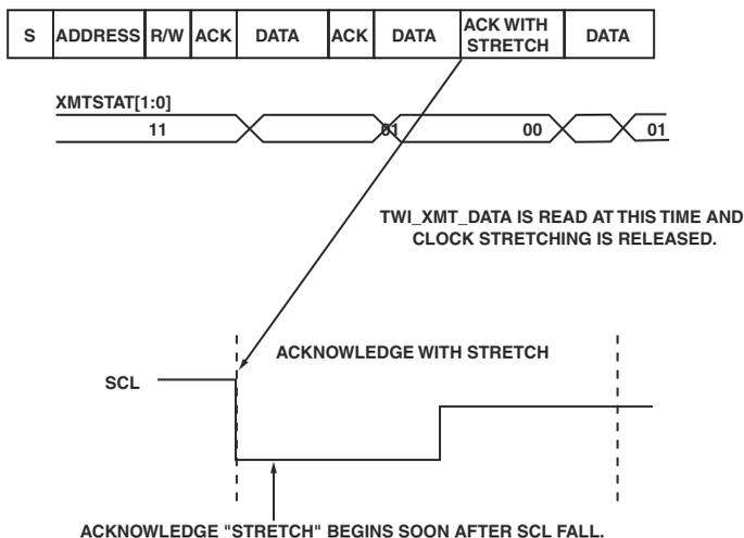
Figure 20-27. Clock Stretching During FIFO Underflow
