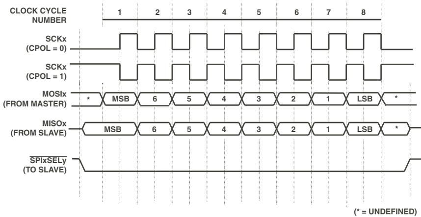
Figure 10-12. SPI Transfer Protocol for CPHA = 0
