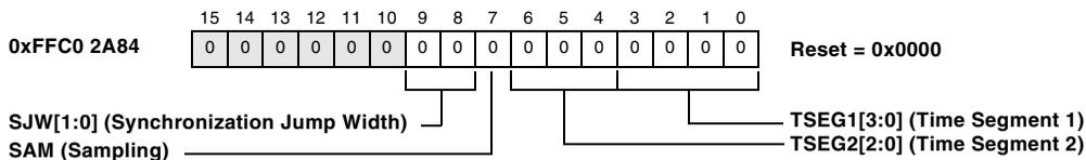
Figure 19-16. CAN Timing Register
