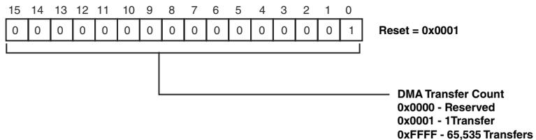
Figure 21-24. MXVR DMA Channel x Transfer Count Registers (MXVR\_DMAx\_COUNT)
