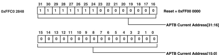
Figure 21-30. MXVR Asynchronous Packet Transmit Buffer Current Address Register (MXVR\_APTB\_CURR\_ADDR)
