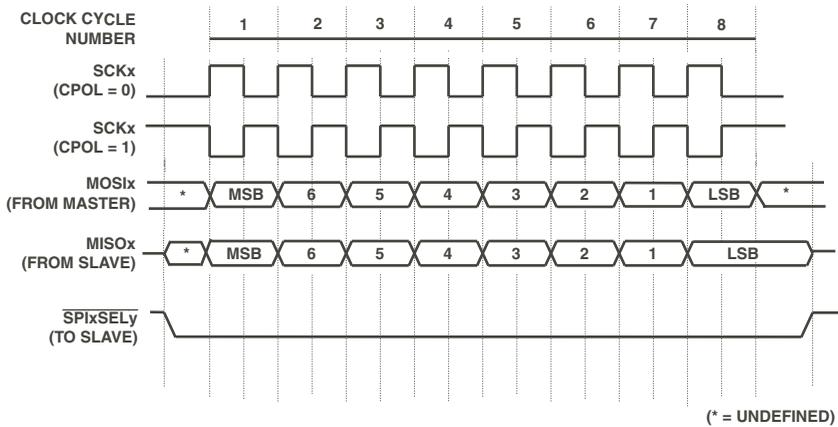
Figure 10-13. SPI Transfer Protocol for CPHA = 1
