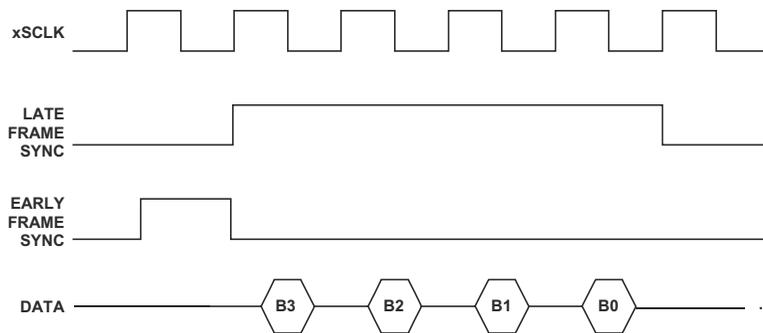
Figure 12-19. Normal Versus Alternate Framing
