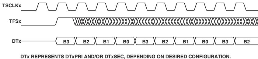
Figure 12-41. SPORT Transmit, Unframed Mode, Alternate Framing
