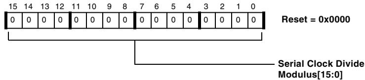
Figure 12-12. SPORTx Transmit Serial Clock Divider Register
