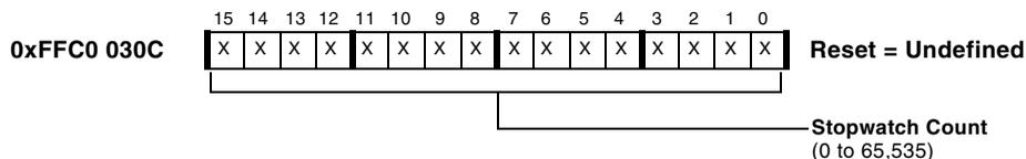
Figure 17-7. RTC Stopwatch Count Register
