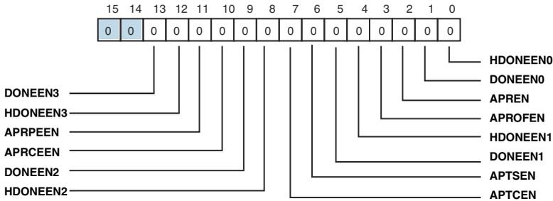
Figure 21-11. MXVR Interrupt Enable Register 1 (MXVR\_INT\_EN\_1)
