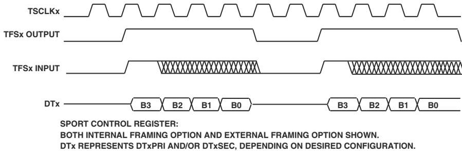
Figure 12-36. SPORT Transmit, Normal Framing
