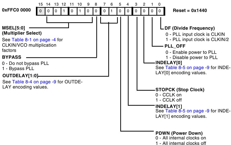
Figure 8-3. The PLL Control Register
