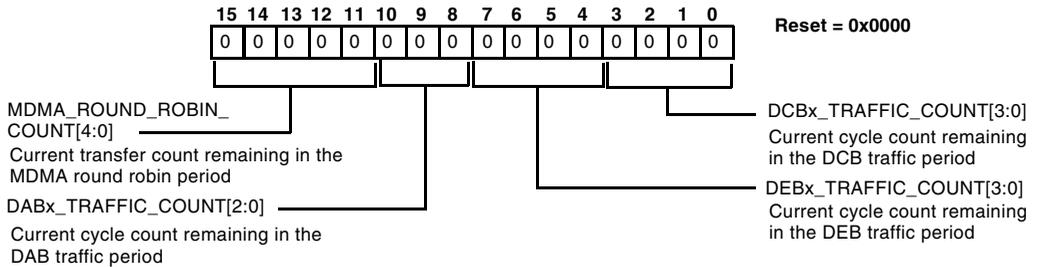
Figure 9-19. DMA Traffic Control Counter Register
