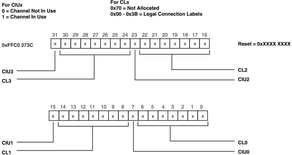
Figure 21-19. MXVR Allocation Table Register (MXVR\_ALLOC\_0)
