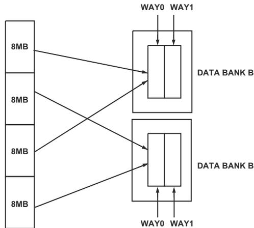
Figure 6-12. Data Cache Mapping When DCBS = 1
