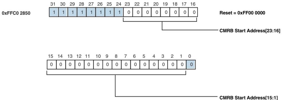
Figure 21-32. MXVR Control Message Receive Buffer Start Address Register (MXVR\_CMRB\_START\_ADDR)
