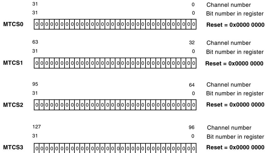
Figure 12-29. SPORTx Multichannel Transmit Select Registers
