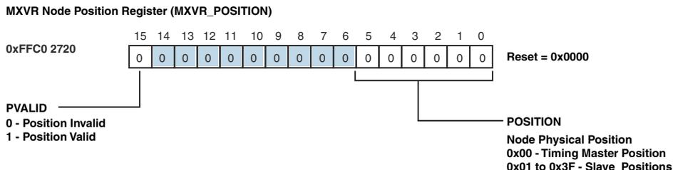
Figure 21-13. MXVR Maximum Node Position Register
