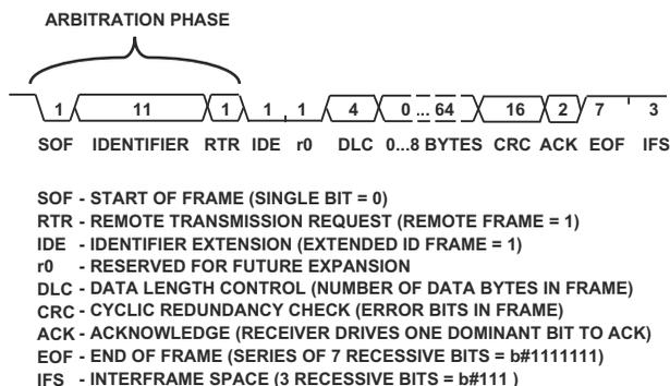
Figure 19-5. Standard CAN Frame
