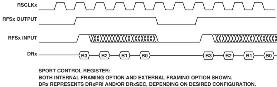
Figure 12-32. SPORT Receive, Alternate Framing
