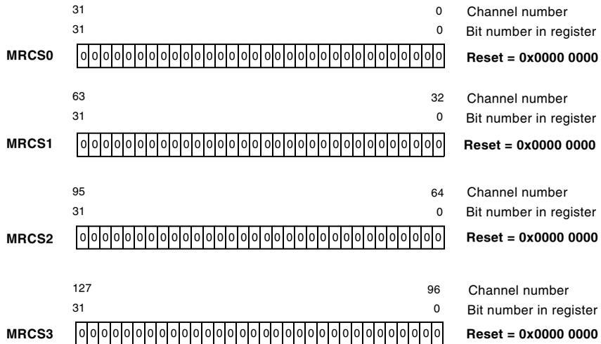
Figure 12-28. SPORTx Multichannel Receive Select Registers
