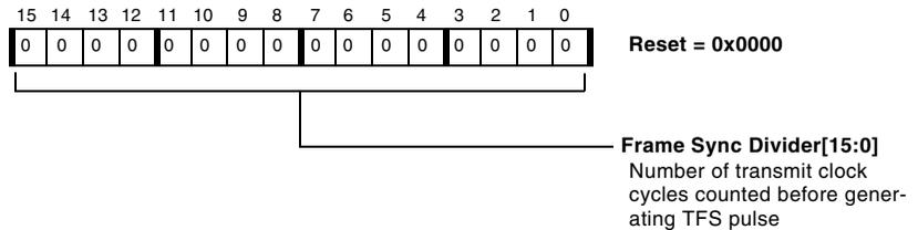
Figure 12-14. SPORTx Transmit Frame Sync Divider Register
