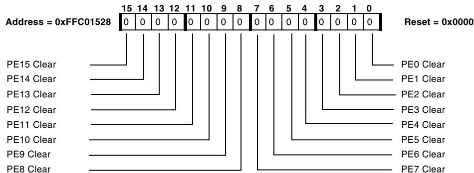
Figure 15-15. GPIO Port E Clear Register
