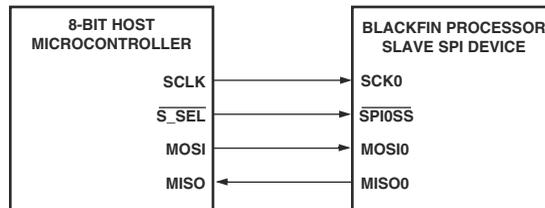
Figure 10-2. ADSP-BF539 Blackfin Processor as a Slave SPI Device
