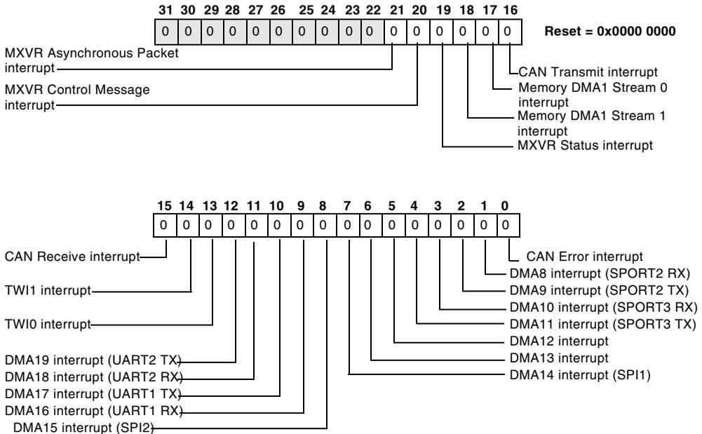
Figure 4-9. System Interrupt Status Register 1 (SIC\_ISR1)
