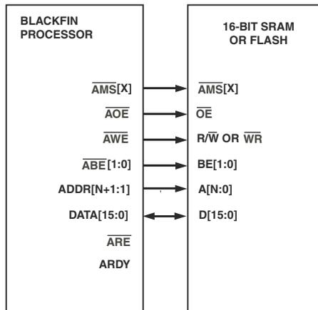
Figure 22-2. Interface to 16-bit SRAM or Flash
