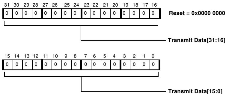
Figure 12-9. SPORTx Transmit Data Register
