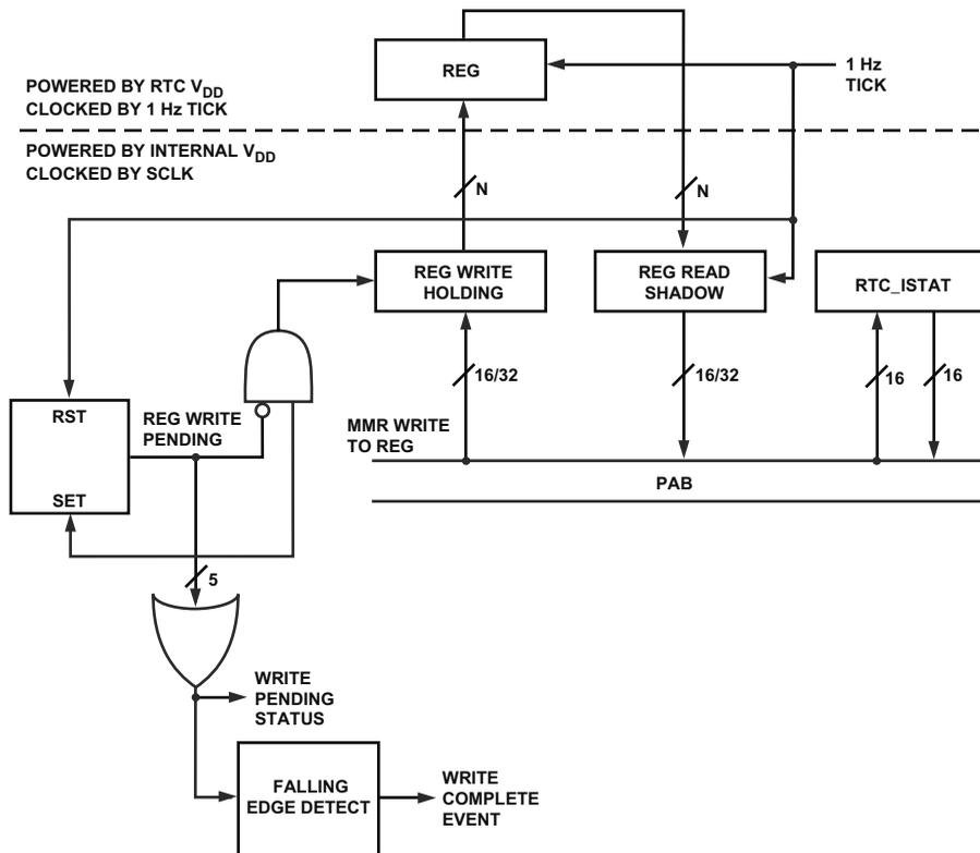
Figure 17-2. RTC Register Architecture
