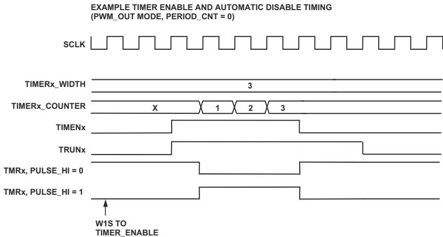
Figure 16-11. Timer Enable and Automatic Disable Timing
