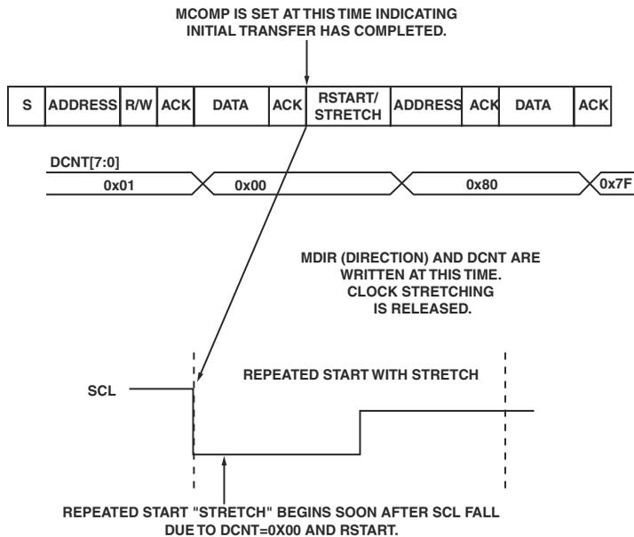
Figure 20-29. Clock Stretching During Repeated Start Condition
