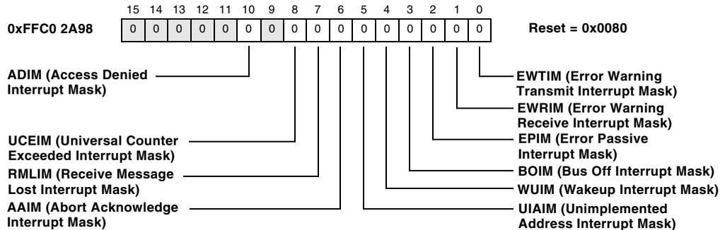
Figure 19-18. Global CAN Interrupt Mask Register
