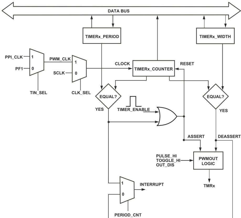
Figure 16-12. Timer Flow Diagram, PWM\_OUT Mode
