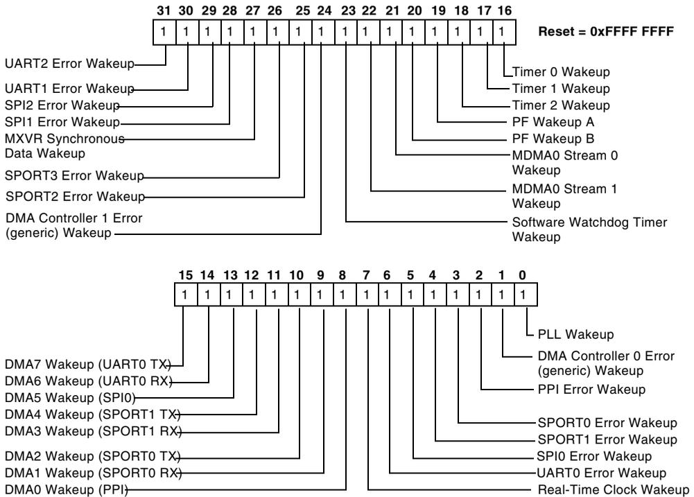
Figure 4-6. System Interrupt Wakeup-Enable Register 0 (SIC\_IWR0)
