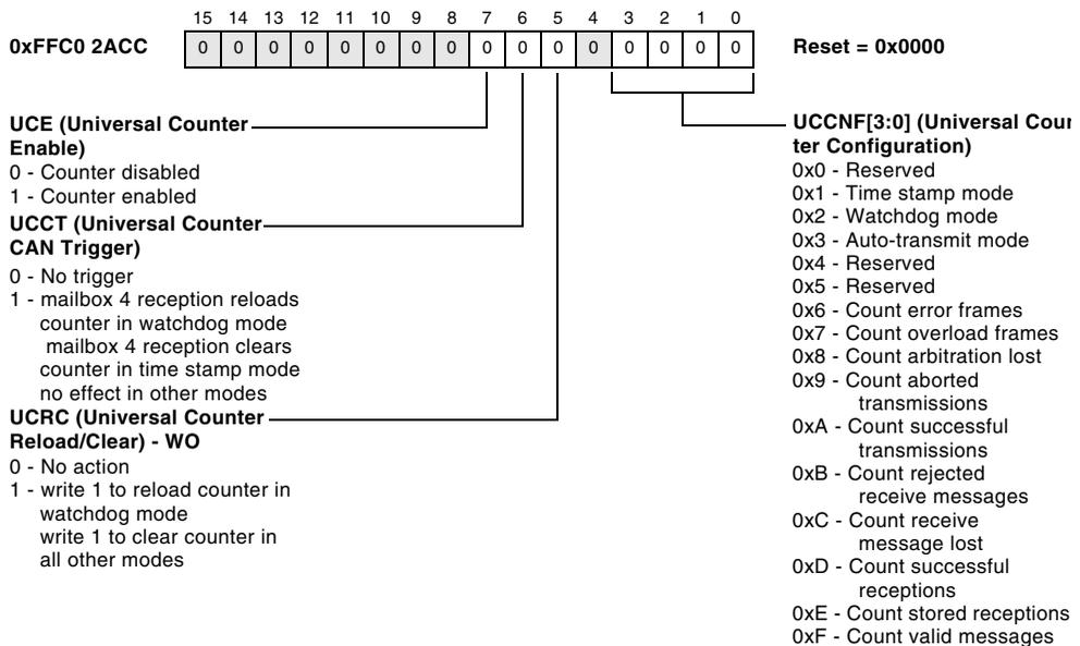
Figure 19-58. Universal Counter Configuration Mode Register
