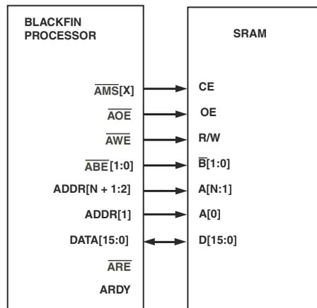
Figure 22-3. Interface to 16-bit SRAM
