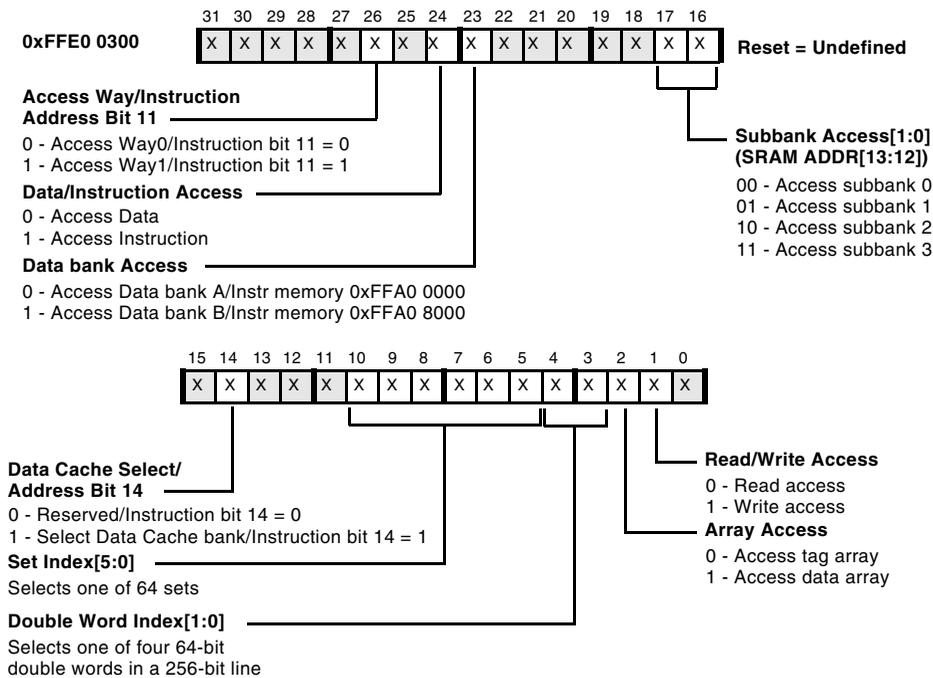
Figure 6-14. Data Test Command Register
