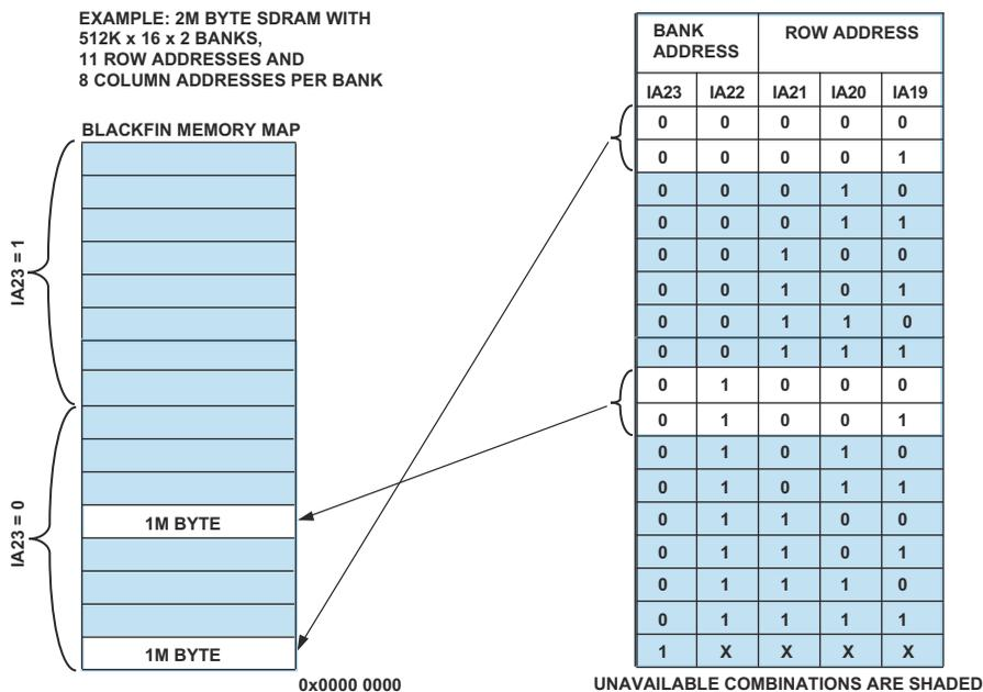
Figure 22-4. Using Small SDRAMs
