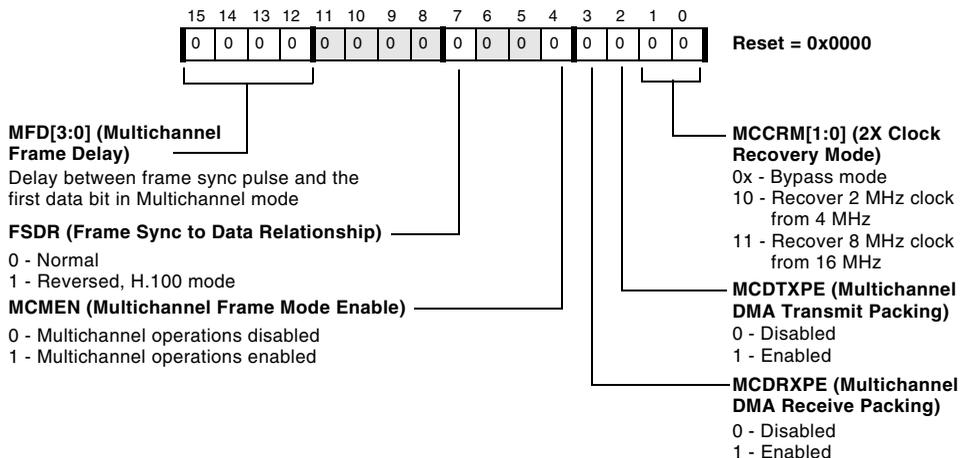
Figure 12-24. SPORTx Multichannel Configuration Register 2
