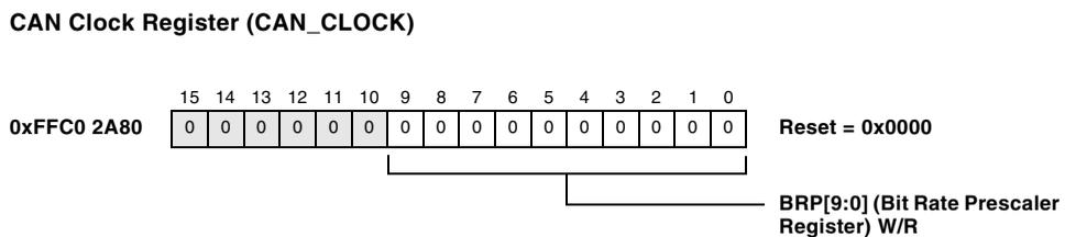
Figure 19-15. CAN Clock Register
