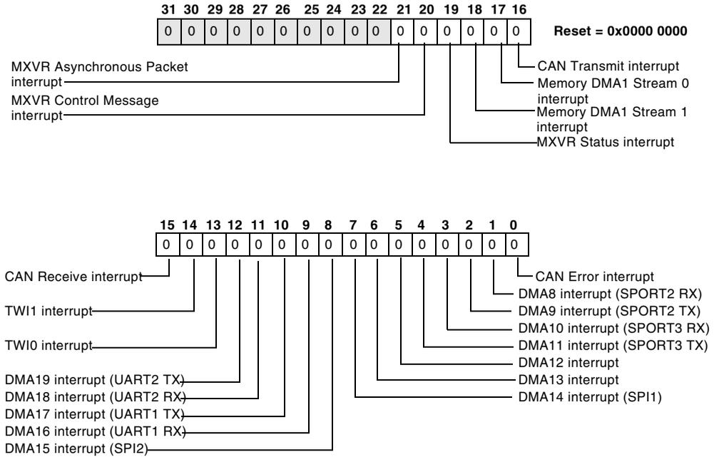
Figure 4-11. System Interrupt Mask Register 1 (SIC\_IMASK1)
