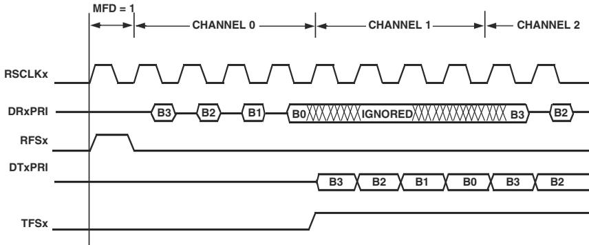
Figure 12-22. Multichannel Operation
