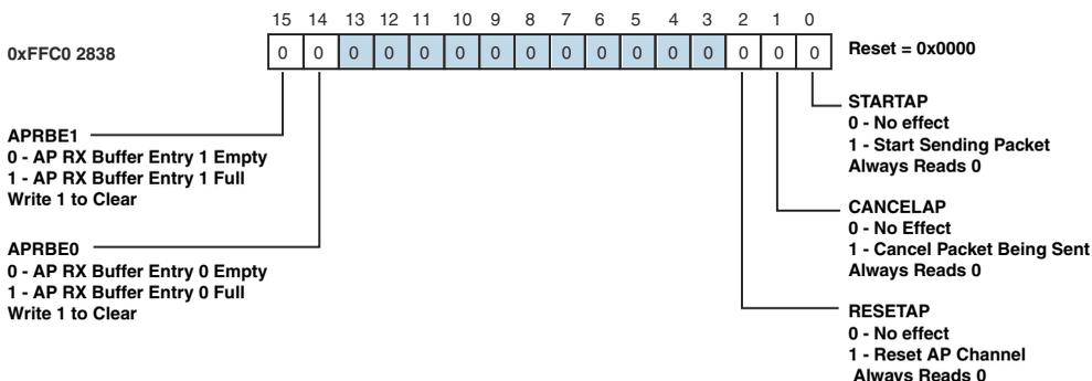
Figure 21-26. MXVR Asynchronous Packet Control Register (MXVR\_AP\_CTL)
