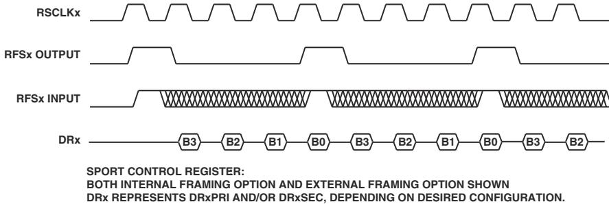
Figure 12-31. SPORT Continuous Receive, Normal Framing
