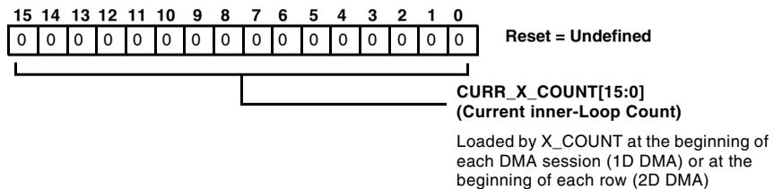
Figure 9-10. Current Inner Loop Count Register
