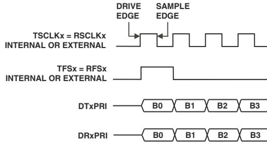
Figure 12-17. Example of  $TCKFE = RCKFE = 0$ , Transmit and Receive Connected
