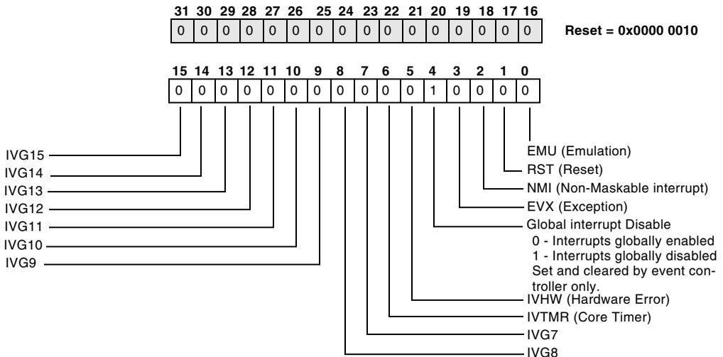
Figure 4-21. Core Interrupt Pending Register
