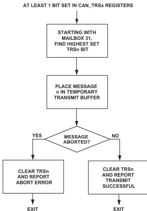
Figure 19-8. CAN Transmit Operation Flow Chart
