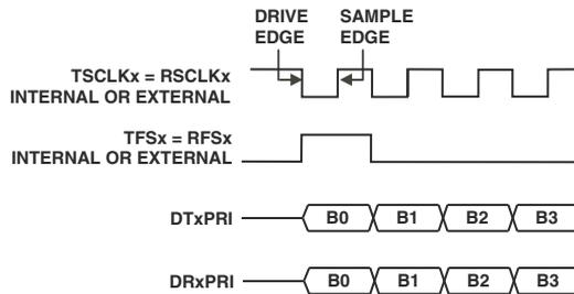
Figure 12-18. Example of  $TCKFE = RCKFE = 1$ , Transmit and Receive Connected
