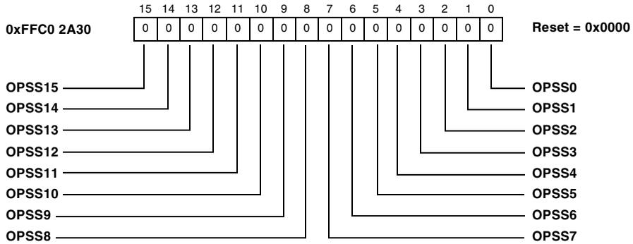
Figure 19-39. Overwrite Protection/Single Shot Transmission Register 1
