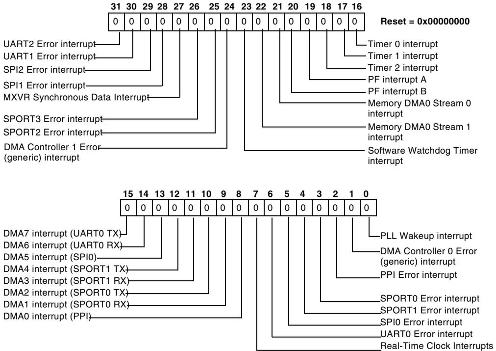
Figure 4-8. System Interrupt Status Register 0 (SIC\_ISR0)
