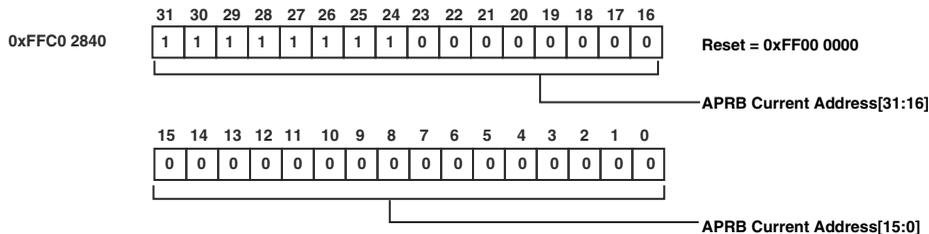
Figure 21-28. MXVR Asynchronous Packet Receive Buffer Current Address Register (MXVR\_APRB\_CURR\_ADDR)
