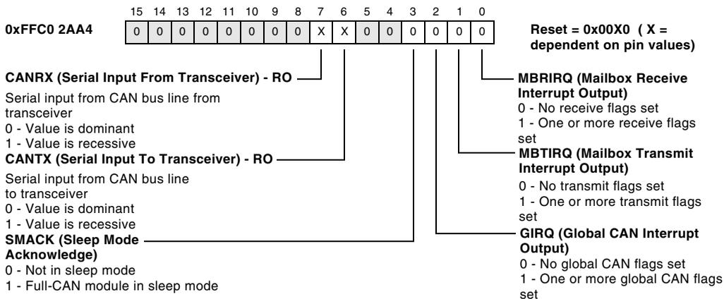
Figure 19-17. CAN Interrupt Register
