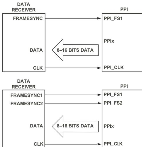
Figure 11-14. TX Mode, 1 or 2 External Frame Syncs
