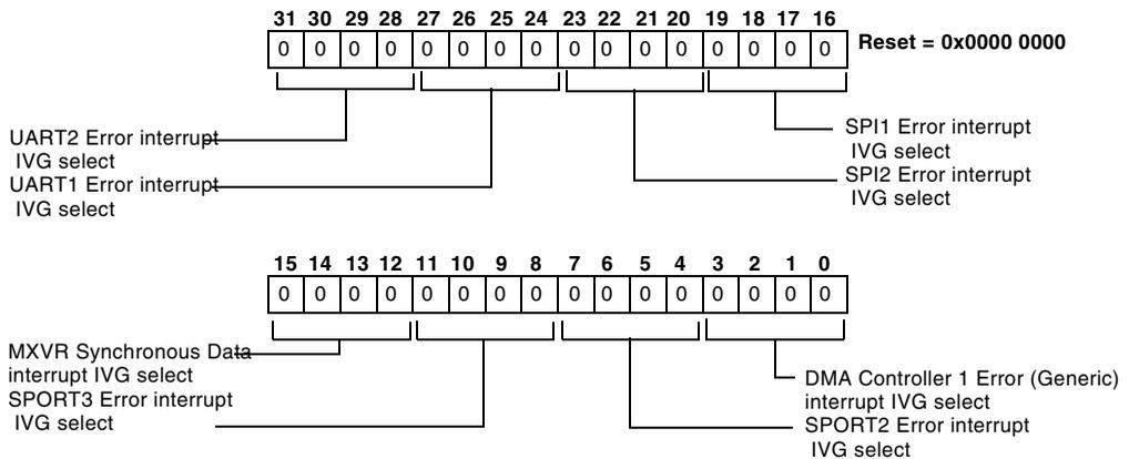
Figure 4-15. System Interrupt Assignment Register 3 (SIC\_IAR3)
