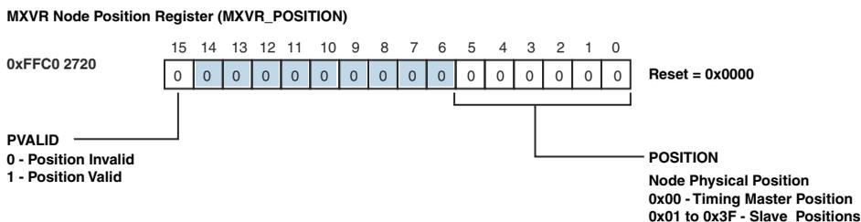
Figure 21-12. MXVR Node Position Register (MXVR\_POSITION)
