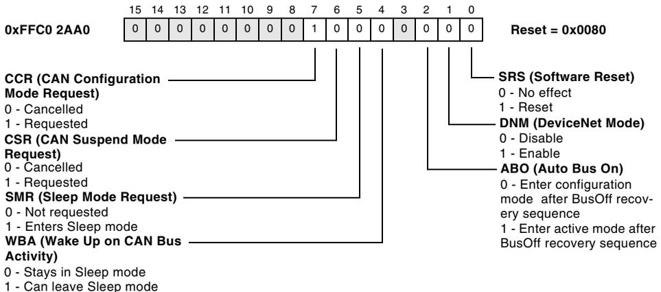
Figure 19-12. Master Control Register
