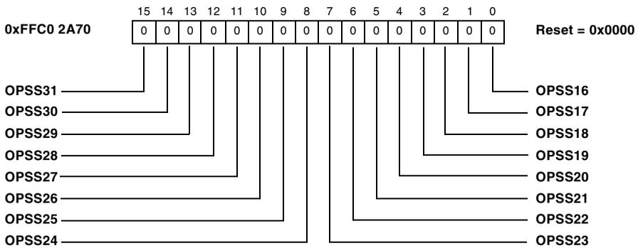
Figure 19-40. Overwrite Protection/Single Shot Transmission Register 2
