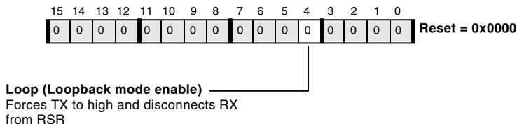
Figure 13-3. UART Modem Control Register
