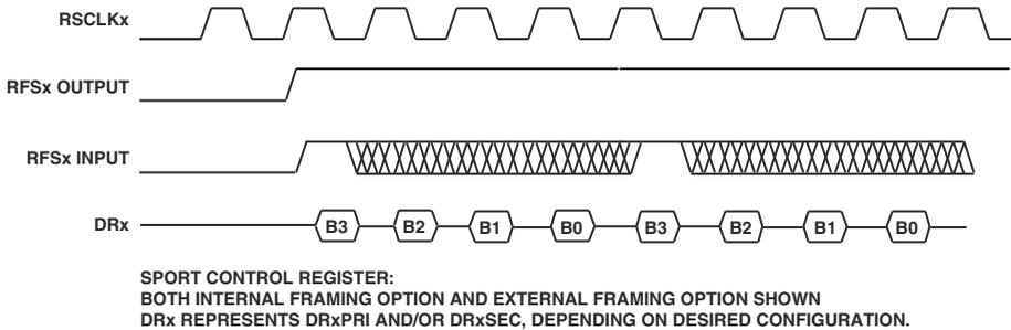
Figure 12-33. SPORT Continuous Receive, Alternate Framing
