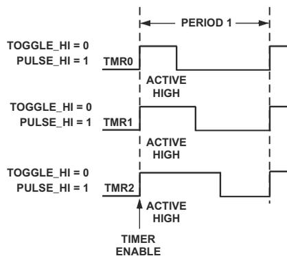
Figure 16-13. Timers With Pulses Aligned to Asserting Edge
