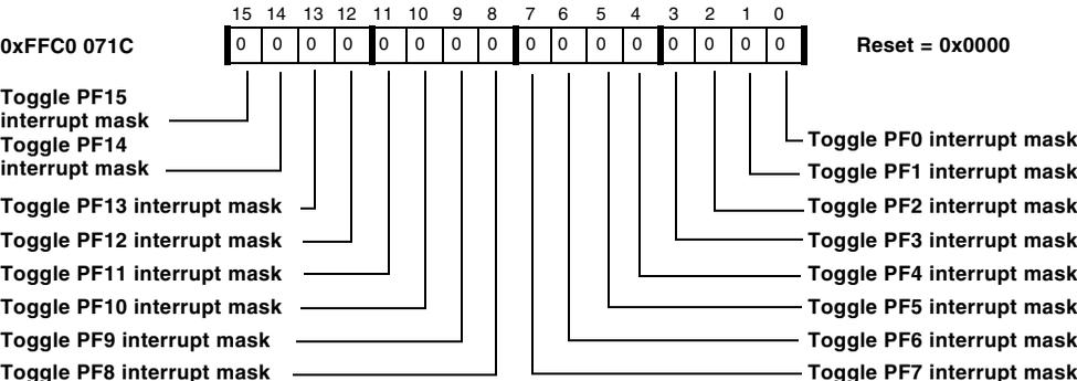
Figure 14-10. Flag Mask Interrupt A Toggle Register
