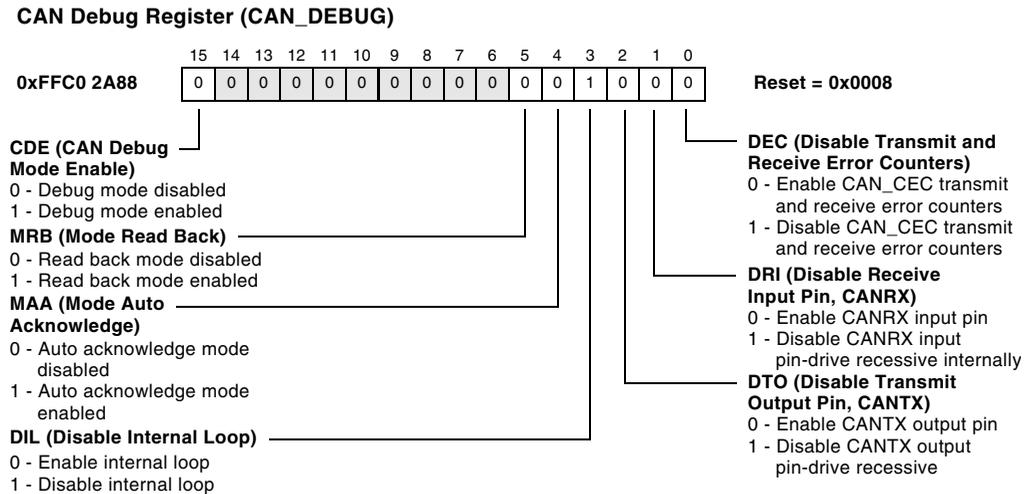
Figure 19-14. CAN Debug Register
