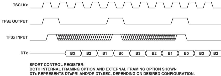
Figure 12-37. SPORT Continuous Transmit, Normal Framing
