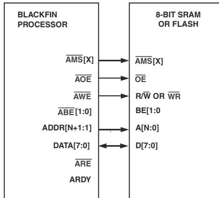
Figure 22-1. Interface to 8-bit SRAM or Flash
