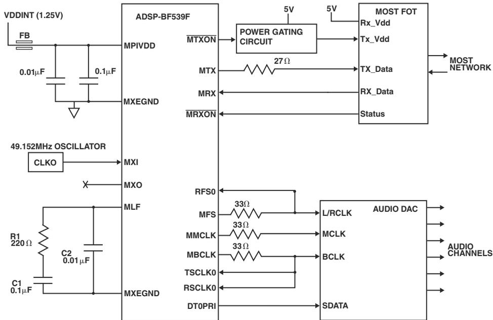
Figure 21-1. Example Connections of ADSP-BF539 to MOST Network
