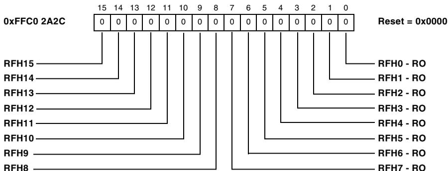
Figure 19-50. Remote Frame Handling Register 1
