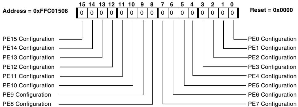
Figure 15-3. GPIO Port E Configuration Register
