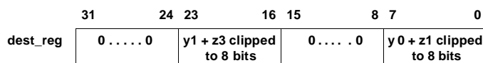
Figure 8-44: The versions that load the result into the lower byte (LO) produce:
