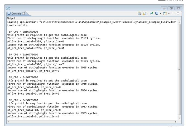
Figure 1. Console Output from Example Program
