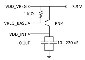
Figure 1. Voltage Regulator External Circuitry Design
