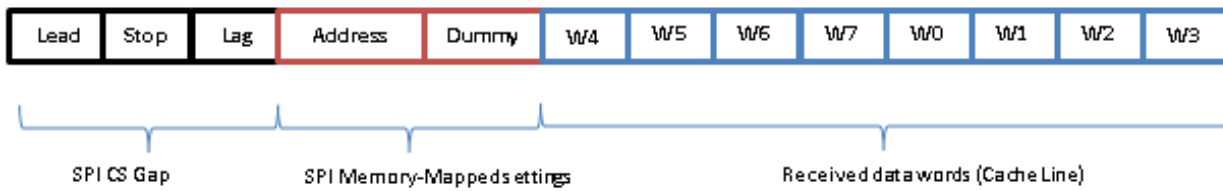
Figure 11. 32-Byte Cache Line (Wrap Mode On, Command Skip On, Word 4 Requested by the Processor)
