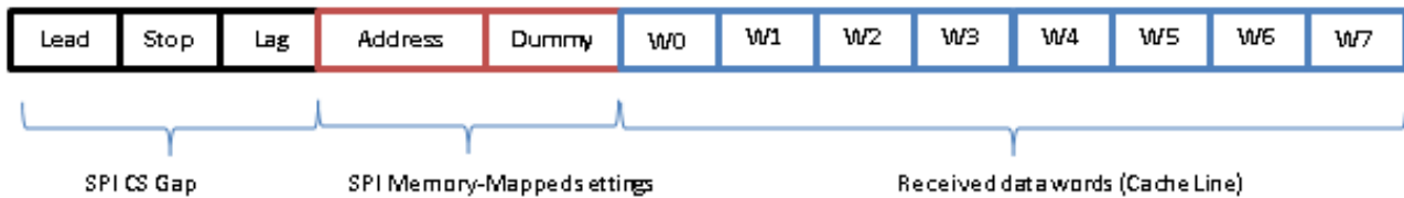
Figure 12. 32-Byte Cache Line (Wrap Mode Off, Command Skip On, Word 4 Requested by the Processor)
