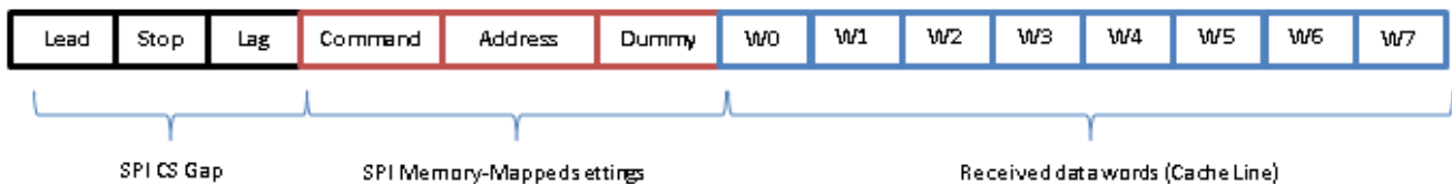
Figure 10. 32-Byte Cache Line (Wrap Mode Off, Command Skip Off, Word 4 Requested by the Processor)
