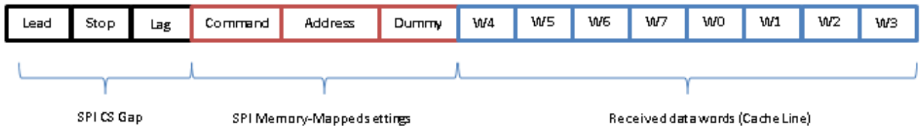
Figure 9. 32-Byte Cache Line (Wrap Mode On, Command Skip Off, Word 4 Requested by Processor)
