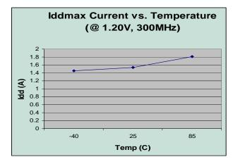
Figure 2: IDDMAX Current vs. Temperature
