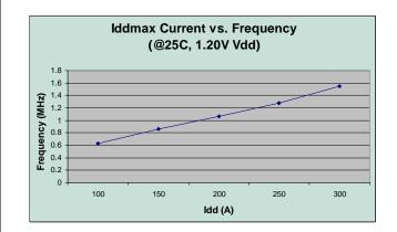
Figure 3: IDDMAX Current vs. Frequency
