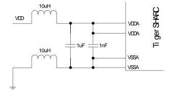
*Figure 4. Analog power supply filtering circuit reference design*
