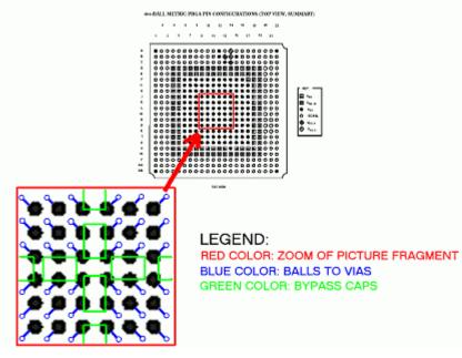
Figure 5. Bypass capacitors layout scheme
