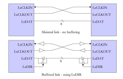
Figure 6. Buffered link port configuration
