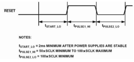
Figure 1. Power-up Reset Waveform
