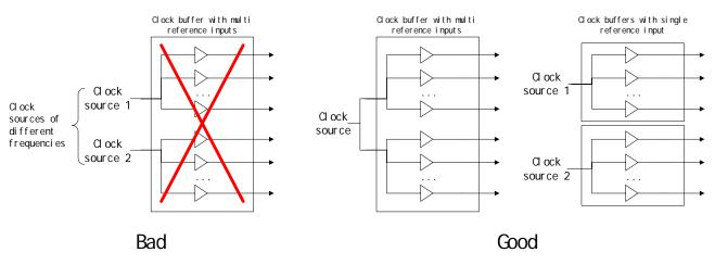
Figure 2. Using fan-out buffers
