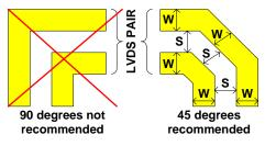
Figure 15. No 90-Deg Angles for LVDS signals
