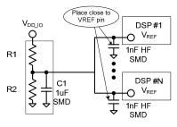
Figure 2. Recommended V<sub>REF</sub> Circuit
