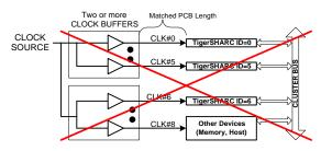
Figure 7. Not Recommended Clock Distribution
