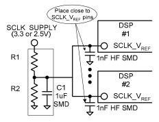
Figure 3. Recommended SCLK\_V<sub>REF</sub> Circuit
