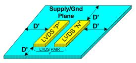
Figure 19. Supply Plane Overlap of LVDS Signal
