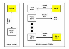
Figure 4. No Cluster Bus Connection Between TS20x Processors. (All Processor ID's Must Be 0)
