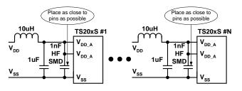
Figure 1. V<sub>DD\_A</sub> Supply Decoupling
