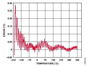
Figure 3. Error When Using Piecewise Linear Approximation Using 52 Calibration Points and Ideal Measurements
