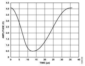
Figure 6. Example SENT Shaped Waveform Transmitter Output
