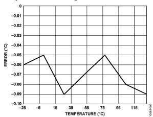
Figure 8. Error in °C of the RTD Measurement Using Piecewise Linearization Code and ADC0 Measurements
