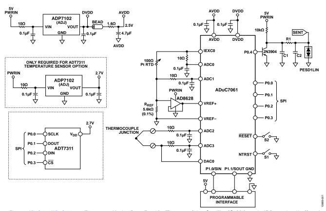
Figure~1.~A Du C7060/A Du C7061~as~a~Temperature~Monitor~Controller~with~a~Thermocouple~Interface~(Simplified~Schematic,~All~Connections~Not~Shown)
