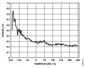
Figure 4. Error When Using Piecewise Linear Approximation Using 52 Calibration Points Measured by the ADC0 Pin of the ADUC7060/ADUC7061
