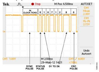
Figure 2. Example SENT Packet Measured at the P0.4 Pin
