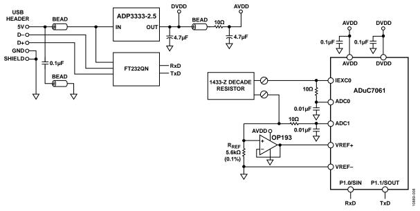
Figure 9. Test Setup Used to Calibrate and Test the RTD Output Voltage Range from −25°C to +114°C
