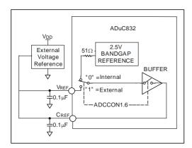
Using the internal refernce: On the ADuC812 to use the internal reference as a reference to external circuitry the Vref pin was used. This can be used to maintain compatibility with the ADuC812 however there is a gain error between this an the reference used for the ADC
