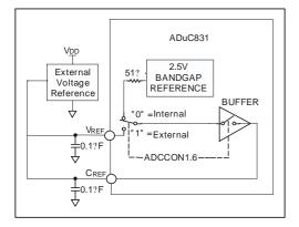
**Using the internal reference:** On the ADuC812 to use the internal reference as a reference to external circuitry the Vref pin was used. This can be used to maintain compatibility with the ADuC812 however there is a gain error between this an the reference used for the ADC conversions.
