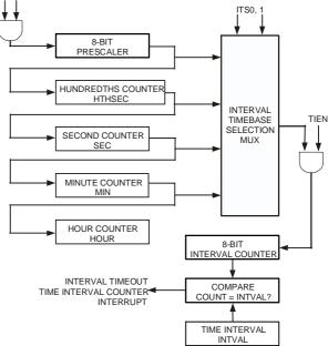
Figure 1. Block Diagram of the TIC structure
