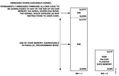
Figure 1. Parallel Programming Memory Map for Small Memory Devices
