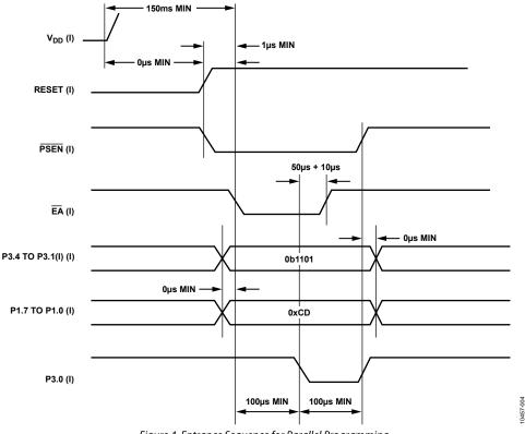
Figure 4. Entrance Sequence for Parallel Programming
