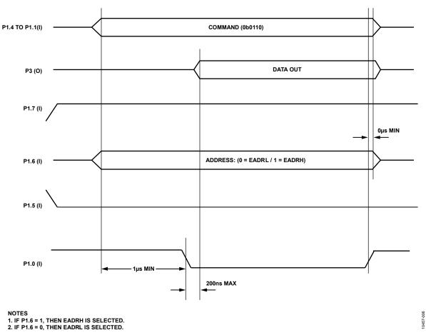
Figure 6. Read the Address Registers
