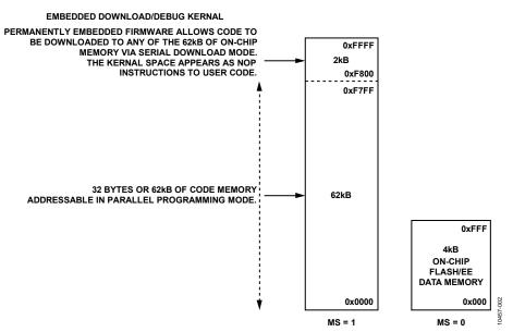
Figure 2. Parallel Programming Memory Map for Large Memory Devices
