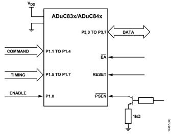
Figure 3. Pin Configuration for Parallel Programming
