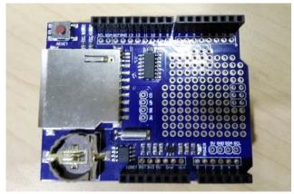
Figure 8. Data Logging Shield
