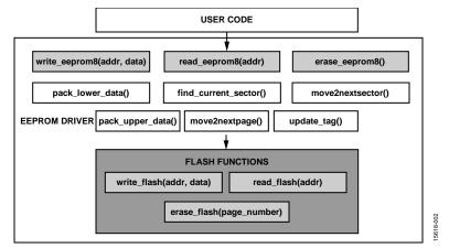
Figure 2. ADuCM3027/ADuCM3029 Flash EEPROM Emulation Software Structure
