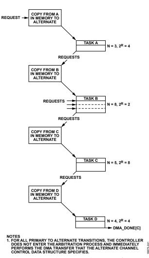
Figure 47. Peripheral Scatter Gather DMA Transfer
