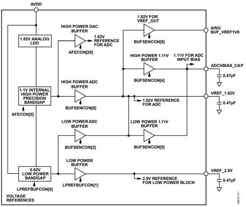
Figure 14. ADC Voltage Reference Options
