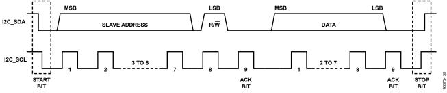
Figure 57. Typical I<sup>2</sup>C Transfer Sequence
