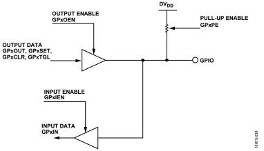
Figure 55. GPIO Structure for Pins with Pull-Up Resistors
