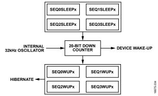
Figure 34. Sleep and Wake-Up Timer Block Diagram
