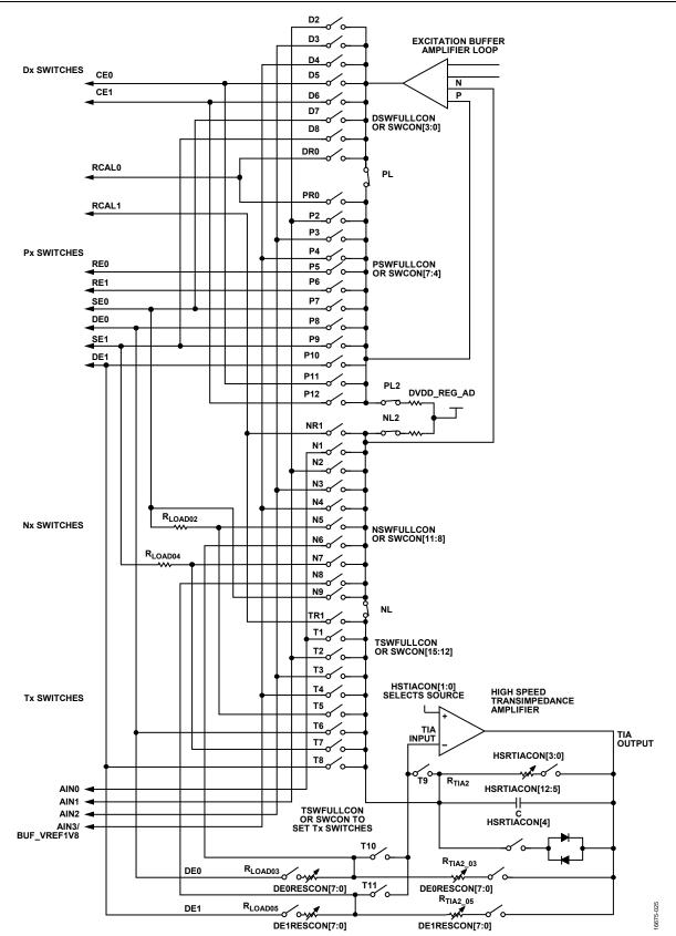
Figure 37. Recommended Switch Settings to Minimize Leakage in Hibernate Mode of Unused AFE Circuits
