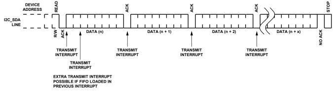
Figure 60. I<sup>2</sup>C Slave Transmit Interrupt Details
