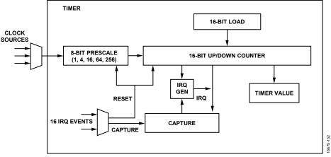
Figure 64. General-Purpose Timers Block Diagram
