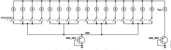
Figure 12. Temperature Sensor 1 Channel Overview
