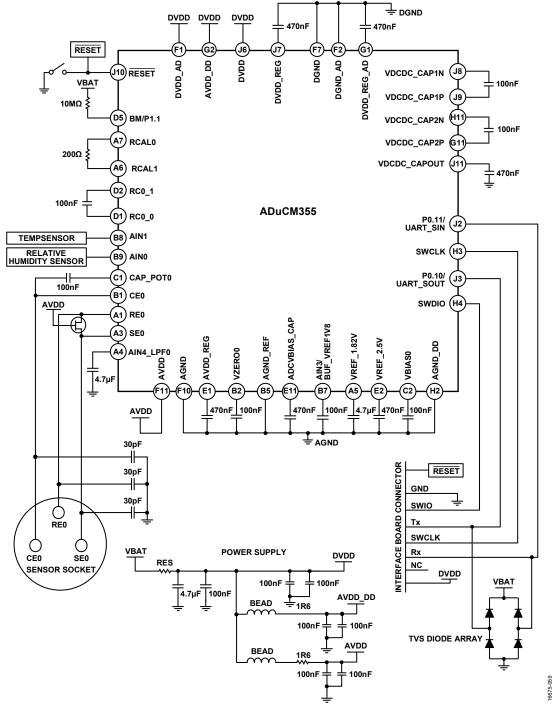
Figure 67. ADuCM355 Typical System Configuration
