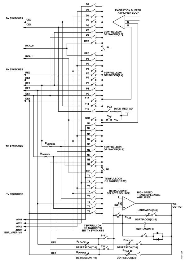
Figure 27. Switch Matrix Block Diagram, All Switches Connected to High Speed DAC Excitation Amplifier and Inverting Input of High Speed TIA
