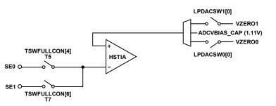
Figure 16. Low Power TIA, Low Power Potentiostat, and Low Power DAC Switches for Channel 0
