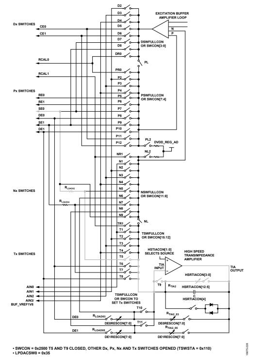
Figure 40. Signal Path for Low Power Potentiostat, Low Power TIA, and Switch Matrix to Perform Cyclic Voltammetry or Pulse Test on SE0 Node Using High Speed TIA
