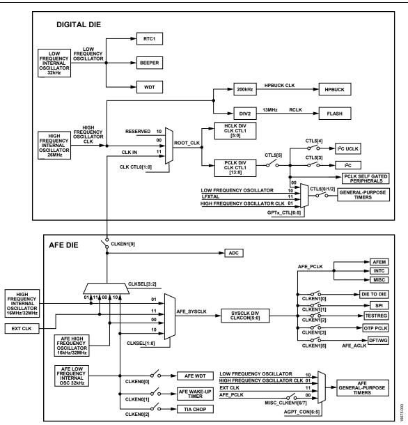
Figure 2. Clock Architecture Block Diagram
