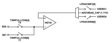
Figure 17. Low Power TIA, Low Power Potentiostat, and Low Power DAC Switches for Channel 1
