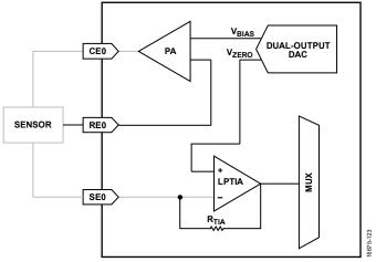
Figure 20. Electrochemical Standard Configuration
