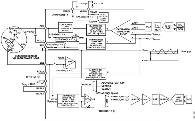
Figure 42. RLOADO2 Measurement
