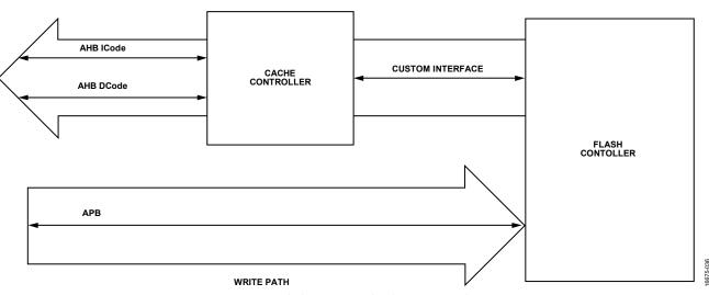
Figure 53. Flash Memory Read and Write Data Paths
