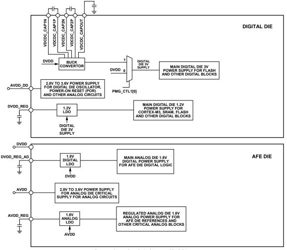
Figure 3. Power Supply Architecture Block Diagram
