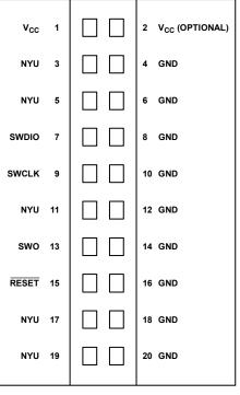
Figure 68. SWD 20-Pin Connector Pinout
