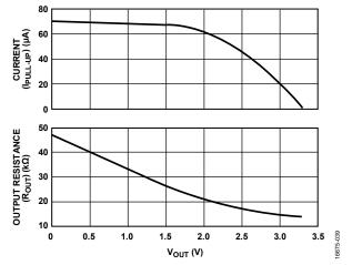
Figure 56. Typical Port 0, Port 1, and Port 2 Pull-Up Characteristics
