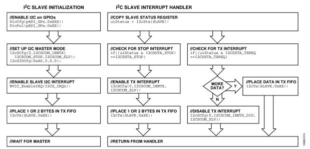
Figure 14. Slave Transmit Flowchart
