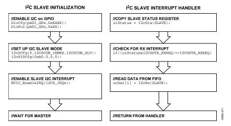
Figure 11. Slave Receive Flowchart
