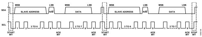
Figure 6. I<sup>2</sup>C Repeated Start Sequence
