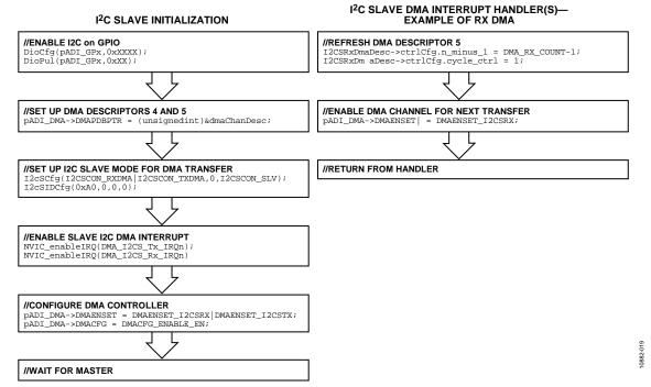
Figure 19. Slave DMA Transfer Flowchart
