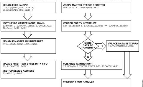
Figure 10. Master Transmit Flowchart
