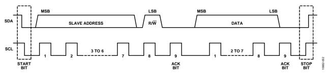
Figure 2. Typical I<sup>2</sup>C Transfer Sequence
