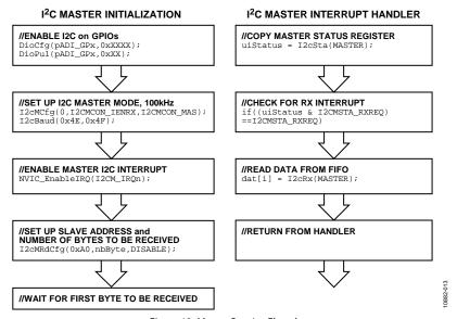
Figure 13. Master Receive Flowchart
