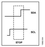
Figure 4. Stop Condition for I<sup>2</sup>C
