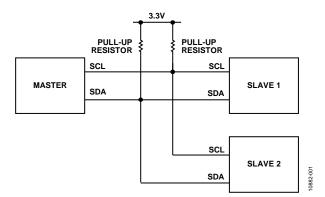
Figure 1. Single Master Multi-Slave I<sup>2</sup>C Block Diagram
