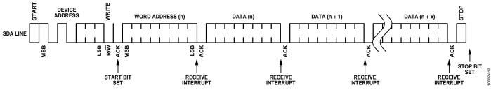
Figure 12. Example of a Slave Receive
