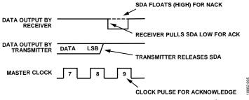
Figure 5. Acknowledge (ACK) and No Acknowledge (NACK) on the I<sup>2</sup>C Bus
