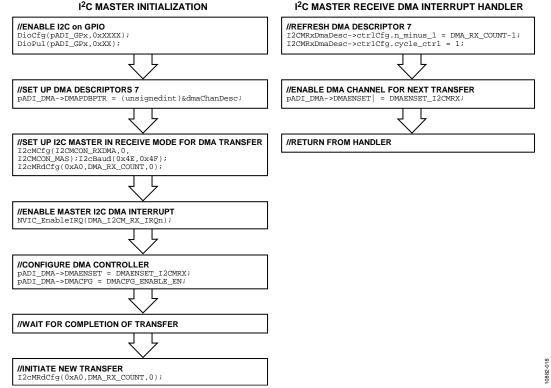
Figure 18. Master Receive DMA Transfer Flowchart
