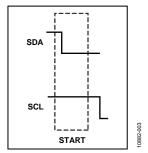
Figure 3. Start Condition for I<sup>2</sup>C
