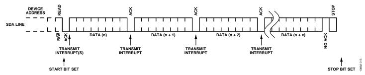
Figure 15. Example of a Slave Transmit
