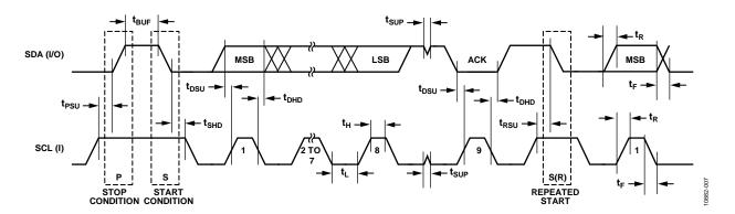
Figure 7. I<sup>2</sup>C Compatible Interface Timing
