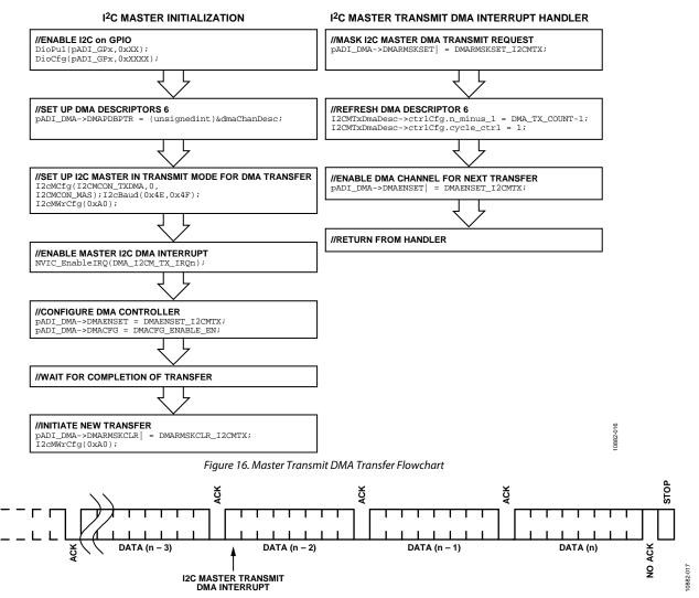
Figure 17. Master Transmit DMA Interrupt
