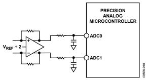
Figure 17. Buffering Differential Inputs
