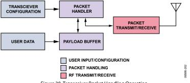
Figure 20. Transceiver Packet Handling Operation
