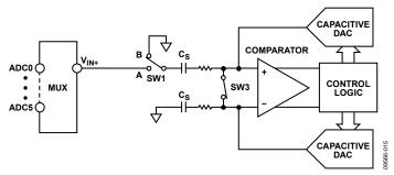
Figure 13. ADC in Single-Ended Mode
