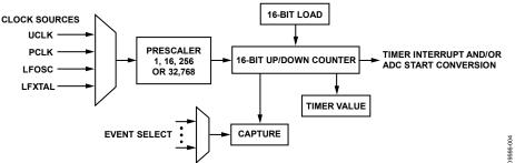
Figure 4. General-Purpose Timers Block Diagram
