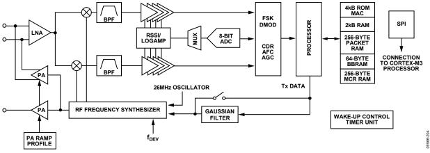
Figure 22. Functional Block Diagram
