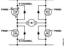
Figure 59. Example H-Bridge Configuration
