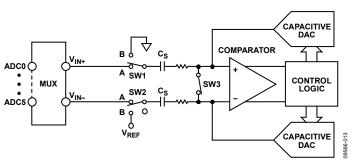
Figure 11. ADC Acquisition Phase
