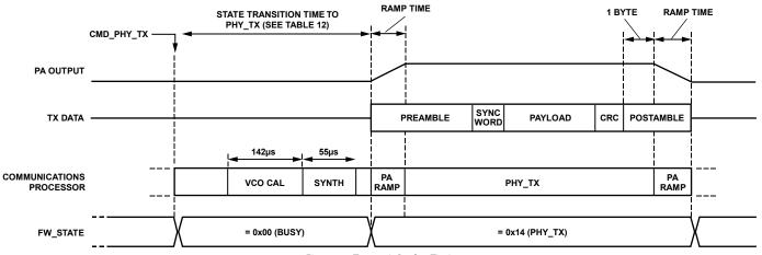
Figure 27. Transmit Packet Timing
