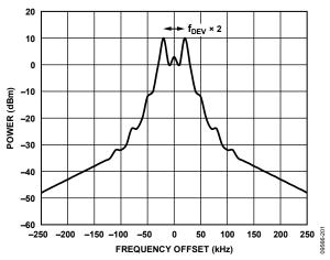
Figure 19. Idealized 2FSK Transmit Spectrum Example at 868 MHz. Data Rate = 38.4 kbps, Frequency Deviation (FDEV) = 20 kHz
