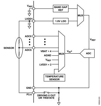
Figure 18. Ratiometric Measurement Typical Connection Diagram
