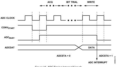
Figure 15. ADC Timing Internal Signals
