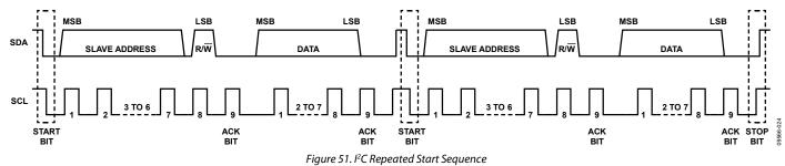
On the slave side, an interrupt is generated (if enabled in the I2CSCON register) when a repeated start and a slave address are received. This can be differentiated from receiving a start and slave address by using the status bits START and REPSTART in the I2CSSTA MMR.
