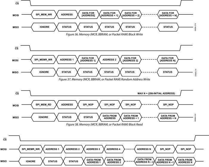
Figure 39. Memory (MCR, BBRAM, or Packet RAM) Random Address Read
