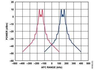
Figure 21. Maximum AFC Frequency Pull-In Range,  $\pm 150$  kHz, IF Bandwidth = 300 kHz
