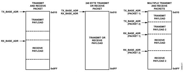
Figure 29. Example Packet RAM Configurations Using the Tx Packet and Rx Packet Address Pointers
