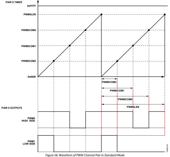
Note that the high-side PWM output for each channel must have a high duration period greater than or equal to the high period duration of the low-side output. For example, the high period for PWM0 must be equal to or, greater than the high period of PWM1.
