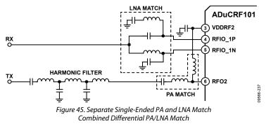
In this matching topology, the single-ended PA is not used. The differential PA and LNA match comprises a five-element discrete balun giving a single-ended input/output as illustrated in Figure 46. The harmonic filter is used to minimize the RF harmonics from the differential PA.
