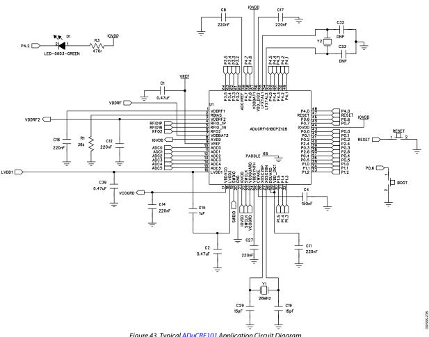
Figure 43. Typical ADuCRF101 Application Circuit Diagram 915 MHz Differential Mode Operation Example
