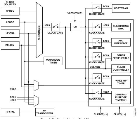
Figure 3. Clocking Architecture Block Diagram
