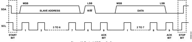
Figure 49. Typical I<sup>2</sup>C Transfer Sequence
