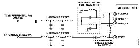
Figure 47. Matching Topology for Transmit Antenna Diversity
