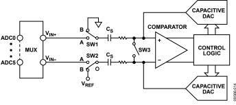
Figure 12. ADC Conversion Phase
