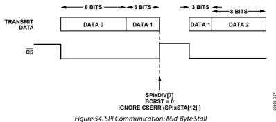
Note the SPI should only be reenabled when the  $\overline{CS}$  signal is high.
