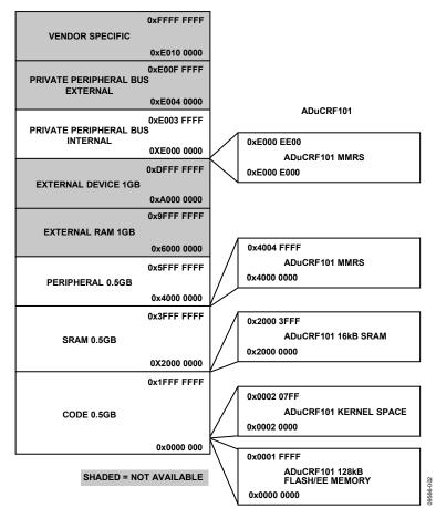
Figure 2. Cortex-M3 Memory Map Diagram
