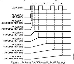
The PA ramps to the level set by the PA\_LEVEL or PA\_LEVEL\_MCR settings. Enabling the PA ramp reduces spectral splatter and helps meet radio regulations (for example, the ETSI EN 300 220 standard), which limit PA transient spurious emissions. To ensure optimum performance, an adequately long PA ramp rate is required based on the data rate and the PA output power setting. The PA\_RAMP setting should, therefore, be set such that
