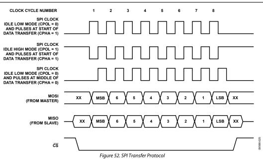
The SPIxCON register also control if the LSB or MSB is transfer first.
