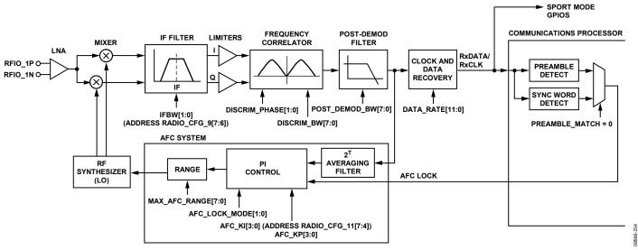
Figure 42. 2FSK/GFSK/MSK/GMSK Demodulation and AFC Architecture
