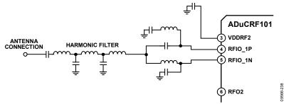
Figure 46. Combined Differential PA and LNA Match Transmit Antenna Diversity
