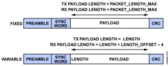
Figure 25. Payload Length in Fixed and Variable Length Packet Modes
