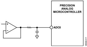
Figure 16. Buffering Single-Ended Input
