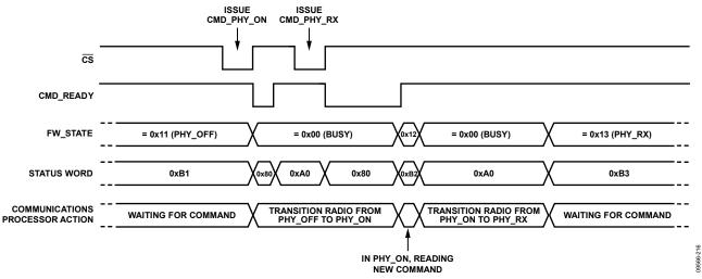
Figure 34. Command Queuing and Operation of the CMD\_READY and FW\_STATE Bits in Transitioning the RF Transceiver from the PHY\_OFF State to the PHY\_ON State and Then to the PHY\_RX State
