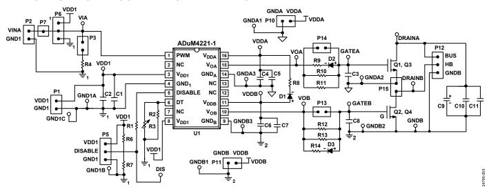
Figure 5. Schematic of the EVAL-ADuM4221-1EBZ
