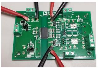
Figure 4. Power Supply Connections
