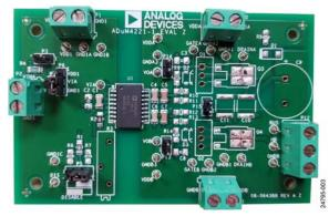
Figure 3. Example of P6 Configured to Connect Input to DC Values
