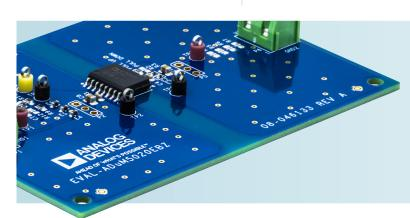
The ADuM5020 and ADuM5028 2-layer evaluation boards meet CISPR 22 Class B without stitching capacitance.
