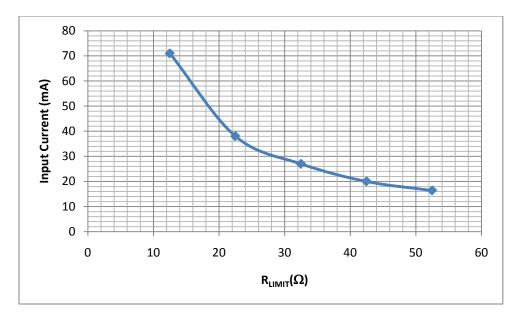
Figure 2. Average  $V_{DD}$  current for different limiting resistors.
