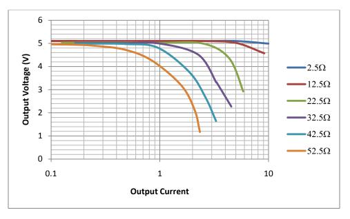
Figure 3. V<sub>ISO</sub> for different loads and limit resistors.
