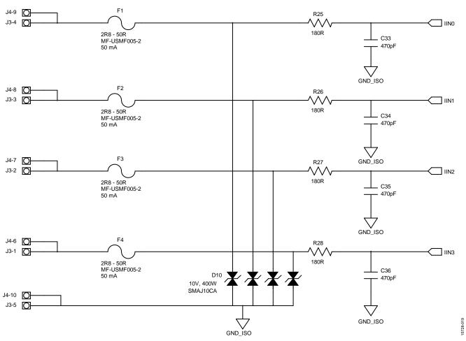
Figure 23. Current Input Front End Schematic
