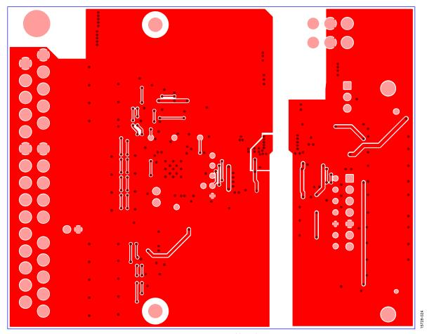
Figure 29. Layer 2, Solder Side
