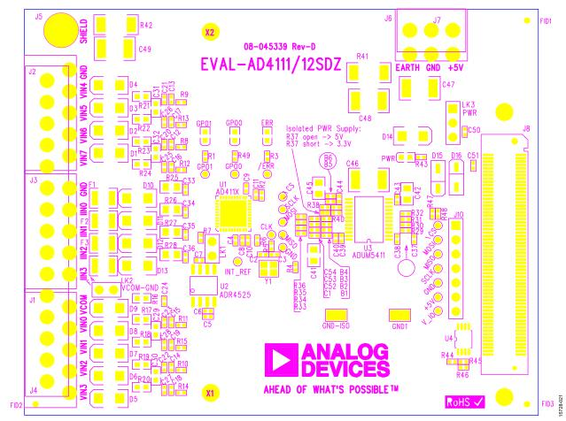
Figure 26. Printed Circuit Board (PCB), Top
