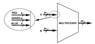
Figure 10. Multiplexed Color Inputs for the ADV7152
