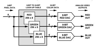
Figure 20. 8-Bit to 24-Bit Pseudo-Color Configuration
