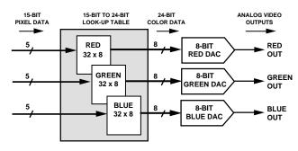
*Figure 22.* 15-Bit to 24-Bit True-Color Configuration This mode allows for the display of 15-bit True-Color Images.
