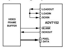
Figure 16. ADV7152 Interface Using SCKIN and SCKOUT
