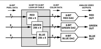
Figure 18. 24-Bit to 24-Bit Direct True-Color Configuration
