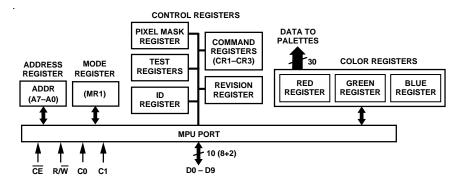
Figure 25. MPU Port and Register Configuration
