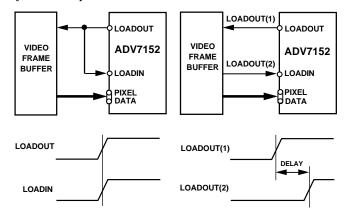
Figure 14. LOADOUT vs. Pixel Clock Input (CLOCK, CLOCK)
