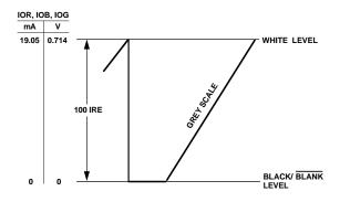
Figure 31. Composite Video Waveform (Pedestal = 0 IRE;  $R_{SET}$  = 259  $\Omega$ )
