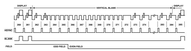
Figure 24. Timing Mode 3 (NTSC)
