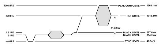
Figure 44. NTSC Composite Video Levels
