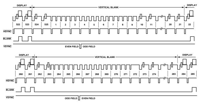
Figure 20. Timing Mode 2 (NTSC)
