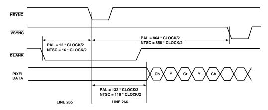
Figure 23. Timing Mode 2 Odd-to-Even Field Transition
