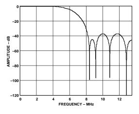
Figure 9. NTSC/PAL Extended Mode Filter
