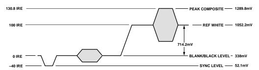
Figure 48. NTSC Composite Video Levels
