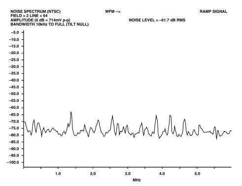
Figure 84. NTSC SNR Ramp Measurement
