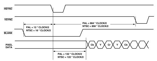
Figure 24. Timing Mode 2 Odd-to-Even Field Transition Master/Slave
