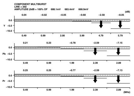
Figure 88. PAL YUV Multiburst Response
