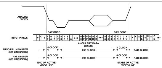
Figure 14. Timing Mode 0 (Slave Mode)
