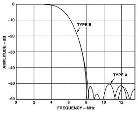
Figure 8. PAL Low-Pass Filter
