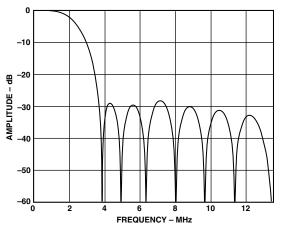
Figure 7. NTSC Notch Filter
