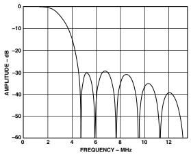
Figure 9. PAL Notch Filter
