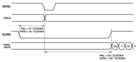
Figure 20. Timing Mode 1 Odd/Even Field Transitions Master/Slave
