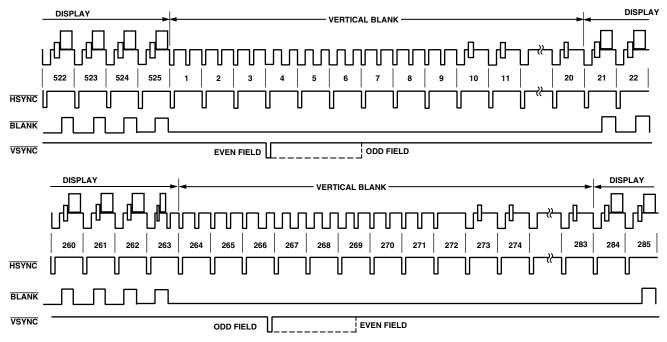
Figure 21. Timing Mode 2 (NTSC)
