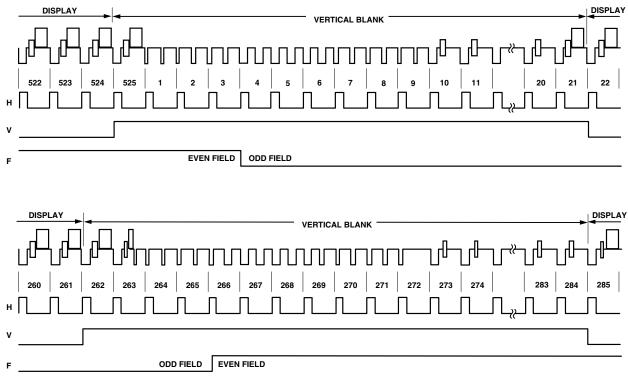
Figure 15. Timing Mode 0 (NTSC Master Mode)
