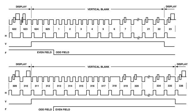
Figure 16. Timing Mode 0 (PAL Master Mode)
