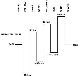
Figure 61. NTSC 100% Color Bars No Pedestal U Levels
