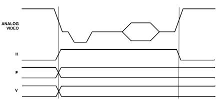
Figure 17. Timing Mode 0 Data Transitions (Master Mode)
