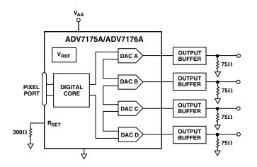
Figure 69. Output DAC Buffering Configuration
