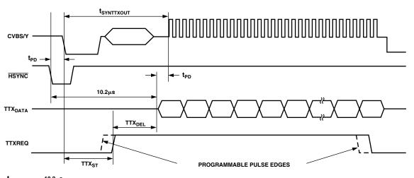
$t_{SYNTTXOUT} = 10.2 \mu s$  $t_{PD} = PIPELINE DELAY THROUGH ADV7175A/ADV7176A$ TTX<sub>DEL</sub> = TTXREQ TO TTX (PROGRAMMABLE RANGE = 4 BITS [0–15 CLOCK CYCLES])
