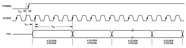
Figure 3. Teletext Timing Diagram
