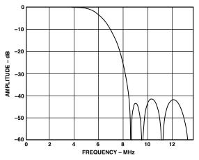
Figure 10. NTSC/PAL Extended Mode Filter
