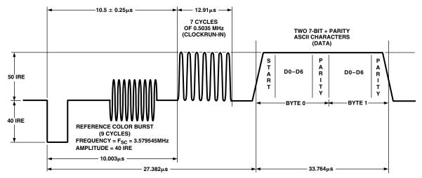
Figure 46. Closed Captioning Waveform (NTSC)
