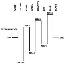
Figure 62. NTSC 100% Color Bars with Pedestal U Levels
