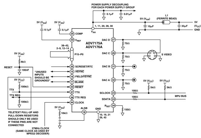
Figure 44. Recommended Analog Circuit Layout
