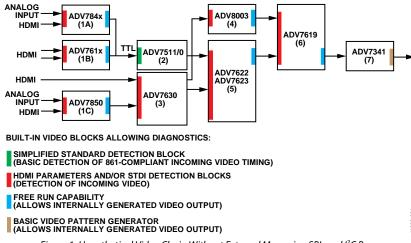
Figure 1. Hypothetical Video Chain Without External Memories, SPI, and I<sup>2</sup>C Buses
