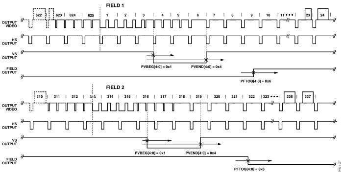
Figure 27. PAL Typical VSync/Field Positions Using Register Writes in Table 122
