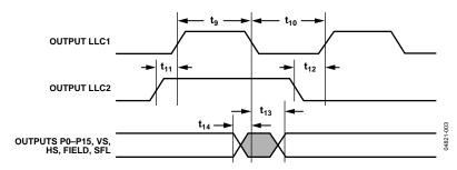
Figure 3. Pixel Port and Control Output Timing
