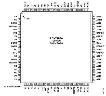
Figure 5. 80-Lead LQFP Pin Configuration
