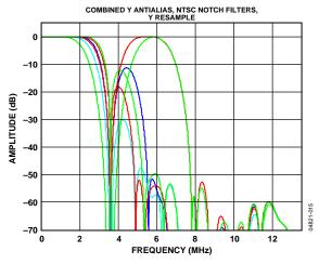
Figure 15. NTSC Notch Filter Responses
