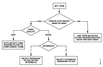
Figure 11. YSFM and WYSFM Control Flowchart
