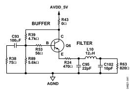
Figure 42. ADI Recommended Antialiasing Circuit for All Input Channels
