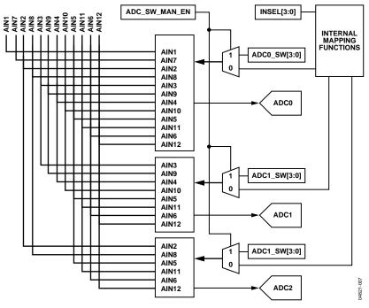
Figure 6. Internal Pin Connections
