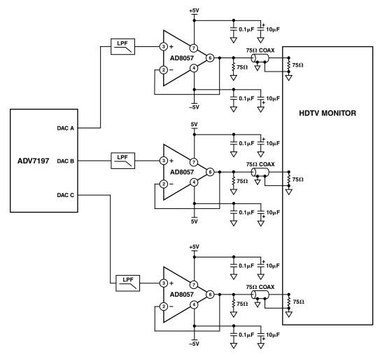
Figure 25. Output Buffer and Optional Filter
