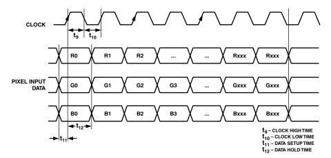
Figure 3. 4:4:4 RGB Input Data Format Timing Diagram
