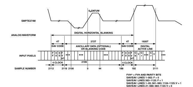
Figure 28. EAV/SAV Input Data Timing Diagram—SMPTE274M (1080i)
