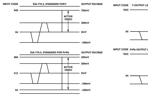
Figure 26. EIA 770.3 Standard Output Signals (1080i, 720p)
