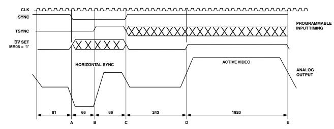
Figure 12. Async Timing Mode—Programming Input Control Signals for SMPTE295M Compatibility
