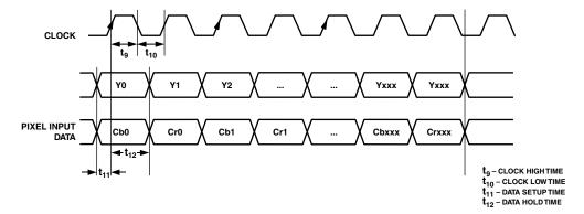
Figure 1. 4:2:2 Input Data Format Timing Diagram
