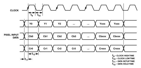
Figure 2. 4:4:4 YCrCb Input Data Format Timing Diagram
