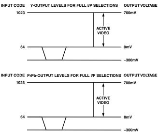
Figure 27. Output Levels for Full I/P Selection
