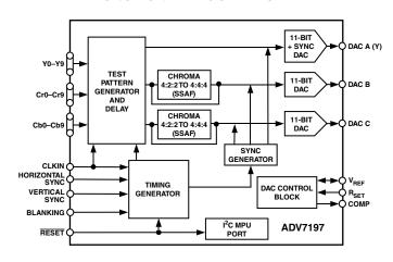
external horizontal, vertical, and blanking signals or EAV/SAV codes control the insertion of appropriate synchronization signals into the digital data stream and therefore the output signals.
