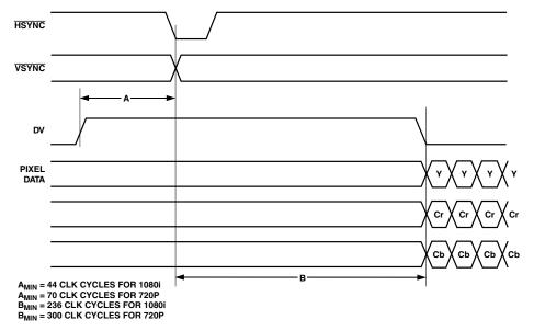
Figure 4. Input Timing Diagram
