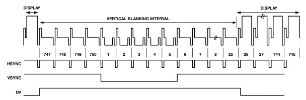
Figure 13. DV Input Control Signal in Relation to Video Output Signal for SMPTE296M (720p)
