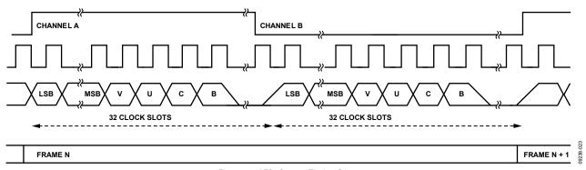
Figure 20. AES3 Stream Timing Diagram
