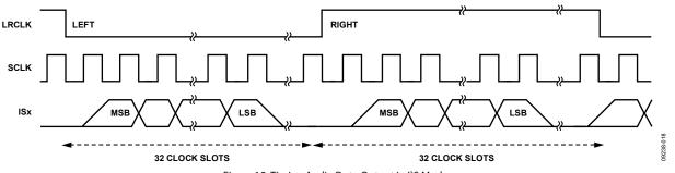
Figure 15. Timing Audio Data Output in I<sup>2</sup>S Mode
