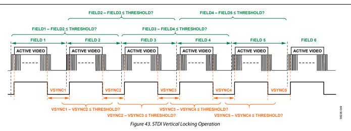
Once the STDI locks to the incoming video, the STDI registers the latest field length/VSync length as latched data (absolute field length: F, absolute VSync length: V). The STDI keeps monitoring and comparing FIELD/VSync lengths with the respective absolute length (F, V) once vertically locked. The STDI vertically unlocks if four consecutive FIELD or VSync lengths are greater than the respective threshold.
