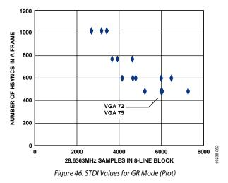
Note: Although the two points for VGA72 and VGA75 look very close, it is anticipated that the difference in the parameters is sufficient to distinguish between them.
