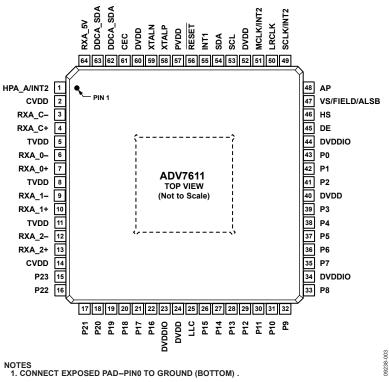
Figure 2. Pin Configuration
