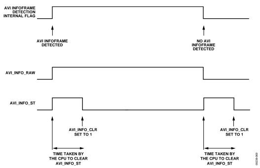
Figure 63. AVI\_INFO\_RAW and AVI\_INFO\_ST Timing
