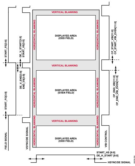
Figure 48. Synchronization Repositioning and Displayed Area
