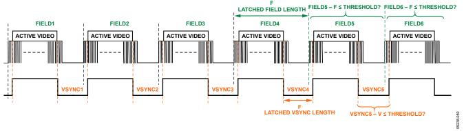
Figure 44. STDI VSync Monitoring Operation
