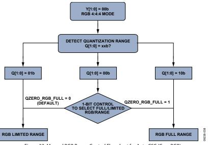
Figure 32. Manual RGB Range Control Flowchart for Auto CSC (Case RGB)
