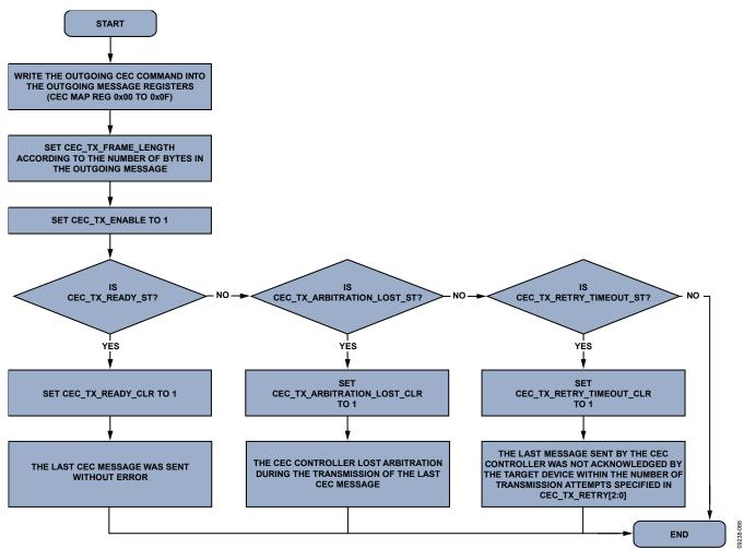
Figure 60. Using CEC Module as Initiator
