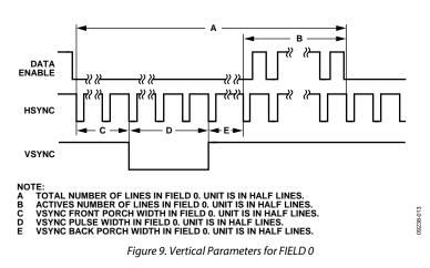
Note: Field 1 measurements should not be used for progressive video modes.
