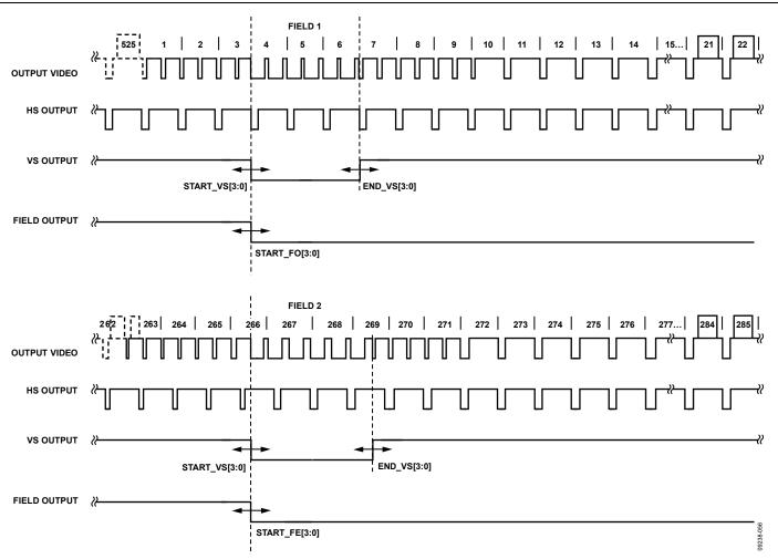
Figure 50. 525i VS Timing
