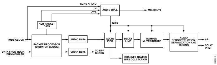
Figure 12. Audio Processor Block Diagram
