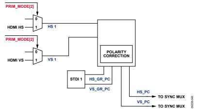
Figure 40. External/HDMI Syncs Routing to CP Section
