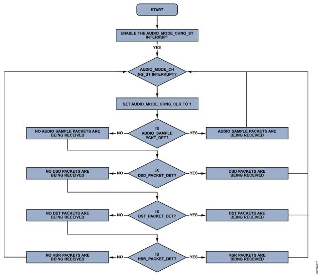
Figure 14. Monitoring Audio Packet Type Processed by ADV7611
