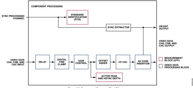
Figure 34. Component Processor Block Diagram
