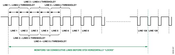
Figure 41. STDI Horizontal Locking Operation
