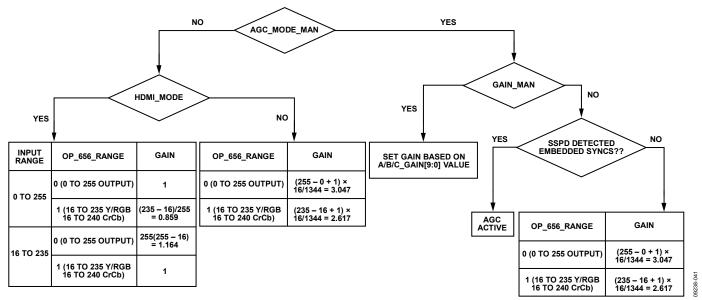
Figure 35. CP Automatic Gain Controls
