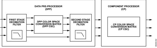
Figure 26. DPP/CP CSC Block Diagram
