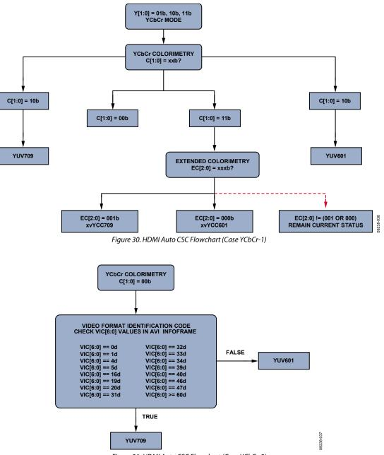
Figure 31. HDMI Auto CSC Flowchart (Case YCbCr-2)
