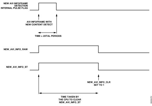
Figure 64. NEW\_AVI\_INFO\_RAW and NEW\_AVI\_INFO\_ST Timing
