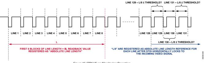
Figure 42. STDI HSync Monitoring Operation
