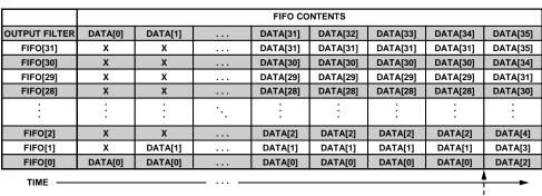
MULTIPLE-BYTE READ OF 2 SAMPLE SETS, DATA[0] AND DATA[1], CAUSES FIFO TO SHIFT.
