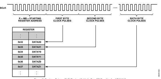
Figure 2. Register Pointer Shift During Multiple-Byte SPI Read in the ADXL345
