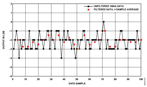
Figure 10. Noise Reduction with a Four-Sample Averaging Filter Utilizing FIFO
