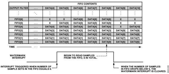
Figure 6. Example of FIFO Mode Operation Using Watermark Interrupt, Samples Value of 6
