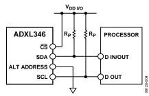
Figure 4. Recommended Connection for I<sup>2</sup>C Mode
