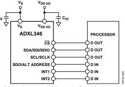
Figure 3. Recommended Connection for 4-Wire SPI Mode
