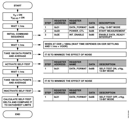
Figure 8. Self-Test Sequence
