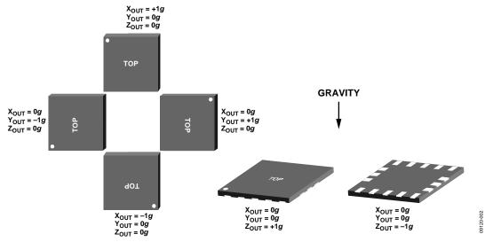
Figure 2. Output Response vs. Orientation to Gravity
